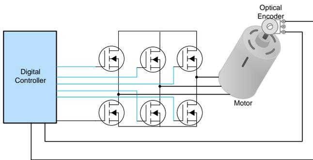
**Figure 3. Digital Control loop for motor**
