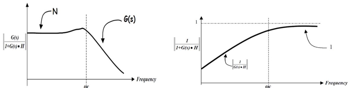
$$G_{NVCO}(s) = \frac{1}{1 + G(s) * H(s)} \quad \text{when } s \rightarrow 0, G_{NVCO}(s) \rightarrow 0; \text{ when } s \rightarrow \infty, G_{NVCO}(s) \rightarrow 1 \quad \text{High Pass For VCO PN}$$
