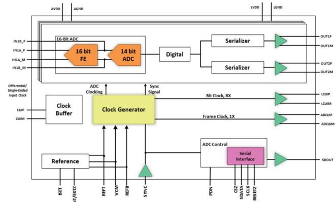
Figure 2. ADS5263 Functional Diagram
