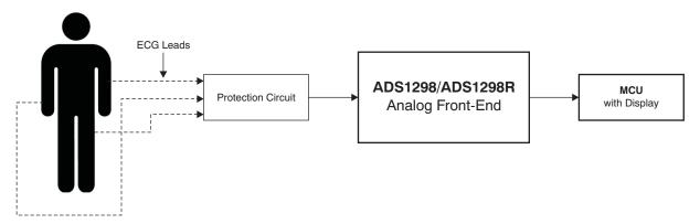
Figure 1. ECG Signal Path Based on ADS1298/98R
