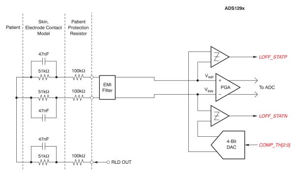
Figure 2. Analog Front-End Input Circuit
