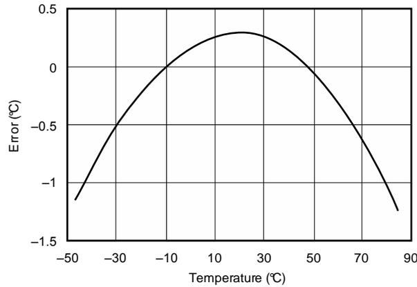
**Figure 5. Error vs Temperature, Single Measurement Technique**
