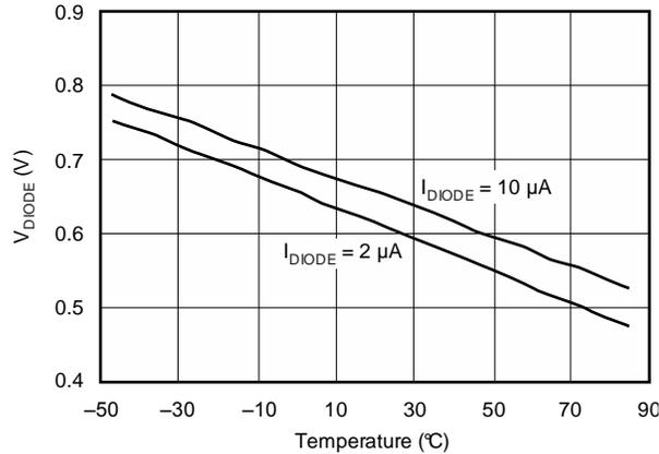
Figure 2.  $V_{\text{DIODE}}$  vs Temperature
