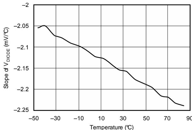
Figure 3. Slope of  $V_{\text{DIODE}}$  vs Temperature
