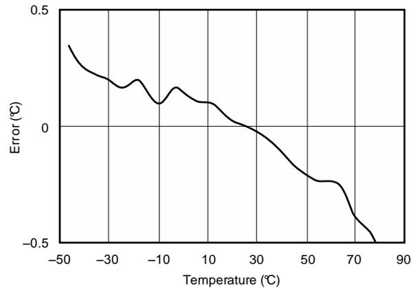
**Figure 6. Error vs Temperature, Differential Measurement Technique**
