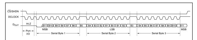
FIGURE 8. A Minor Software Change Corrects the Problem Illustrated in Figure 7.
