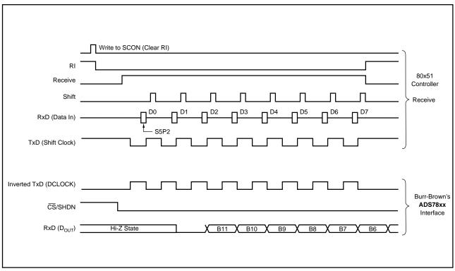
FIGURE 4. Timing Diagram for the ADS7816, ADS7817, or ADS7822 and a Generic 80x51 Microcontroller. This Timing Operation Requires that the TxD Output be Inverted with an External Gate.
