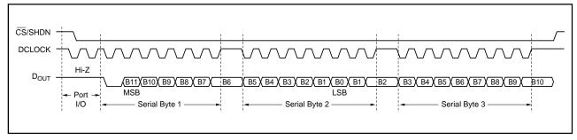
FIGURE 7. Since the 80x51 Type Controller Requires LSB First, the A/D Converter Must Output Its First 12 Bits (MSB First) and the 12 More Bits (LSB First). Notice that Bit 11 is Missing at the End of the Transfer.
