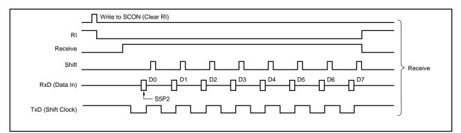
FIGURE 3. Serial Port Timing Diagram for the 80x51 Type Microcontroller.
