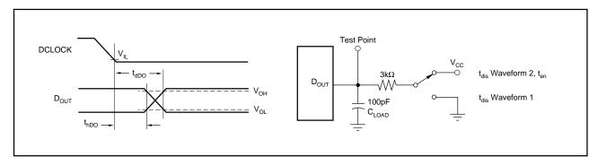
FIGURE 5. Set-up (t<sub>dDO</sub>) and Hold (t<sub>hDO</sub>) Times of the ADS1286, ADS7816, ADS7817 and ADS7822. See Table I for Timing Details.
