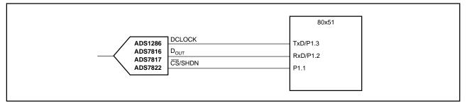
FIGURE 2. Circuit Diagram for the ADS7816, ADS7817, or ADS7822 and a Generic 80x51 Microcontroller.
