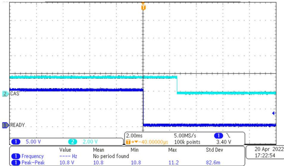
**Figure 4-19. Time-Domain Plot of Fault Detection Circuit Delay**
