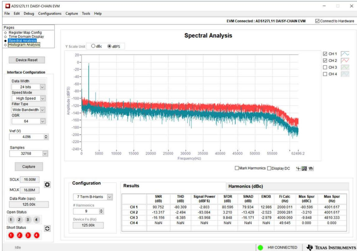
4-14. Frequency-Domain Plot of 20-V<sub>PP</sub> Input at Channel 1
