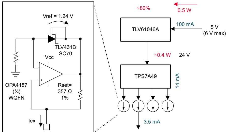
図 2-4. Current Source and Booster Stage
