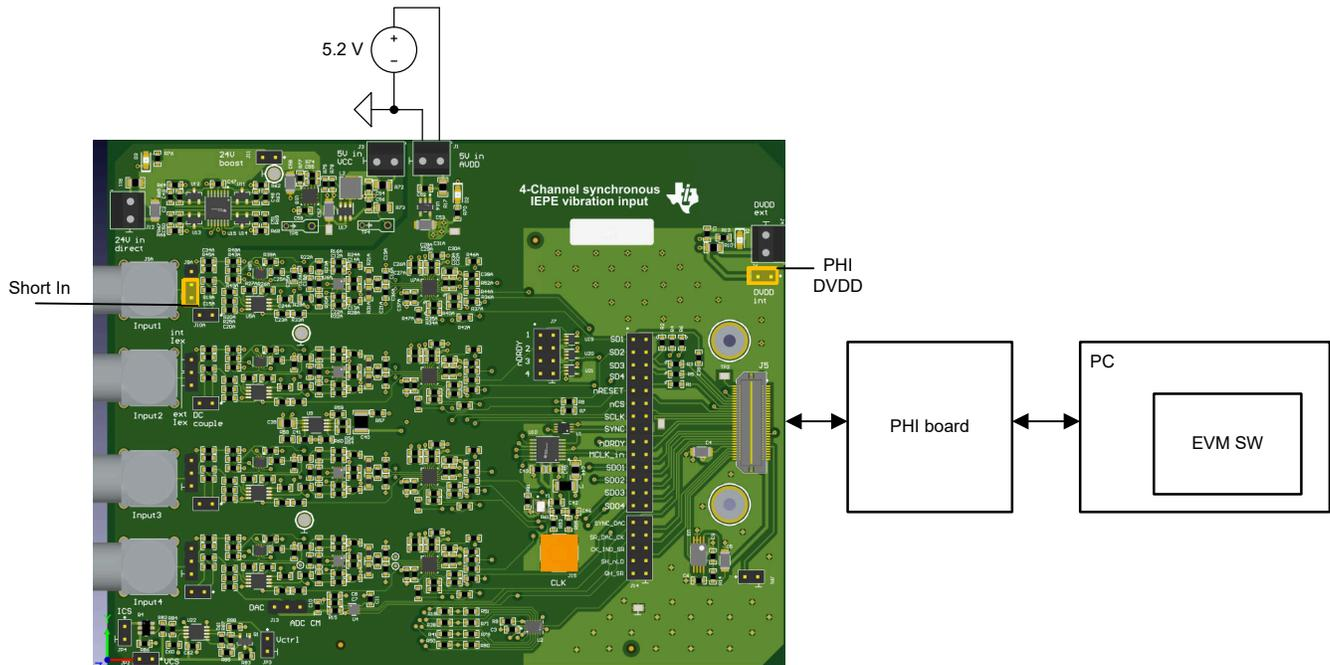
Figure 4-8. Basic Test Setup
