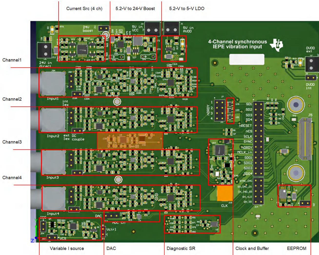
Figure 4-1. PCB Layout
