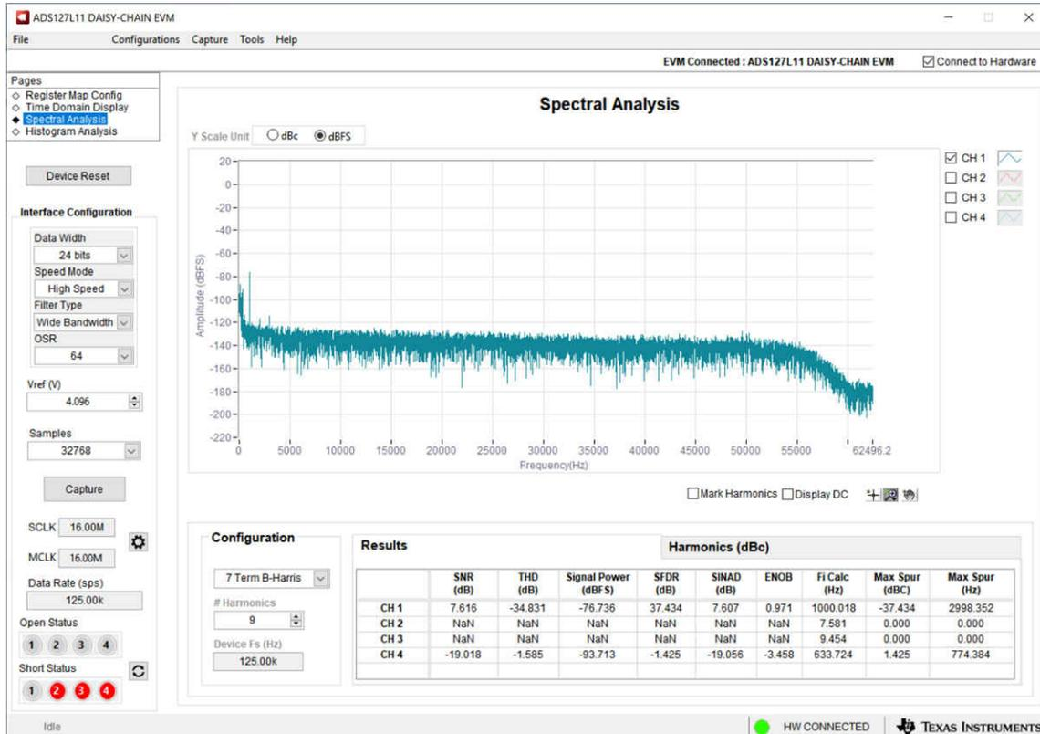
4-20. Frequency-Domain Plot of 1 kHz Applied to the IEPE Sensor
