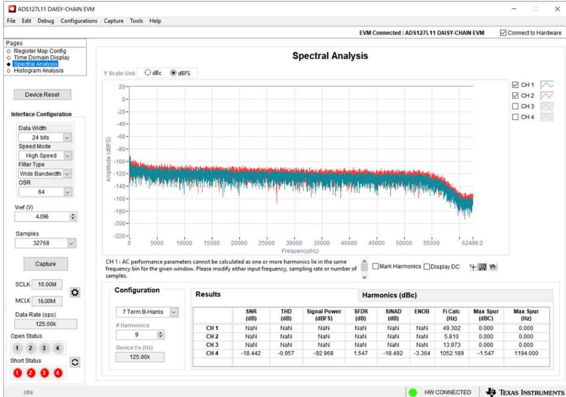
**Figure 4-16. Frequency-Domain Plot of 10-V<sub>PP</sub> Clock Image Input at Channel 1**
