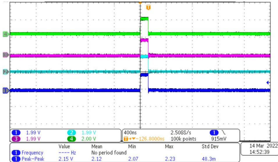
Figure 4-17. Time-Domain Plot of Data Ready Signal
