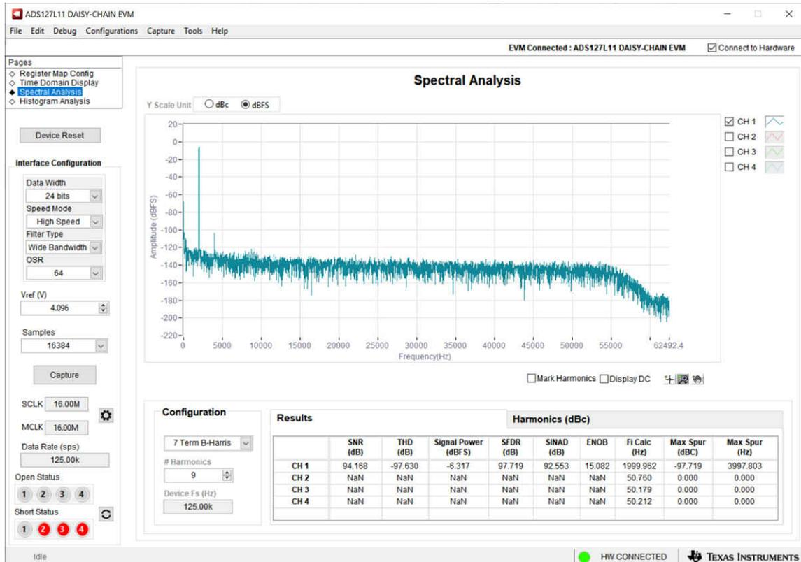
**Figure 4-15. Frequency-Domain Plot of 2-kHz, 10-V<sub>PP</sub> Input at Channel 1**
