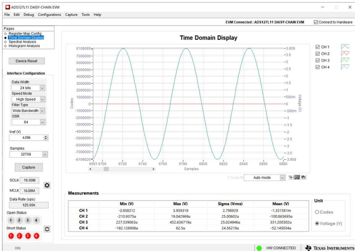
4-13. Time-Domain Plot of 20-V<sub>PP</sub> Input at Channel 1
