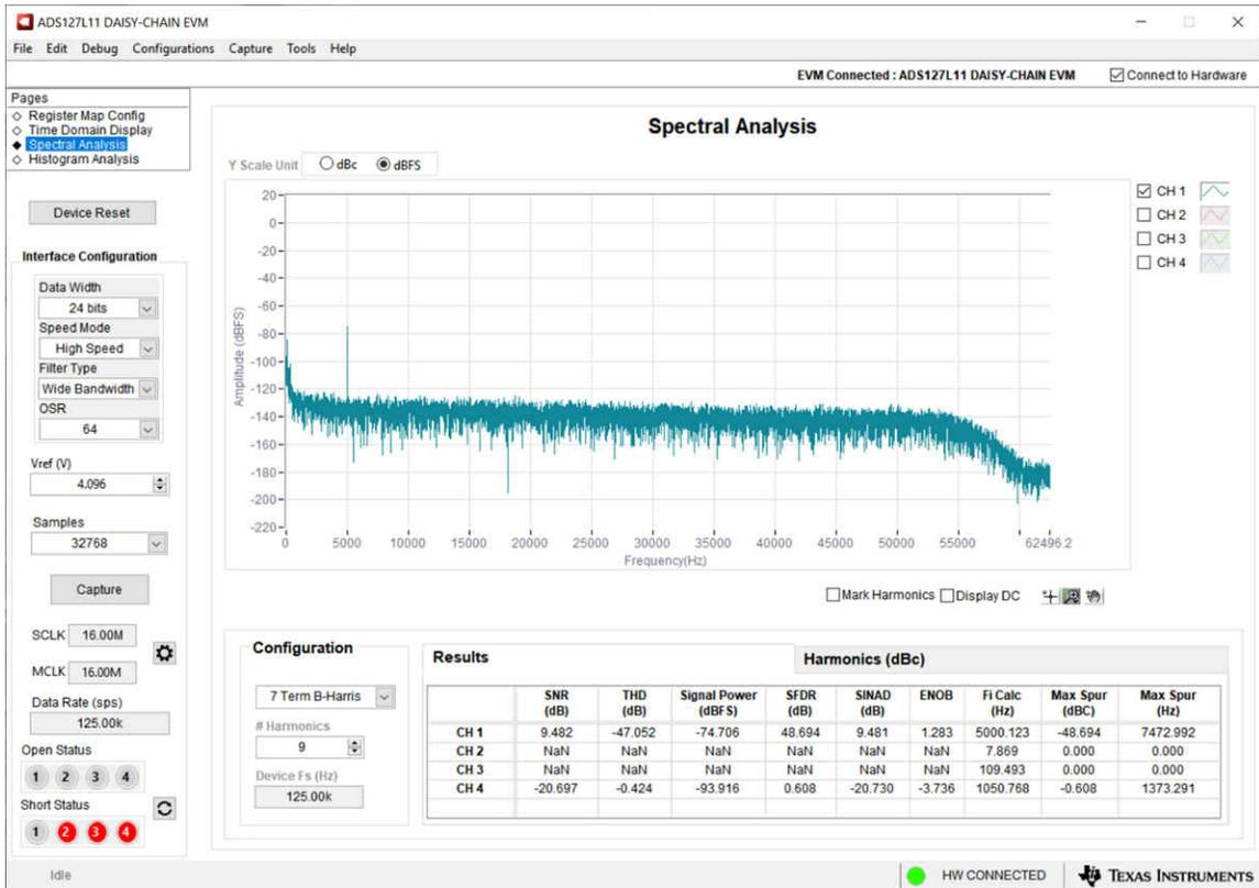
図 4-21. Frequency-Domain Plot of 5 kHz Applied to the IEPE Sensor
