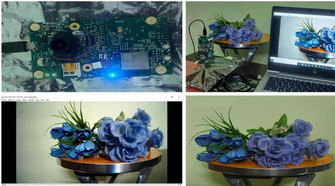
☒ 3-22. Video Streaming- Camera Module (Top Left), Camera Video Streaming Subject (Top Right), Camera Video Streaming on VLC (Bottom Left), Subject (Bottom Right)
