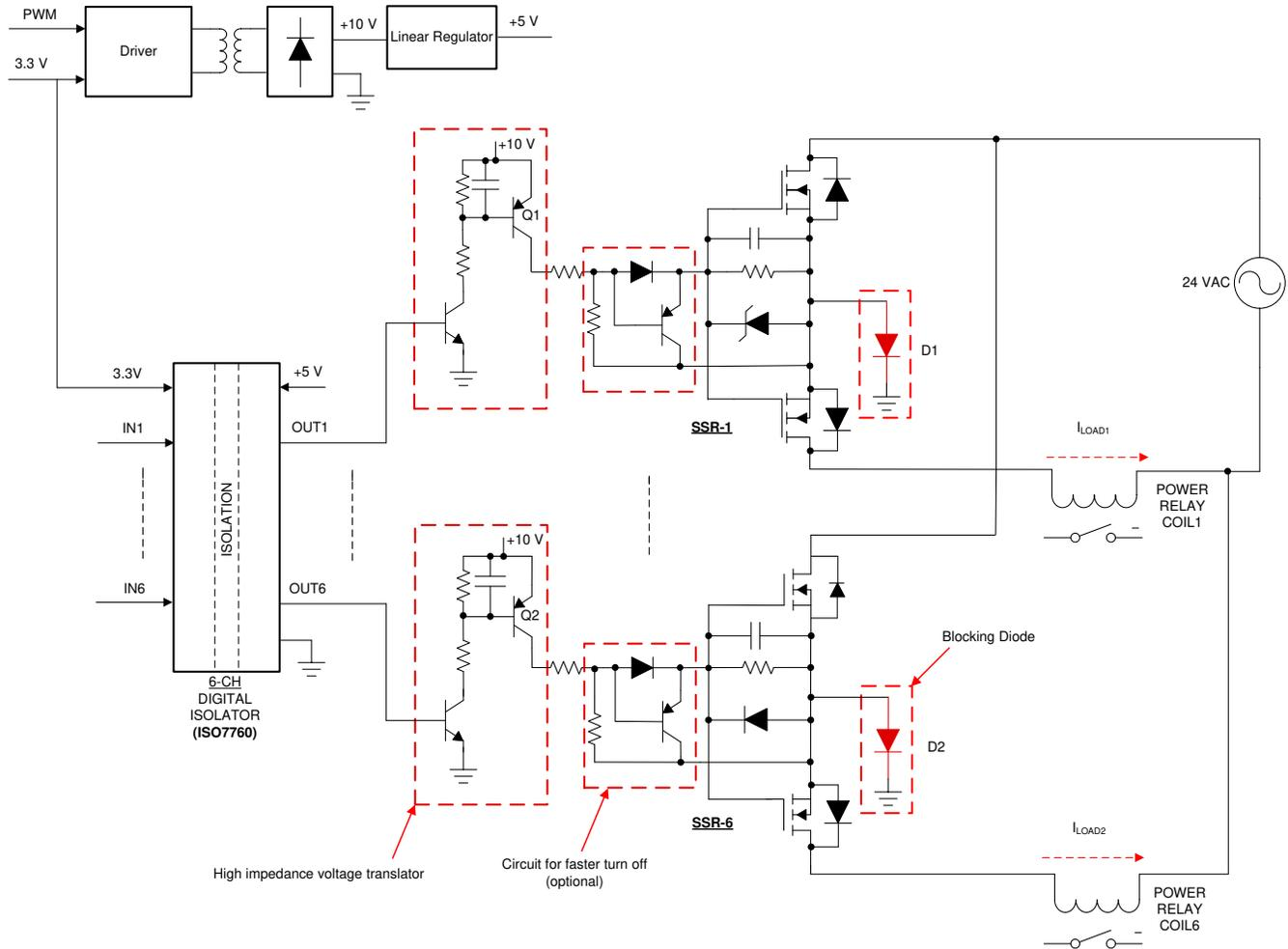
図 2-6. Circuit Topology to Drive Multiple SSR With Single Isolating Element
