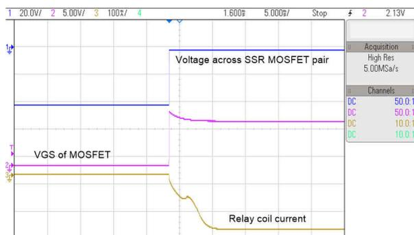
図 3-8. SSR Turn on Waveform at -40 V
