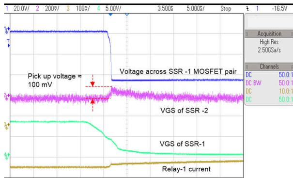
3-14. Test Waveforms Showing Least Cross-Coupling During SSR Turn Off
