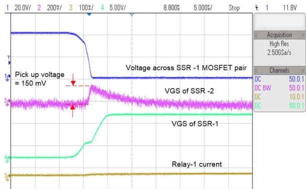
3-15. Test Waveforms Showing Least Cross-Coupling During SSR Turn On
