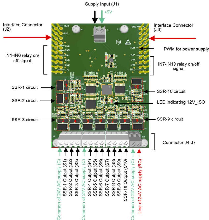
図 3-1. Input and Output Connectors in the Reference Design Board
