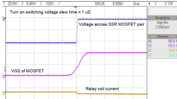
図 3-10. MOSFET Turn on Switching Waveform
