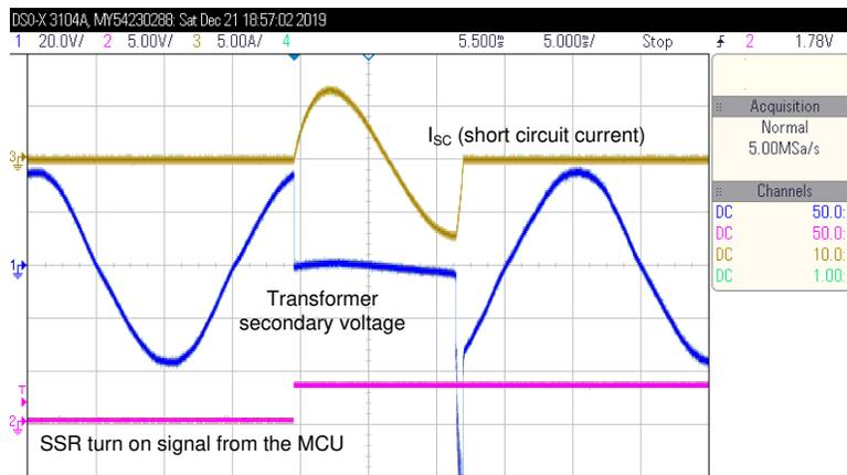
**3-18. Short-Circuit Test Waveforms With External Fuse**
