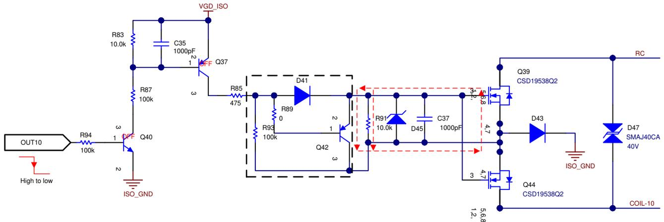
**図 2-10. Gate Driver Circuit for the SSR MOSFETs and the Turn off Gate Current Path**
