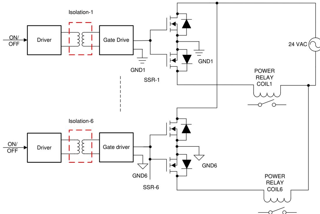
図 2-3. Multichannel SSR Topology With Independent Isolation Between SSR Channels
