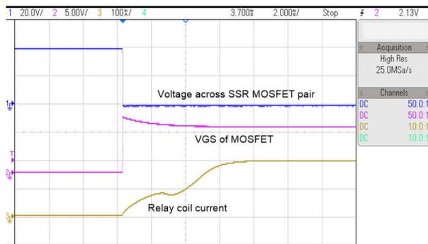
図 3-6. SSR Turn on Waveform at 40 V
