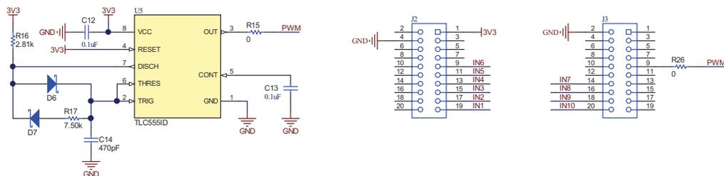
**Figure 2-13. TIMER to Generate PWM Signal and Interface Connector**
