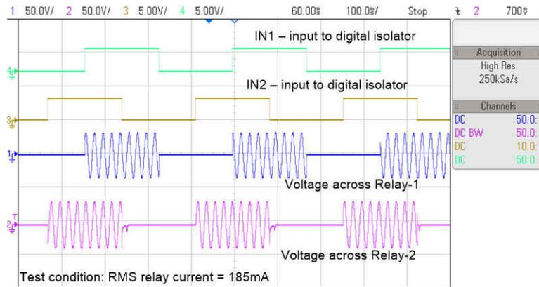
3-16. Test Waveforms at 24-VAC Supply - Independent Operation of SSR
