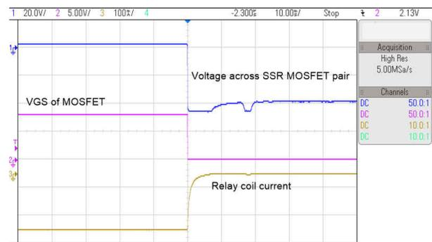
図 3-9. SSR Turn off Waveform at -40 V
