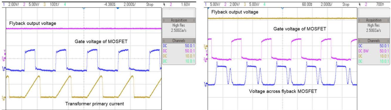
図 3-5. Flyback Circuit Voltage and Current Waveforms - All SSR Off
