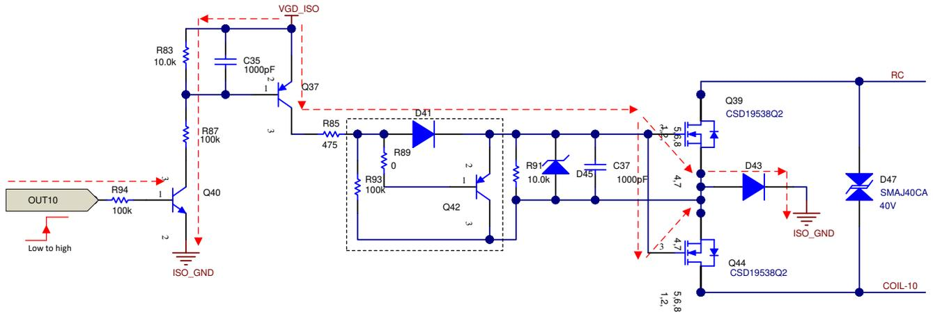
図 2-9. Gate Driver Circuit for the SSR MOSFETs and the Turn on Gate Current Path
