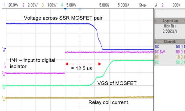
図 3-12. Waveforms Showing SSR Turn on Time
