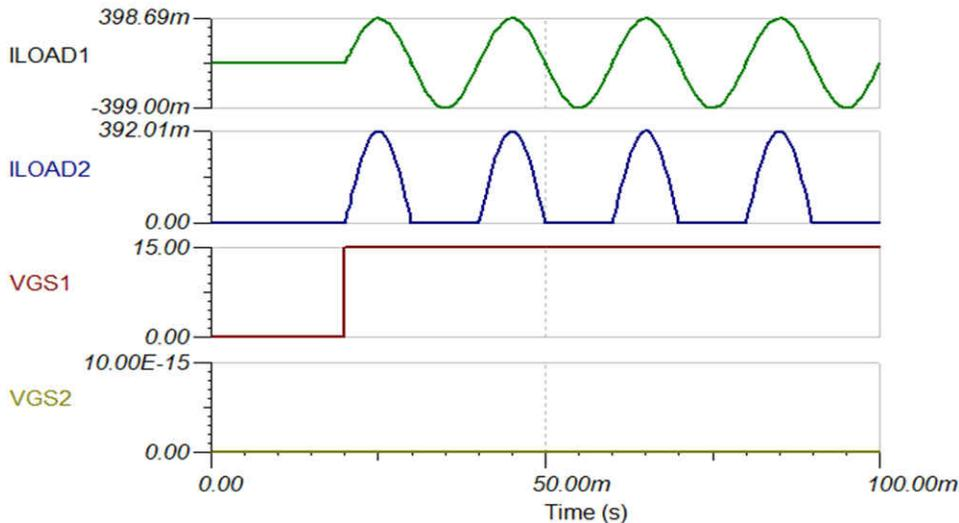
Figure 2-5. Half-Wave Rectified Current in Driving Multiple SSR With Common Ground Gate-Drive Supply
