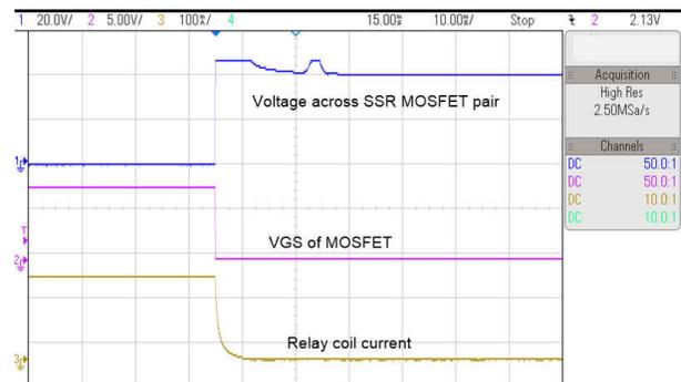
図 3-7. SSR Turn off Waveform at 40 V
