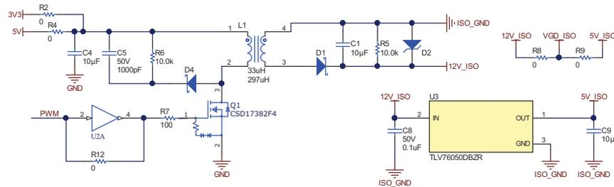
**Figure 2-12. Open-Loop Flyback Power Supply**
