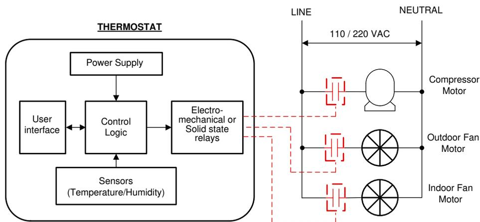
図 2-1. Multiple Relays Controlling Different Loads in Thermostats
