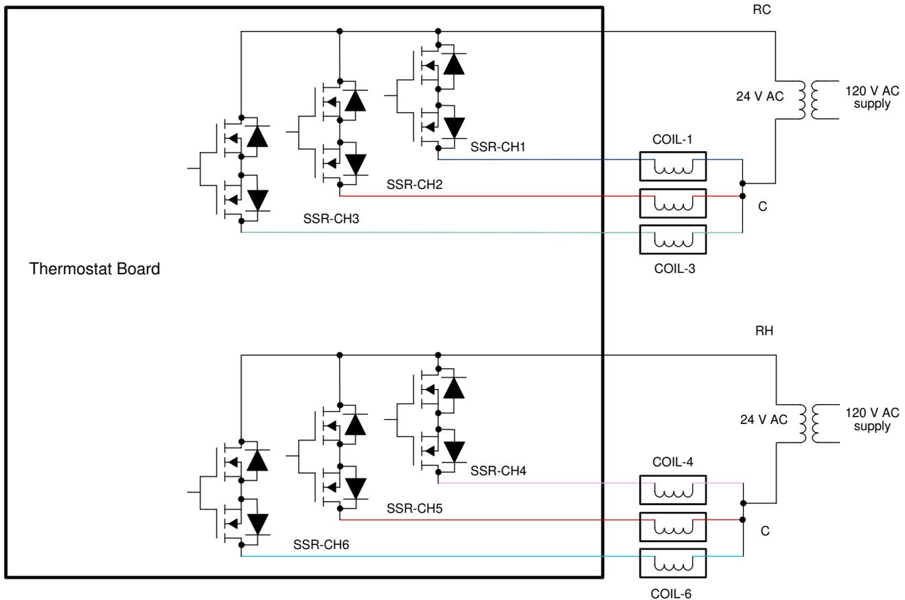
Figure 3-19. Circuit Topology in Driving Multiple SSRs With two AC Transformers
