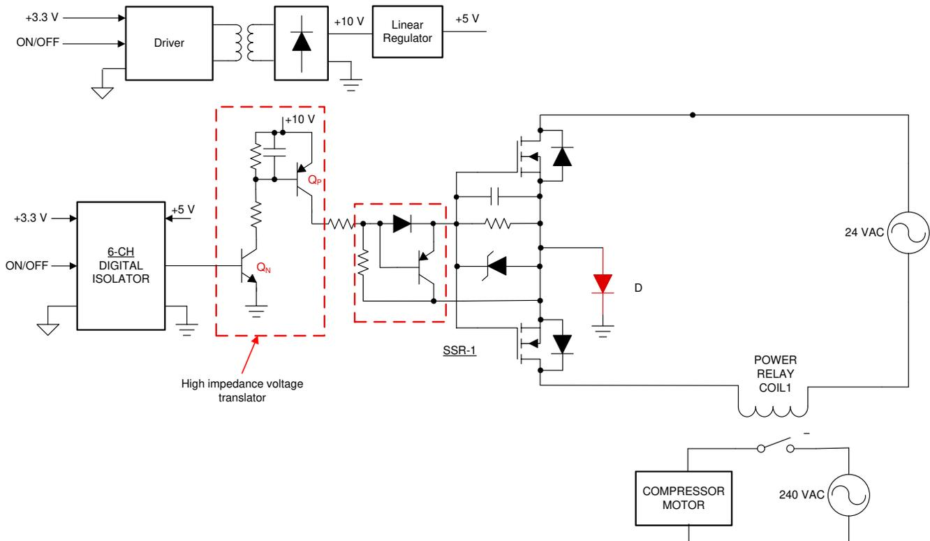
**Figure 2-7. High Impedance Voltage Translator for Driving Multiple SSR With Single Isolating Element**
