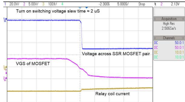
図 3-11. MOSFET Turn off Switching Waveform
