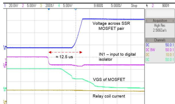
図 3-13. Waveforms Showing SSR Turn off Time
