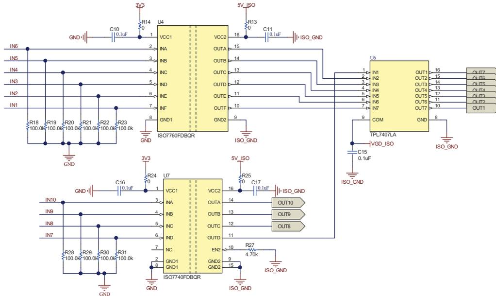
図 2-11. Digital Isolator Interface for Ten Channel SSR
