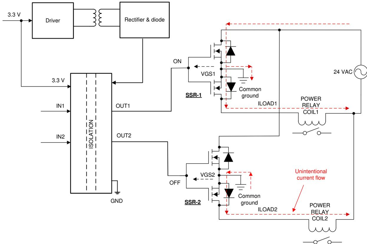
Figure 2-4. Unintentional Current Flow in Driving Multiple SSR With Common Ground Gate-Drive Supply
