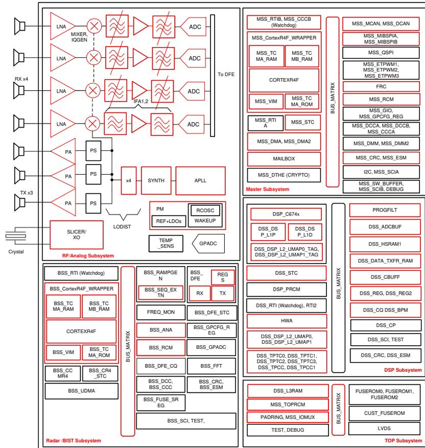
Figure 2-2. mmWave Safety Components
