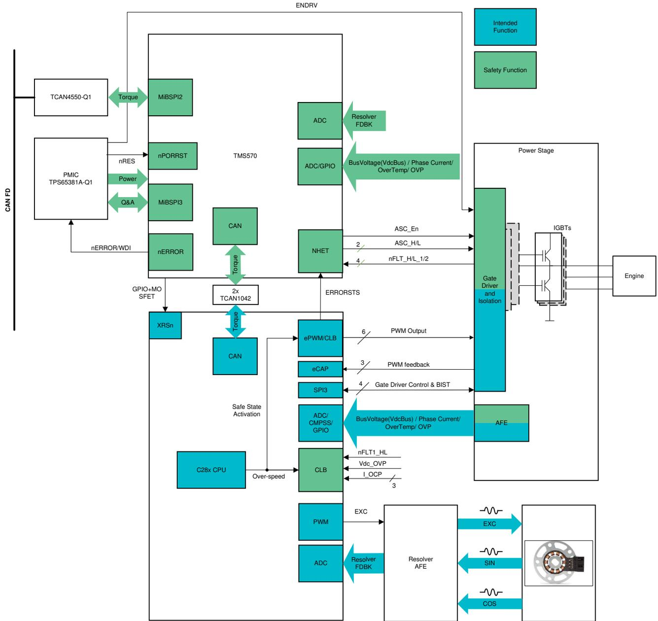
図 3-19. EV Traction Inverter System Block Diagram
