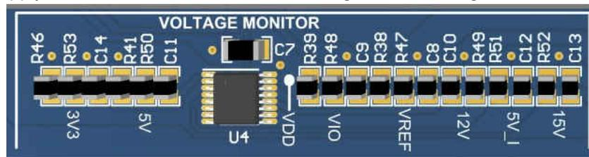
**Fig 3-8. External Power Monitoring by Safety MCU**
