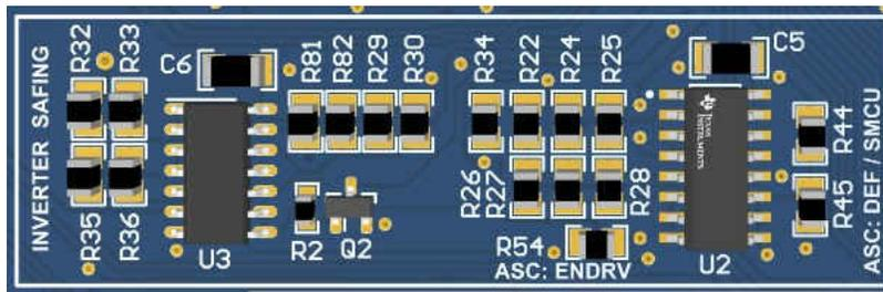
Figure 3-3. ASC Logic Selection between Safety MCU and Default Setting
