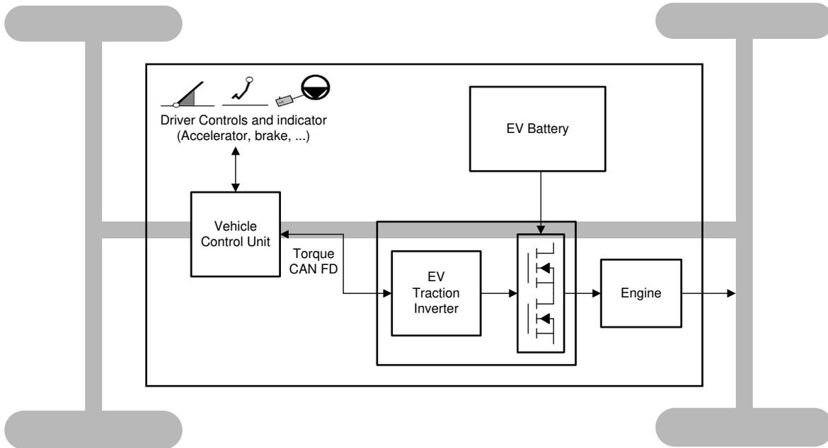
図 1-2. Electric Vehicle Traction System
