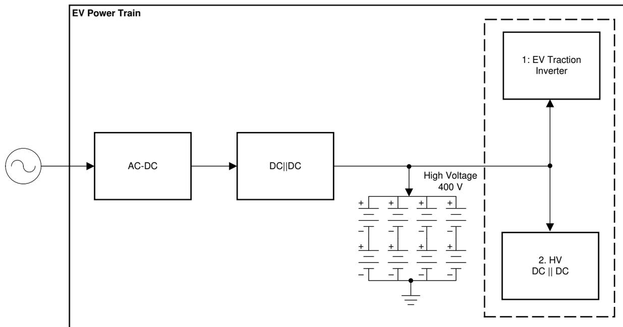
**Fig 1-1. Electric Vehicle Power-Train System**
