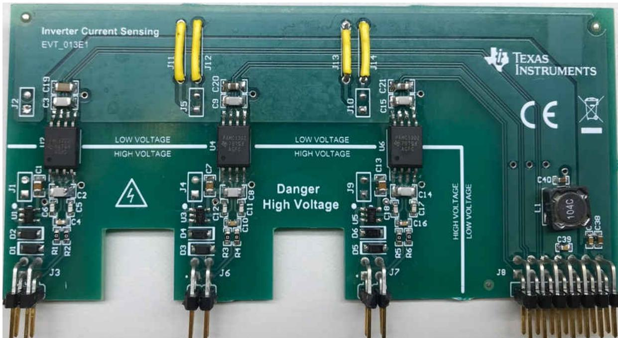
図 3-24. Inverter Current Sense Board
