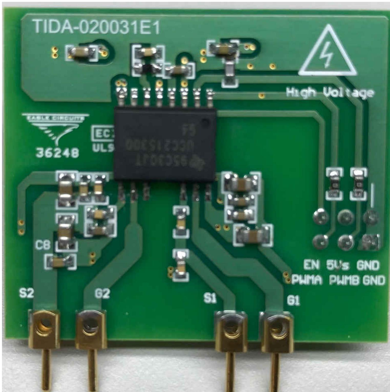
図 3-28. DC-DC Isolated Gate Driver
