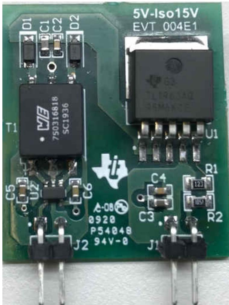
図 3-14. 5-V to 15-V/0.5-A power supply module
