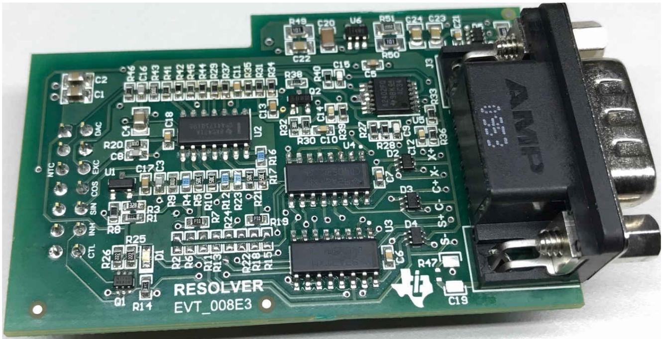
図 3-18. Resolver Analog Front End Module
