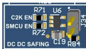
Figure 3-5. MCU Selection for DC-DC Safing
