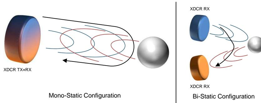
図 5. Sonar Configurations
