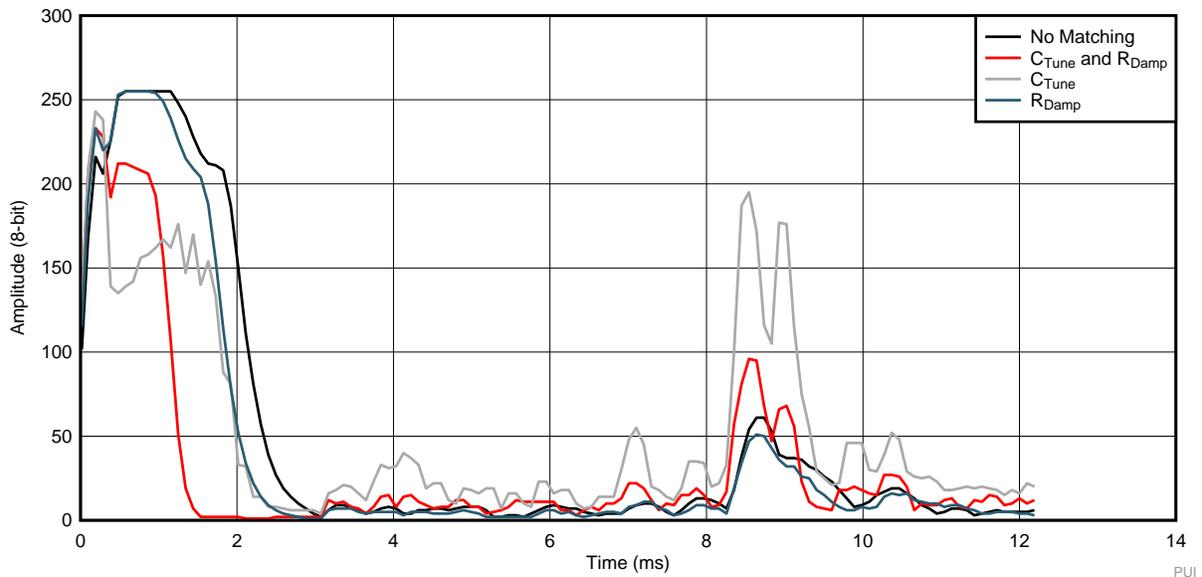
図 16. PUI Audio Short Range Matching Options With Reference Object at 1.4 m
