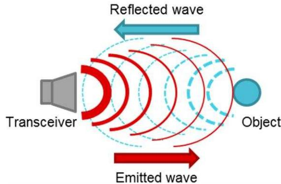
図 1. Ultrasonic Time-of-Flight Measurement
