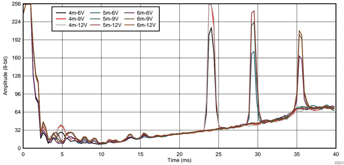
図 19. Murata Long Range Echo Data Dump Performance (100 Samples Averaged) at 4, 5, and 6 m With Voltages of 6, 9, and 12 V
