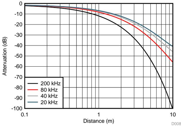
4 shows the attenuation of sound pressure by distance and frequency.
