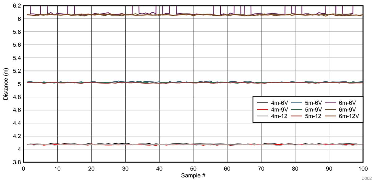
図 20. Murata Long Range Measurement Results (100 Samples Averaged) at 4, 5, and 6 m With Voltages of 6, 9, and 12 V
