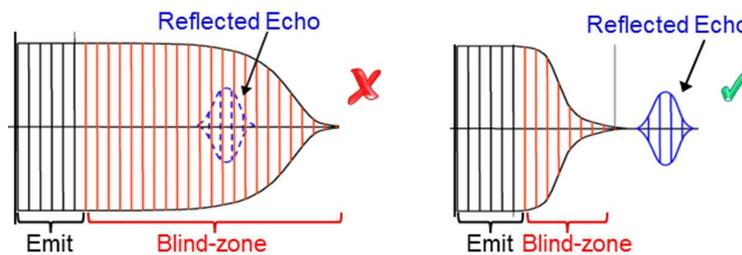
図 6. Monostatic Ring Decay Limiting Short Range Detection
