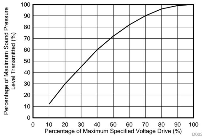
図 7. Voltage Driver vs Sound Pressure Level
