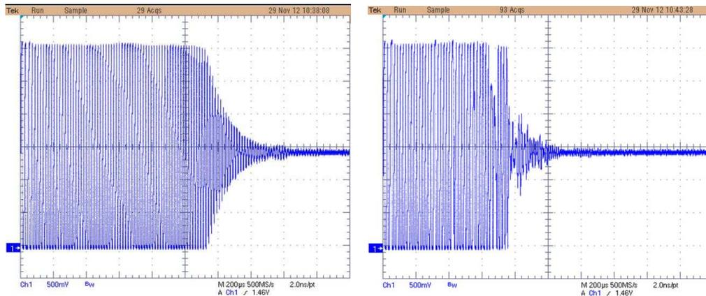
図 9. Ringing-Decay Time Before and After Tuning of Variable Coil Transformer
