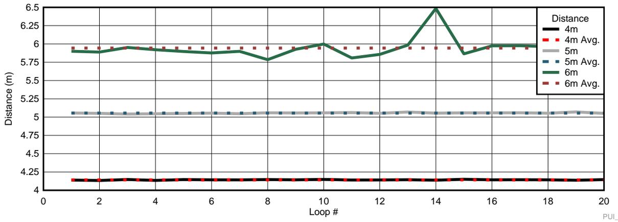
図 15. PUI Audio Long Range Measurement Results at 4, 5, and 6 m
