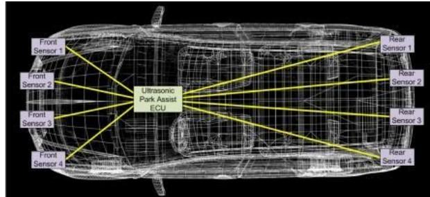
図 2. Ultrasonic Parking Assist Sensor in a Point-to-Point Configuration
