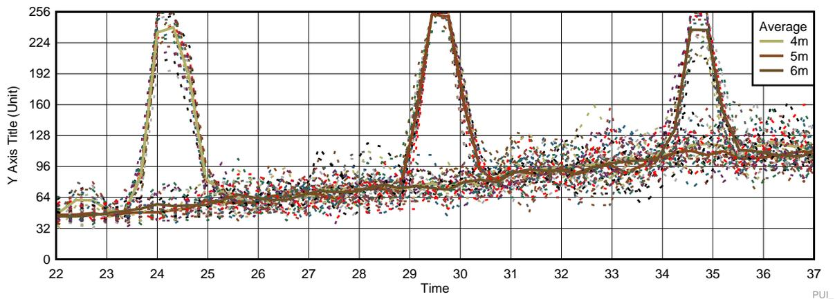
図 14. PUI Audio Long Range Echo Data Dump Performance at 4, 5, and 6 m
