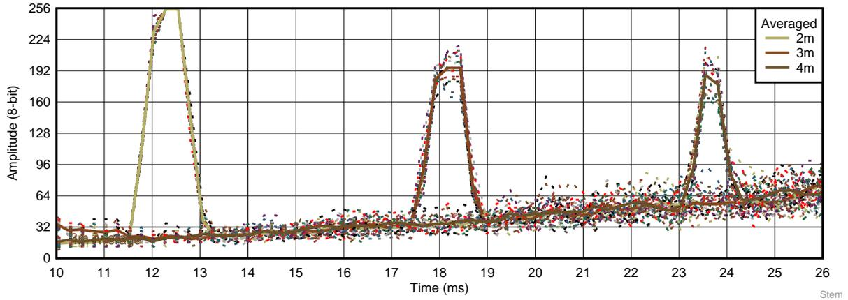
図 17. Steminc Long Range Echo Data Dump Performance at 2, 3, and 4 m
