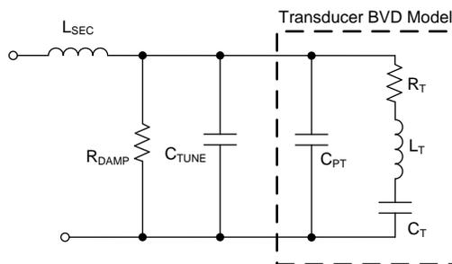
図 8. Transducer and Transformer Electrical Model With Tuning Components
