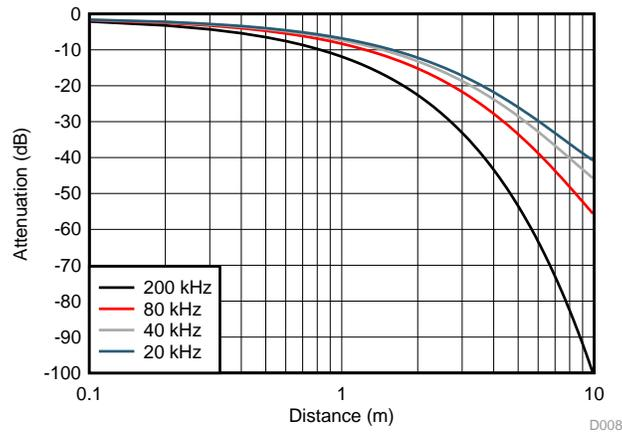
**図 4. Attenuation Characteristics of Sound Pressure by Distance**
