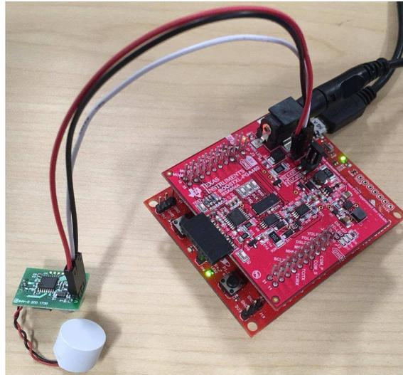
図 11. External OWI Evaluation Setup for PGA460PSM With Software Modification
