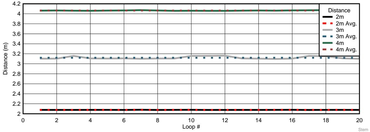
図 18. Steminc Long Range Measurement Results at 2, 3, and 4 m
