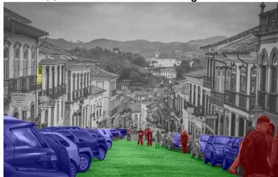
TI developed an example network model named as JacintoNet11 to demonstrate object classification, JDetNet model to demonstrate object detection and JSegNet21 to demonstrate pixel-level semantic segmentation.
