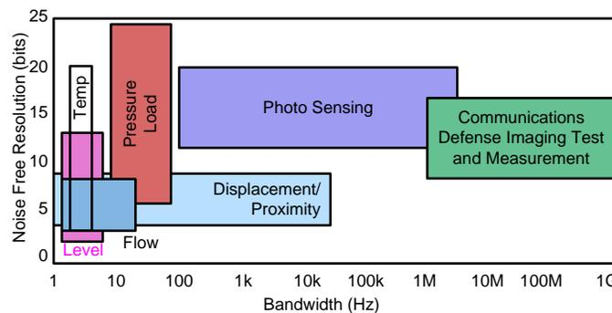
図 7. Noise-Free Resolution Versus Bandwidth
