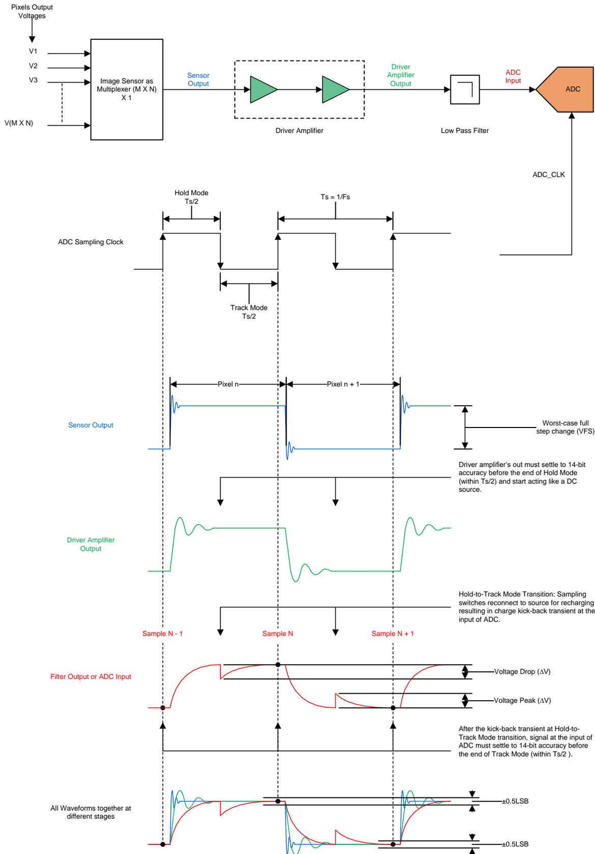
図 14. Waveforms at Different Stages in the Signal Chain
