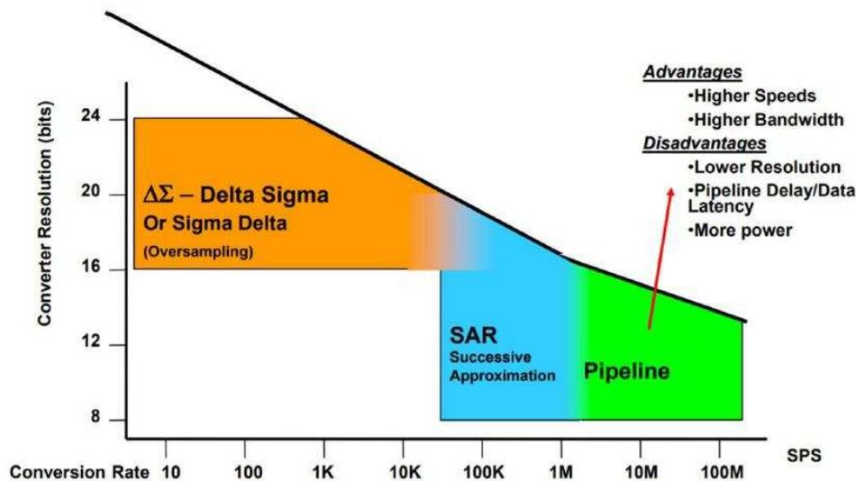
図 8. Converter Resolution Versus Conversion Rate
