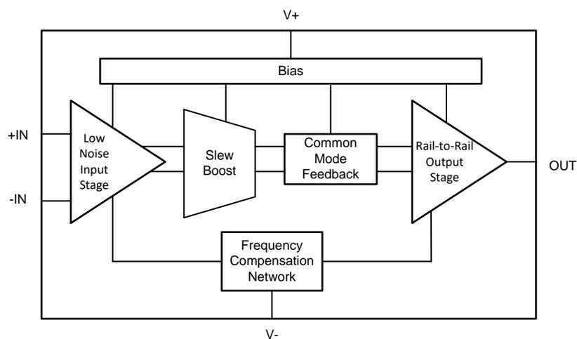
図 2. OPAx262 Functional Block Diagram
