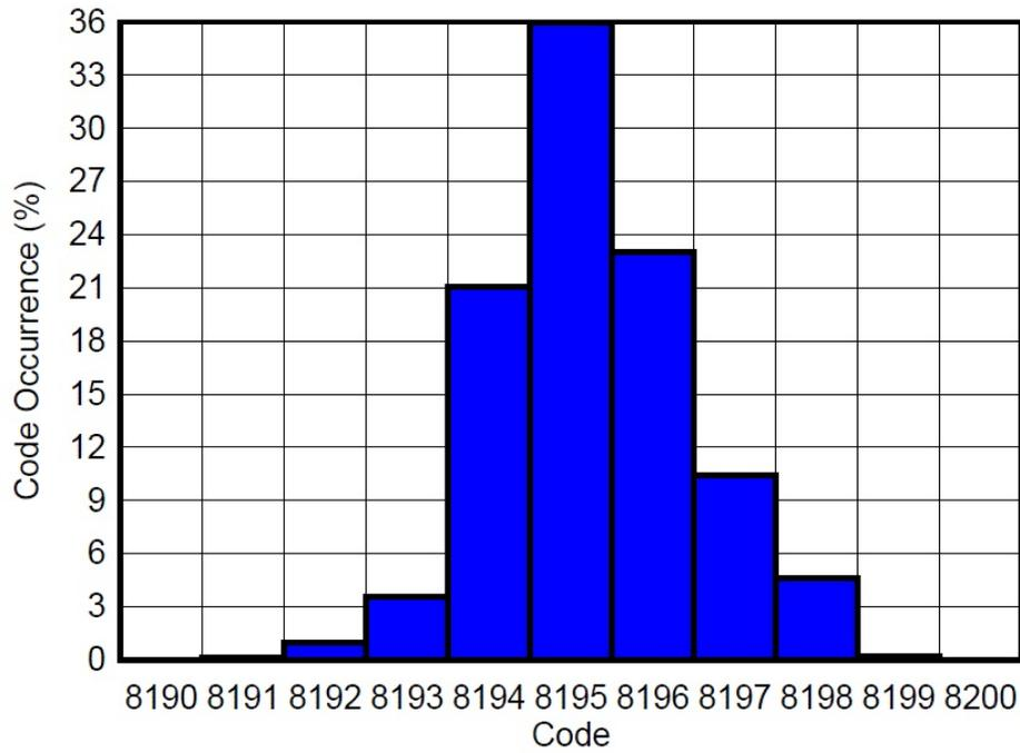
図 26. DC Input Histogram Test of ADC With Driver Amplifier
