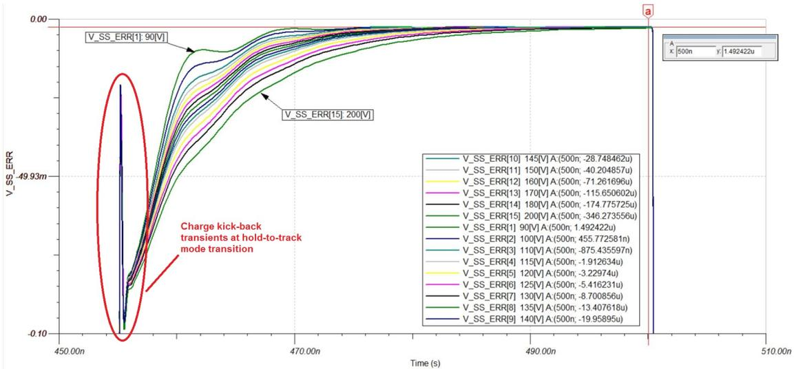
**Figure 20. Parameter Stepping Simulation for Filter Resistors from 90 Ω to 200 Ω**
