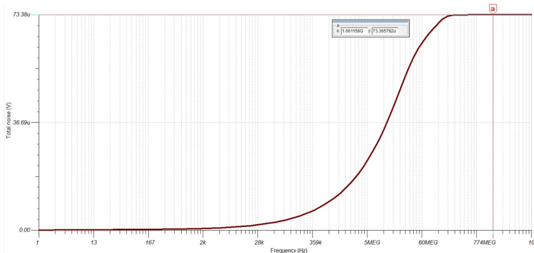
図 23. Total Output Noise of Front-End Amplifier
