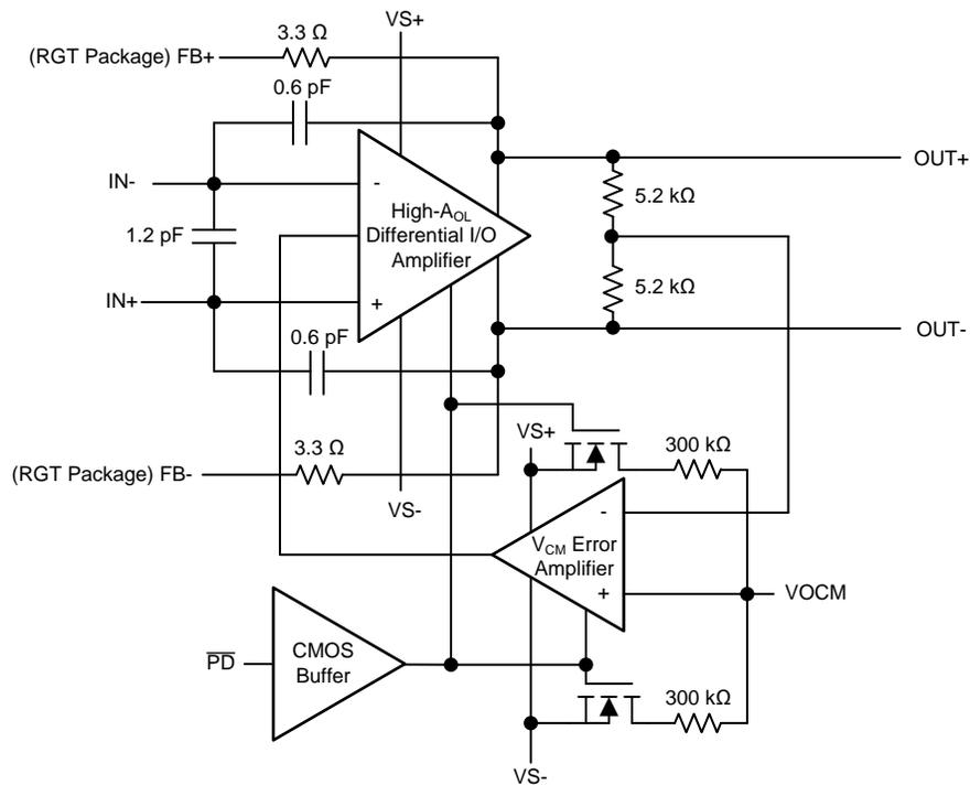
図 3. THS4551 Functional Block Diagram
