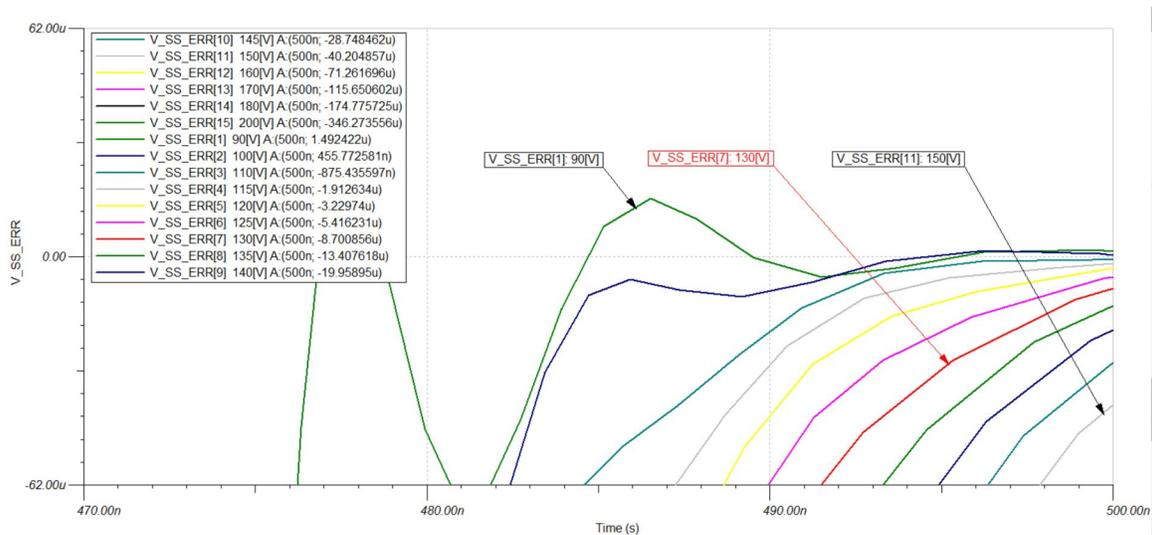
図 21. Parameter Stepping: Curves Settling Within  $\pm 0.5$  LSB
