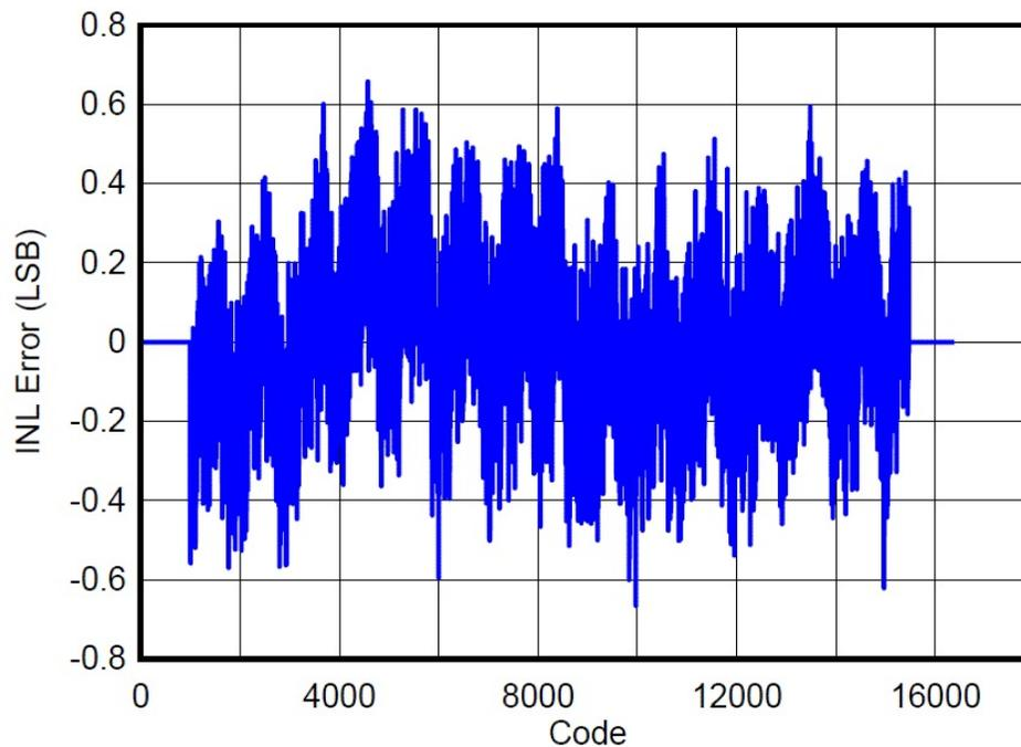
図 28. ADC INL Test With Driver Amplifier
