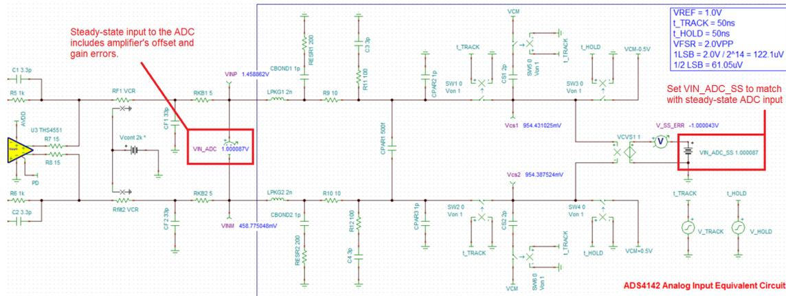
図 19. Run DC Analysis for Steady State ADC Input Voltage
