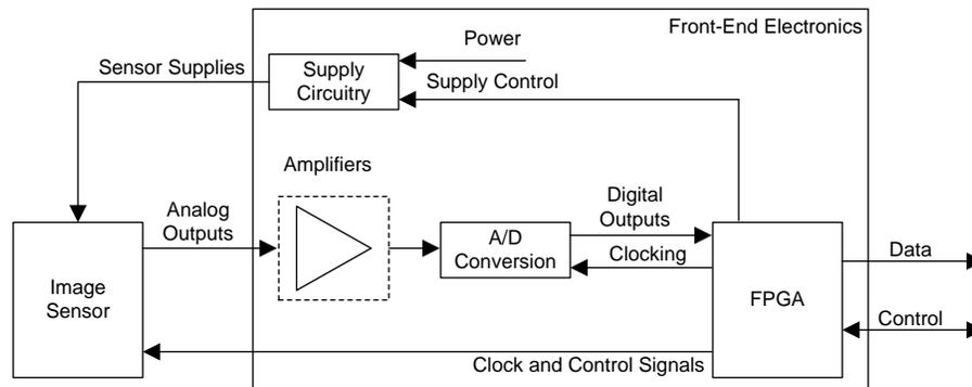
図 5. Basic Architecture of Camera Electronics
