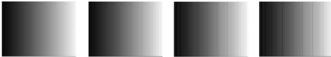
図 6. Smooth Gradient Scene With Increasing DNL Error
