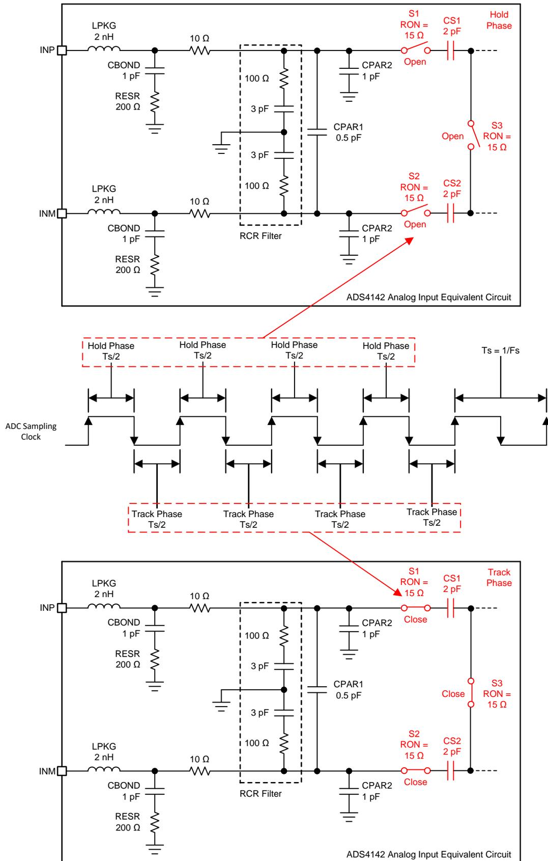
図 12. Sampling Switches S1 and S2
