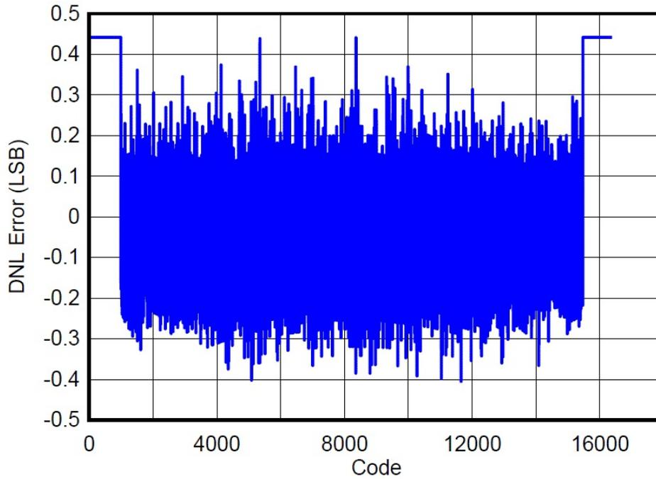
図 27. ADC DNL Test With Driver Amplifier
