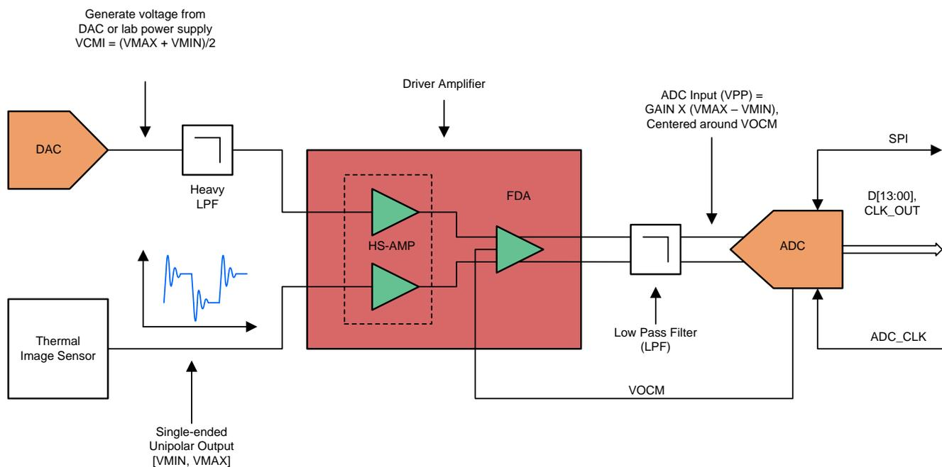
図 10. Conceptual Schematic of AFE Circuit for IR Imaging Applications
