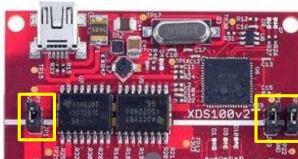
**Figure 13. F28379D Jumper Configuration**
