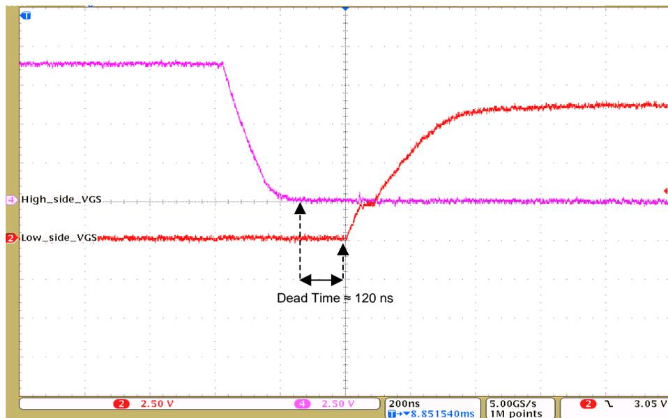
図 16. Dead Time at Rising Edge of Low-Side  $V_{GS}$
