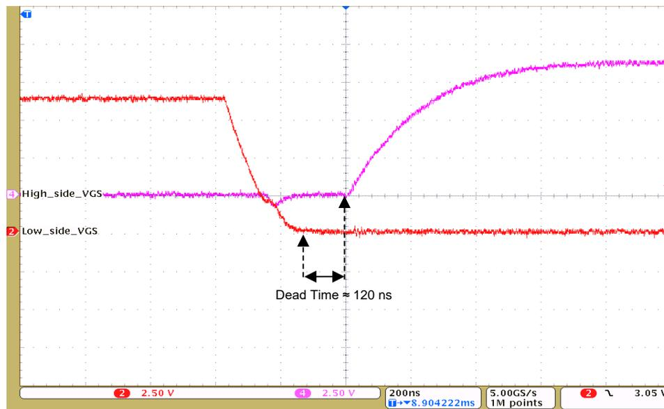
図 17. Dead Time at Trailing Edge of Low-Side  $V_{GS}$
