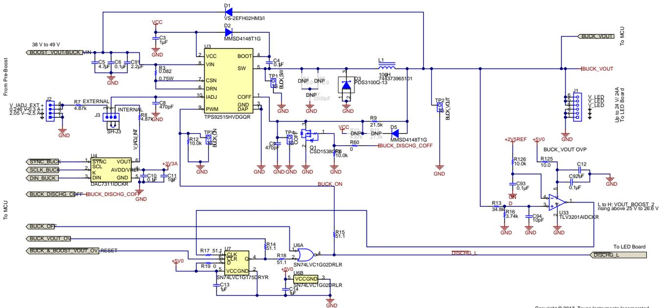
図 28. LED Buck With IADJ-DAC and OVP
