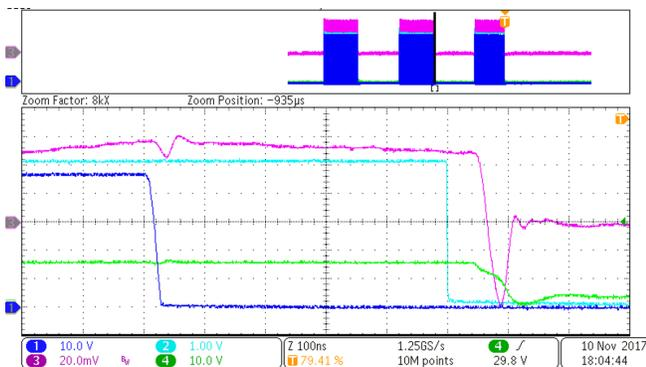
[Fig 60](#). LED Buck Normal Operation Control Through BUCK\_ON Signal, LED ON/OFF—Transition During  $t_{OFF}$
