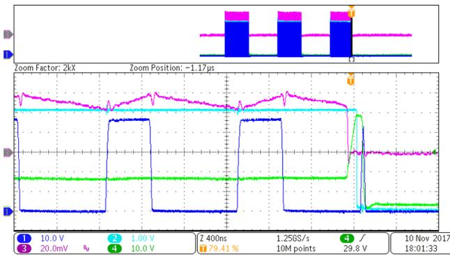
[Fig 58](#). LED Buck OVP—Third LED Pulse Stopped After Overvoltage Caused by Removing SH-J5
