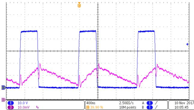
図 56. Buck Switch Node at 200 mA of LED Current
