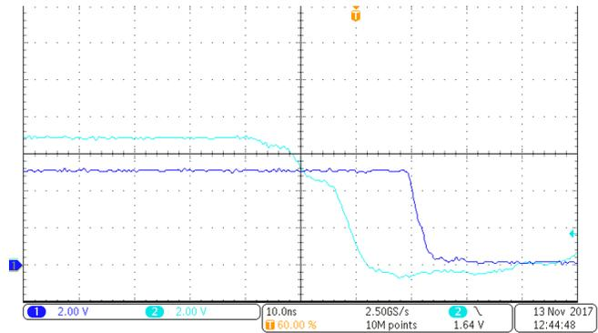
図 51. ISOW7842 Propagation Delay of 14 ns
