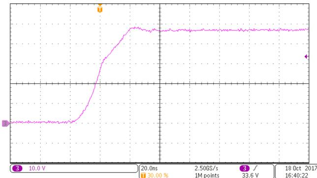
[Fig 64](#). Pre-Boost Switch Node, Rising, R34 = 15 Ω, R35 = 15 Ω
