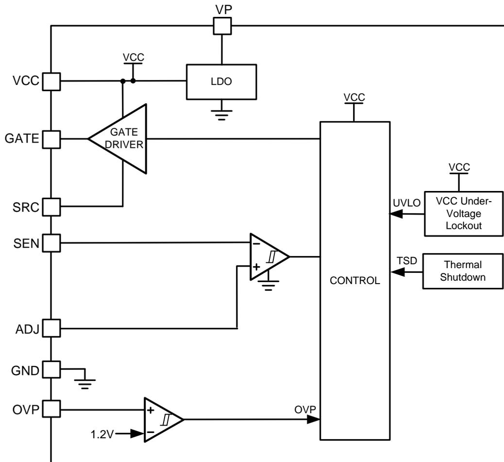
図 3. Functional Block Diagram of TPS92561
