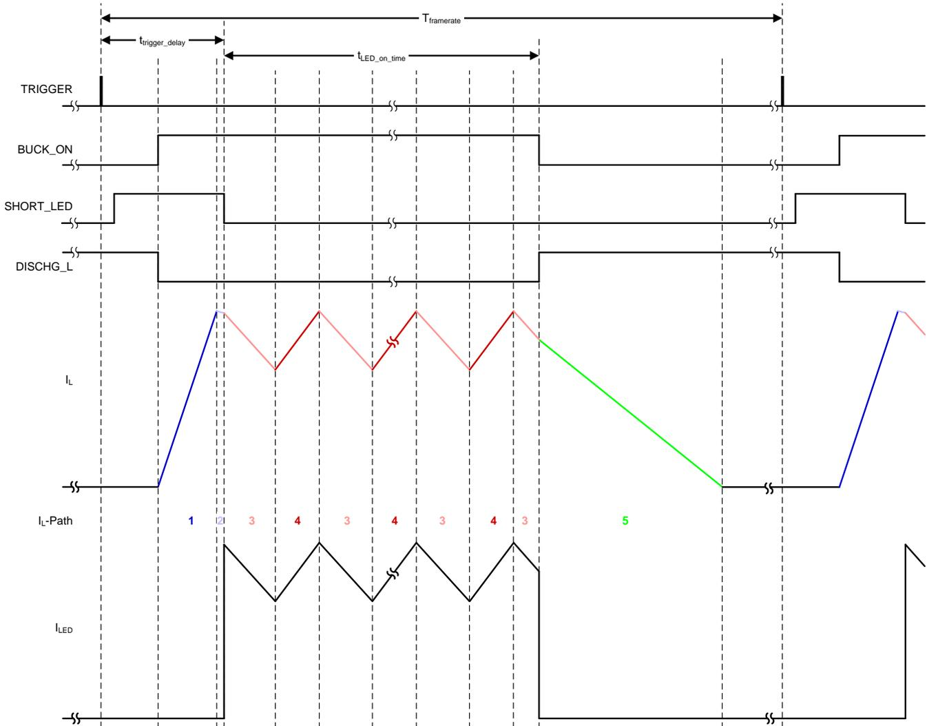
図 27. Timing Diagram of LED Buck and LED Board
