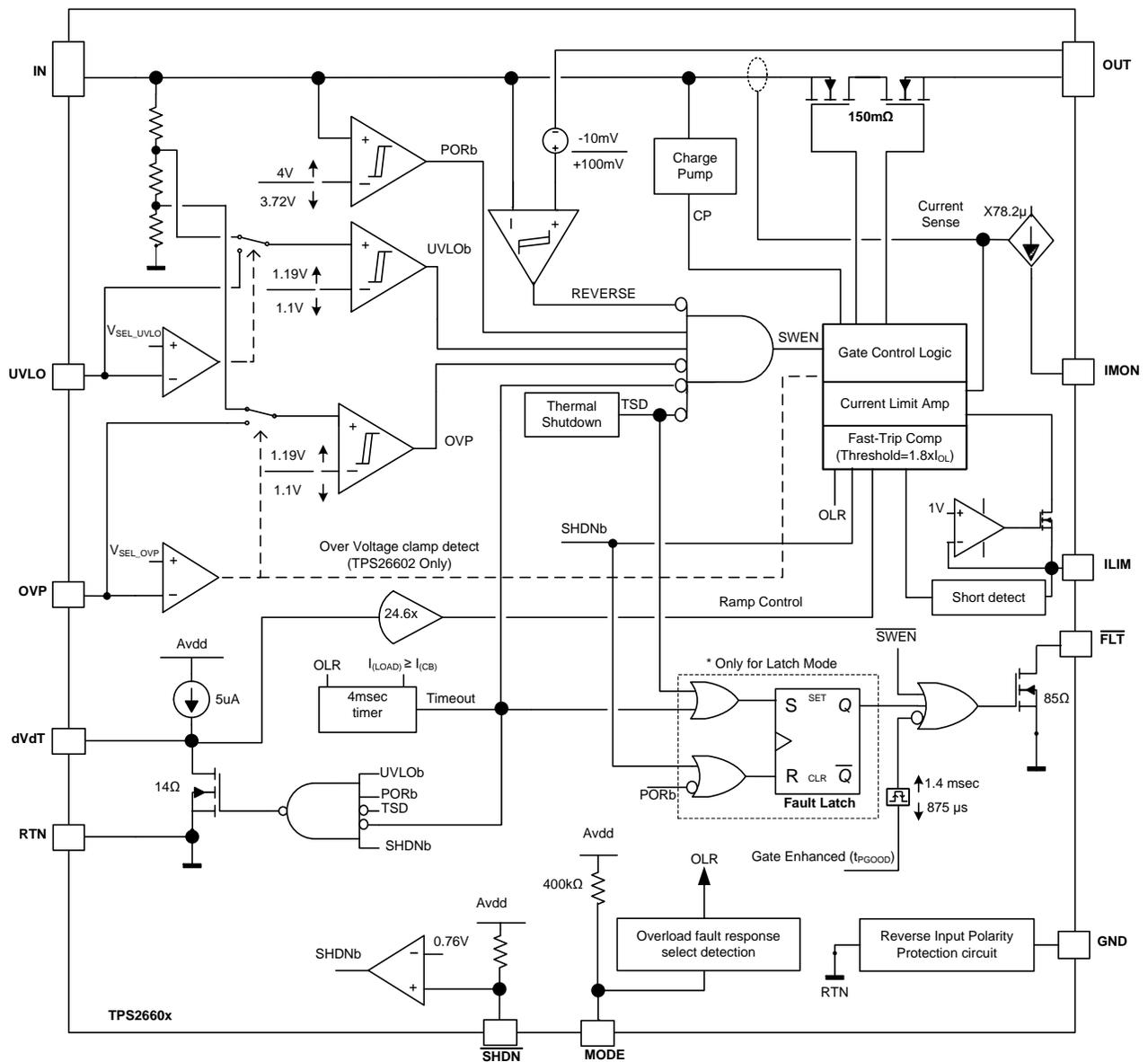
図 4. Functional Block Diagram of TPS2660x
