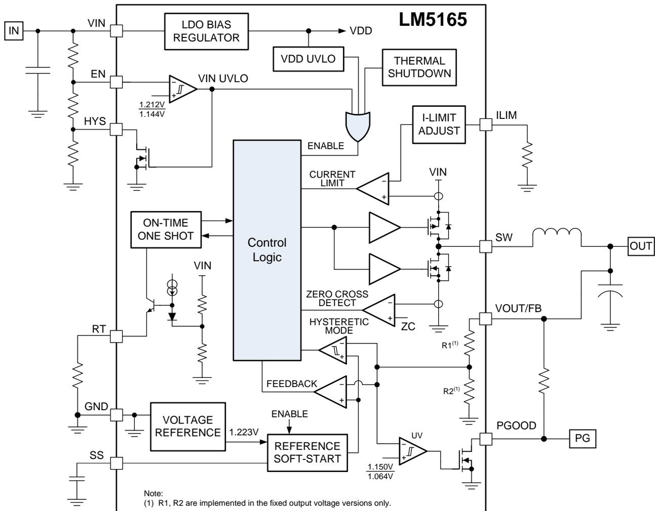
図 5. Functional Block Diagram of LM5165
