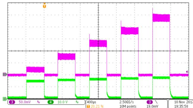
**Figure 48. Current Bracketing: On Time = 400  $\mu$ s, Frame Rate = 1428 Hz, N = 5, I<sub>LED</sub> = 200 mA, Current Brk = 550 mA, 5 Steps From 200 mA to 2.4 A in 4 Increments of 550 mA**
