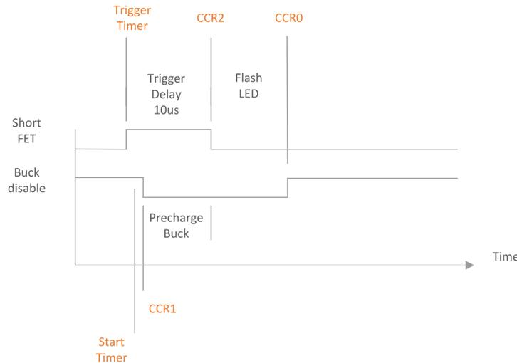
**Figure 35. Timing of Buck Regulator and Short FET**
