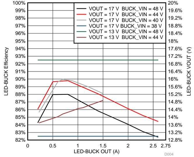
図 55. LED Efficiency and VOUT vs IOUT: Comparing Test With LED Board vs Resistive Load
