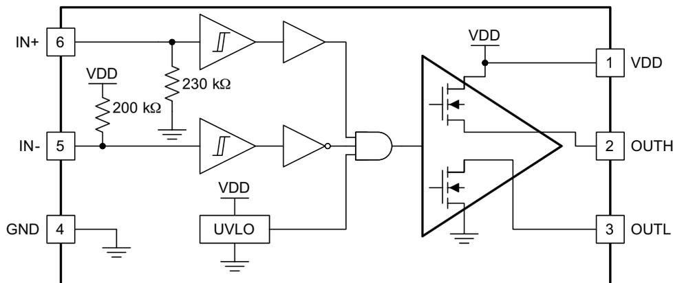
図 15. Functional Block Diagram of UCC27511
