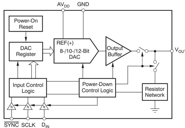
図 9. Functional Block Diagram of DAC7311
