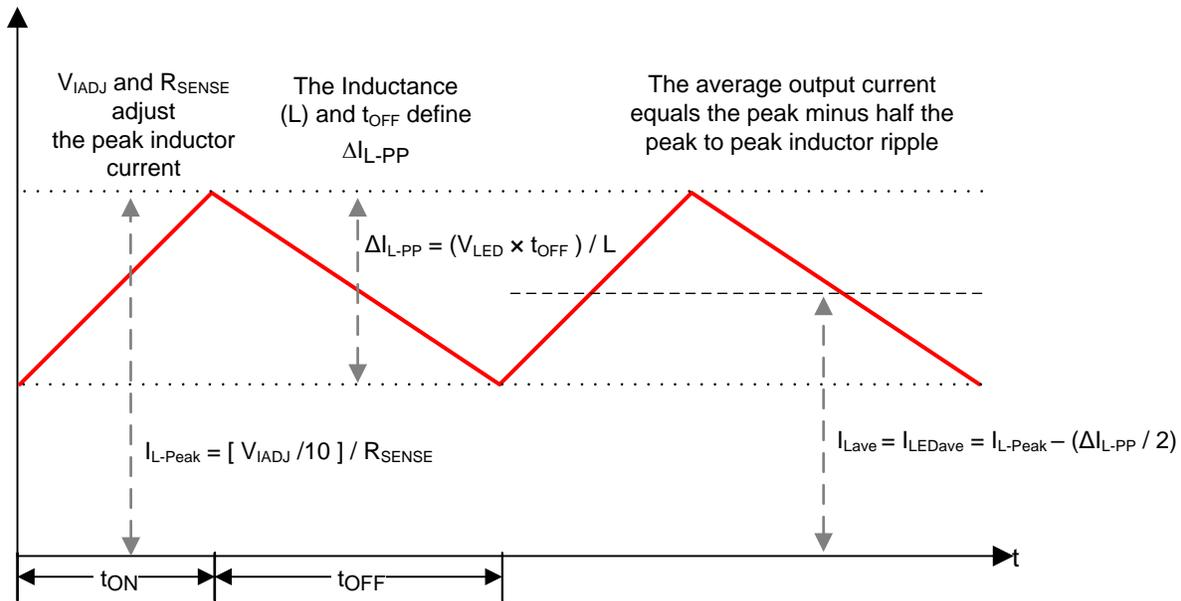
図 25. Principle of Hysteretic Operation: Constant Off-Time, Peak-Current Control
