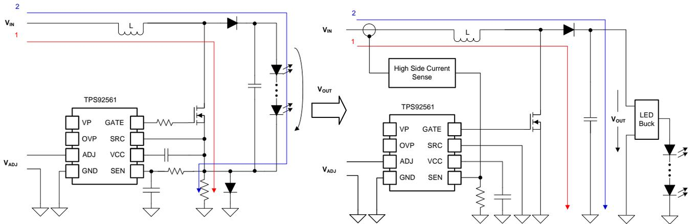
図 33. Pre-Boost Operation—Standard vs Modified Implementation and Input Current Waveform
