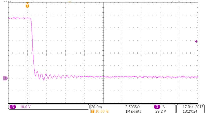
[Fig 63](#). Pre-Boost Switch Node, Falling, R34 = 0 Ω, R35 = 3.32 Ω
