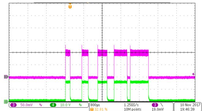
**Figure 49. Time Bracketing: On Time = 400  $\mu$ s, Frame Rate = 1428 Hz, N = 5, I<sub>LED</sub> = 1000 mA, Time Brk = 0.5**
