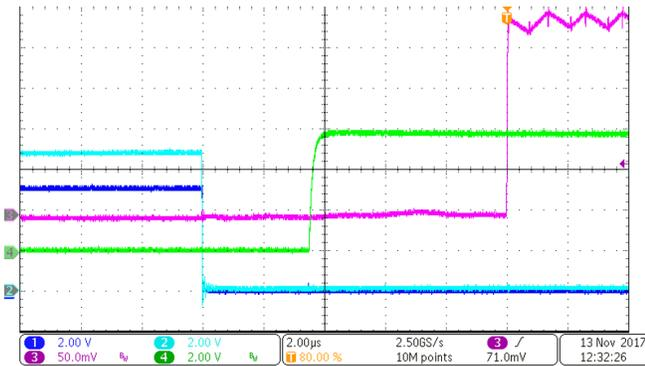
図 50. Trigger Delay of 10  $\mu$ s Fixed
