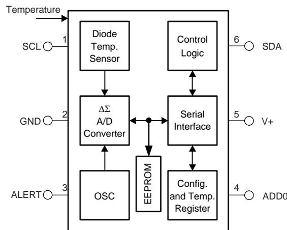
図 17. Functional Block Diagram of TMP116
