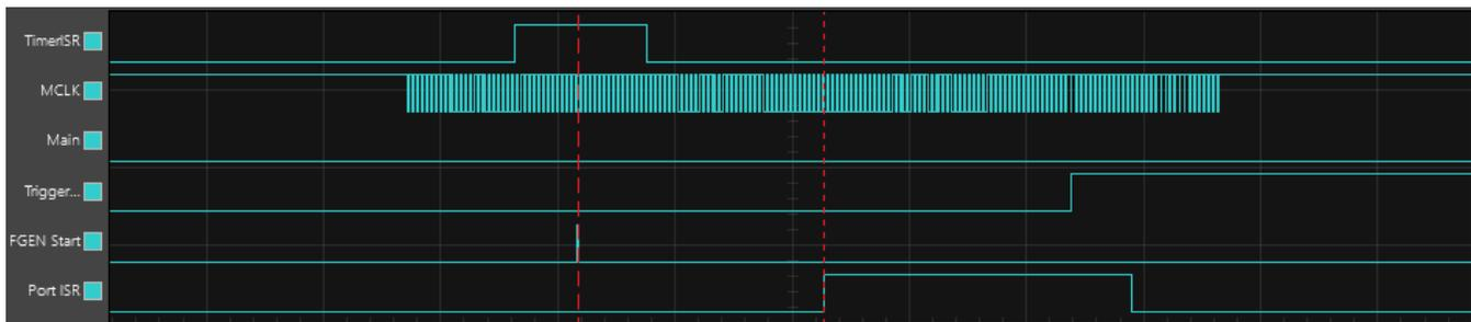
Figure 42. Jitter on External IRQ Caused by Timer (1  $\mu$ s/div)
