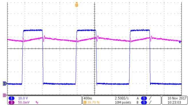
図 57. Buck Switch Node at 2400 mA of LED Current
