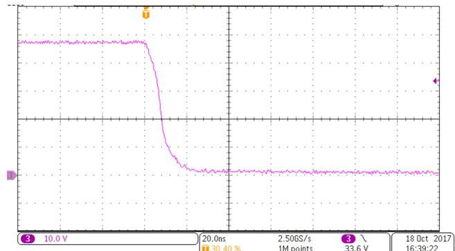
[Fig 65](#). Pre-Boost Switch Node, Falling, R34 = 15 Ω, R35 = 15 Ω
