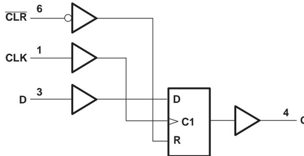
図 18. Functional Block Diagram of SN74LVC1G175
