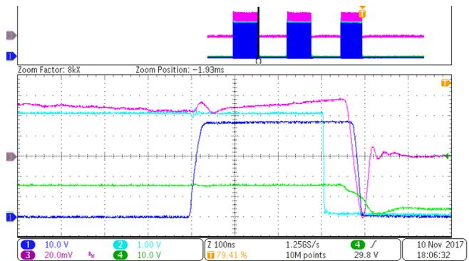
[Fig 61](#). LED Buck Normal Operation Control Through BUCK\_ON Signal, LED ON/OFF—Transition During  $t_{ON}$
