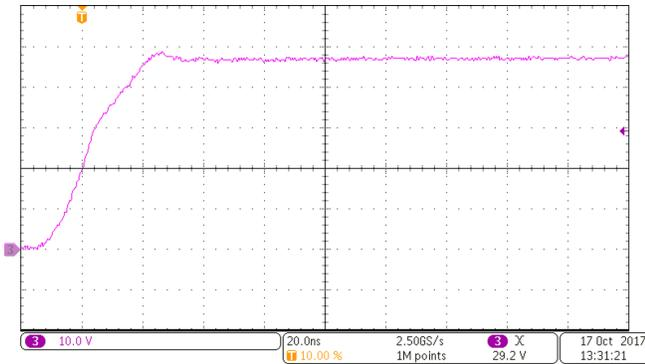
[Fig 62](#). Pre-Boost Switch Node, Rising, R34 = 0 Ω, R35 = 3.32 Ω
