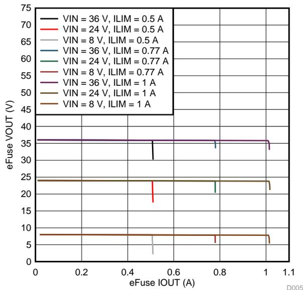
☒ 70. VOUT vs IOUT for Selectable Current Limit
