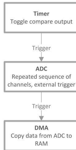
図 38. ADC Operation Optimized for Low CPU Load
