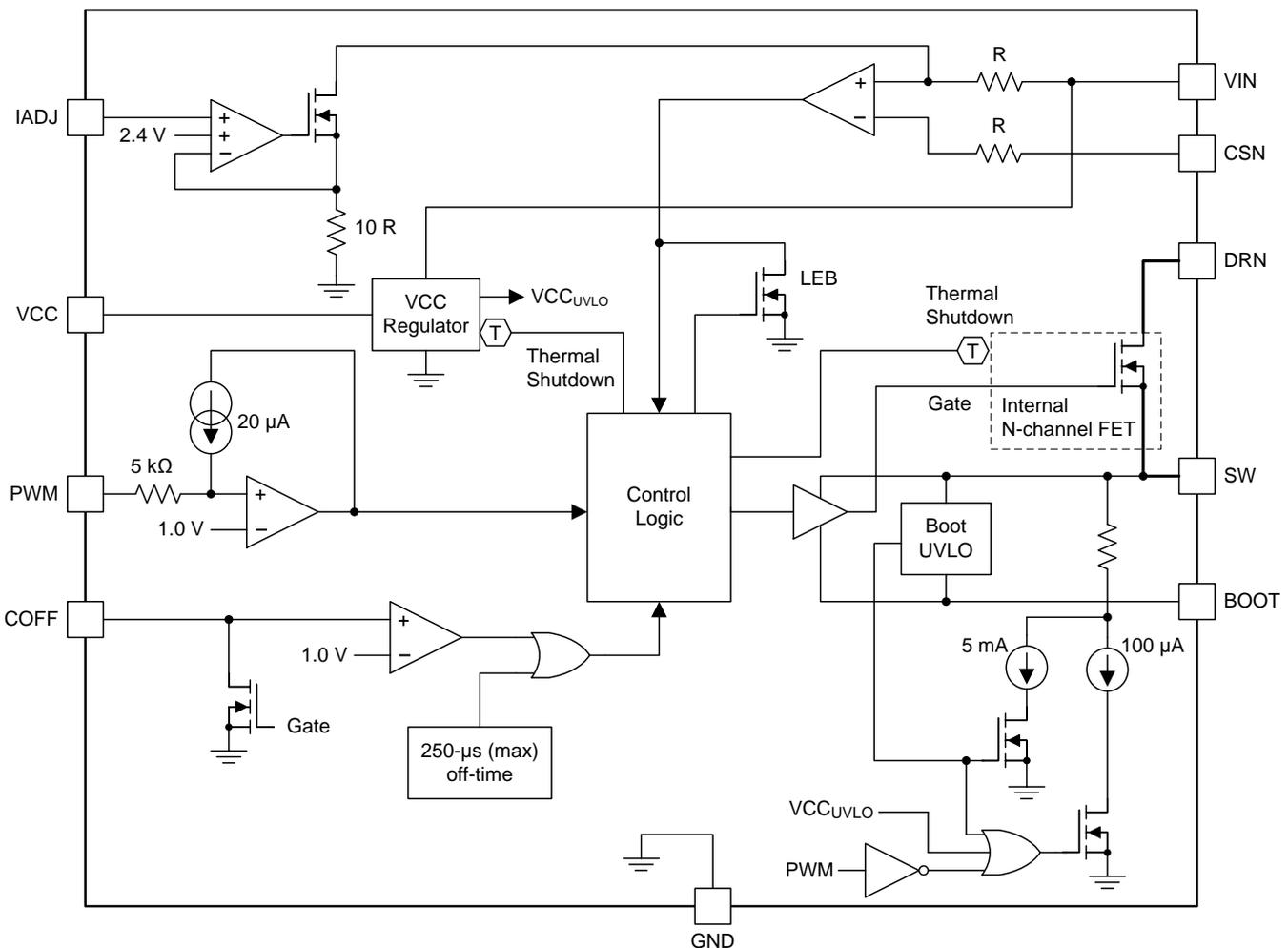
図 2. Functional Block Diagram of TPS92515HV
