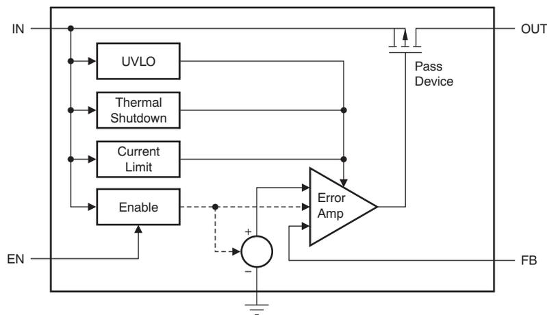
図 14. Functional Block Diagram of TPS7A4101
