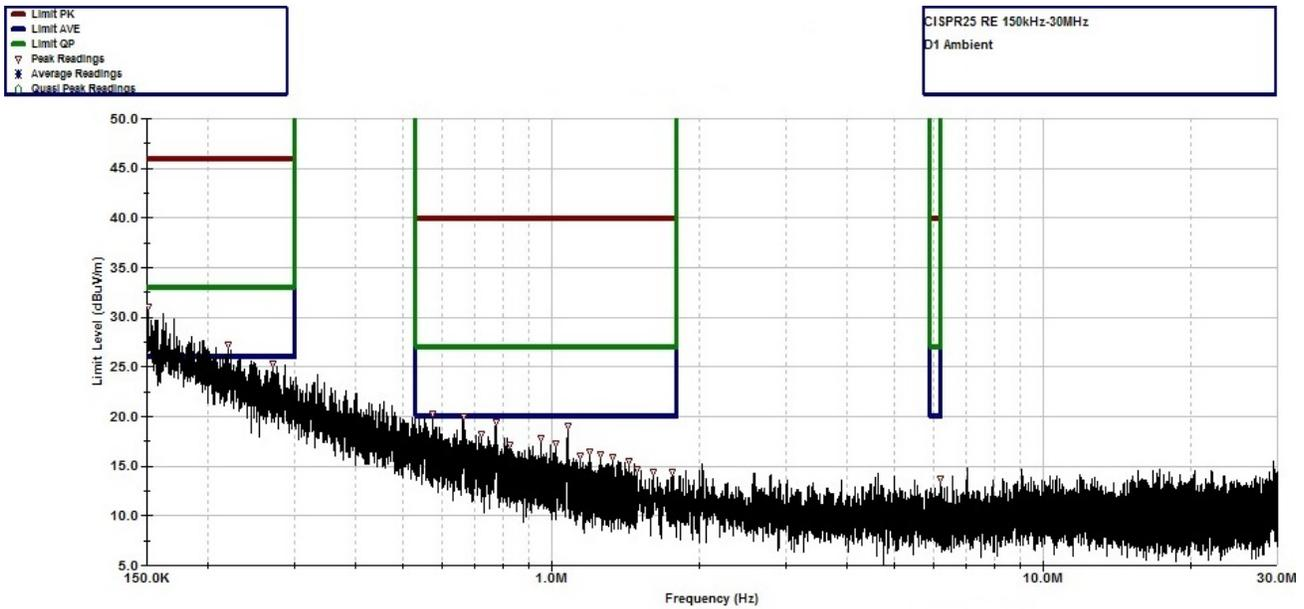
Figure 32. CISPR 25 Radiated Emissions: 150 kHz to 30 MHz, Ambient
