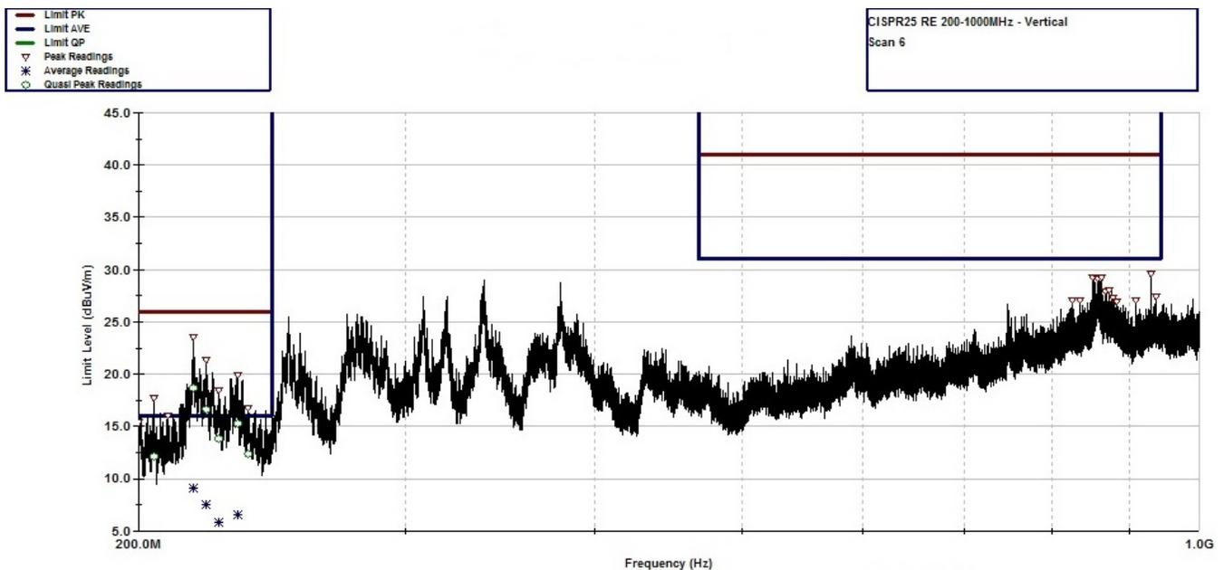
図 41. CISPR 25 Radiated Emissions: 200 MHz to 1 GHz, Vertical Antenna Orientation
