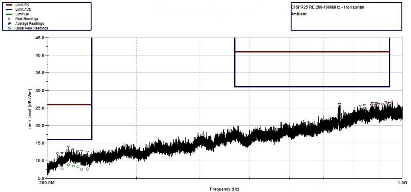
**Fig 38. CISPR 25 Radiated Emissions: 200 MHz to 1 GHz, Horizontal Antenna Orientation, Ambient Scan**
