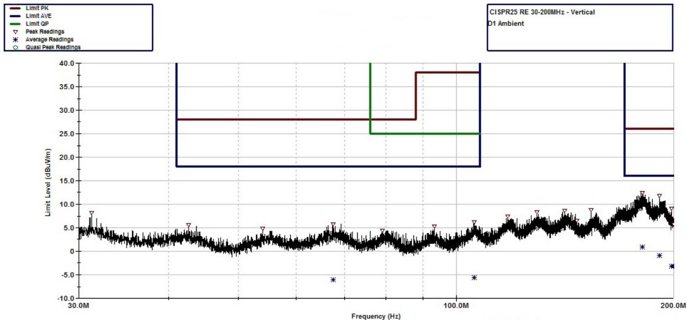
**Fig 35. CISPR 25 Radiated Emissions: 30 MHz to 200 MHz, Vertical Antenna Orientation, Ambient Scan**
