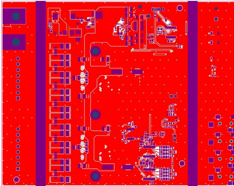
図 42. TIDA-00733 Top Circuit Board—Top Layer
