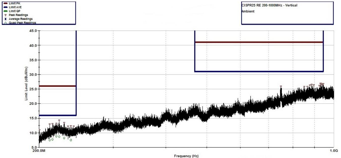
**Fig 39. CISPR 25 Radiated Emissions: 200 MHz to 1 GHz, Vertical Antenna Orientation, Ambient Scan**
