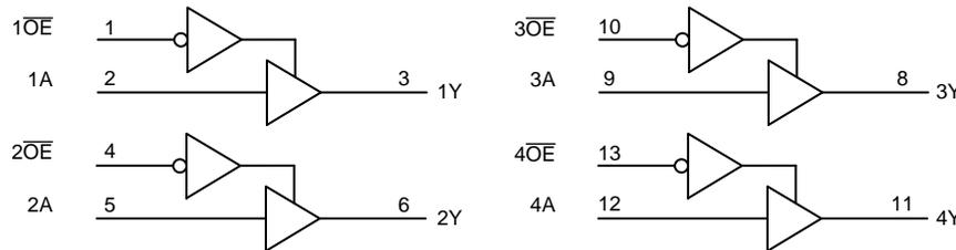
**Figure 8. SN74LVC125A-Q1 Logic Diagram (Positive Logic)**
