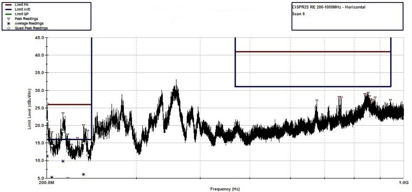
図 40. CISPR 25 Radiated Emissions: 200 MHz to 1 GHz, Horizontal Antenna Orientation
