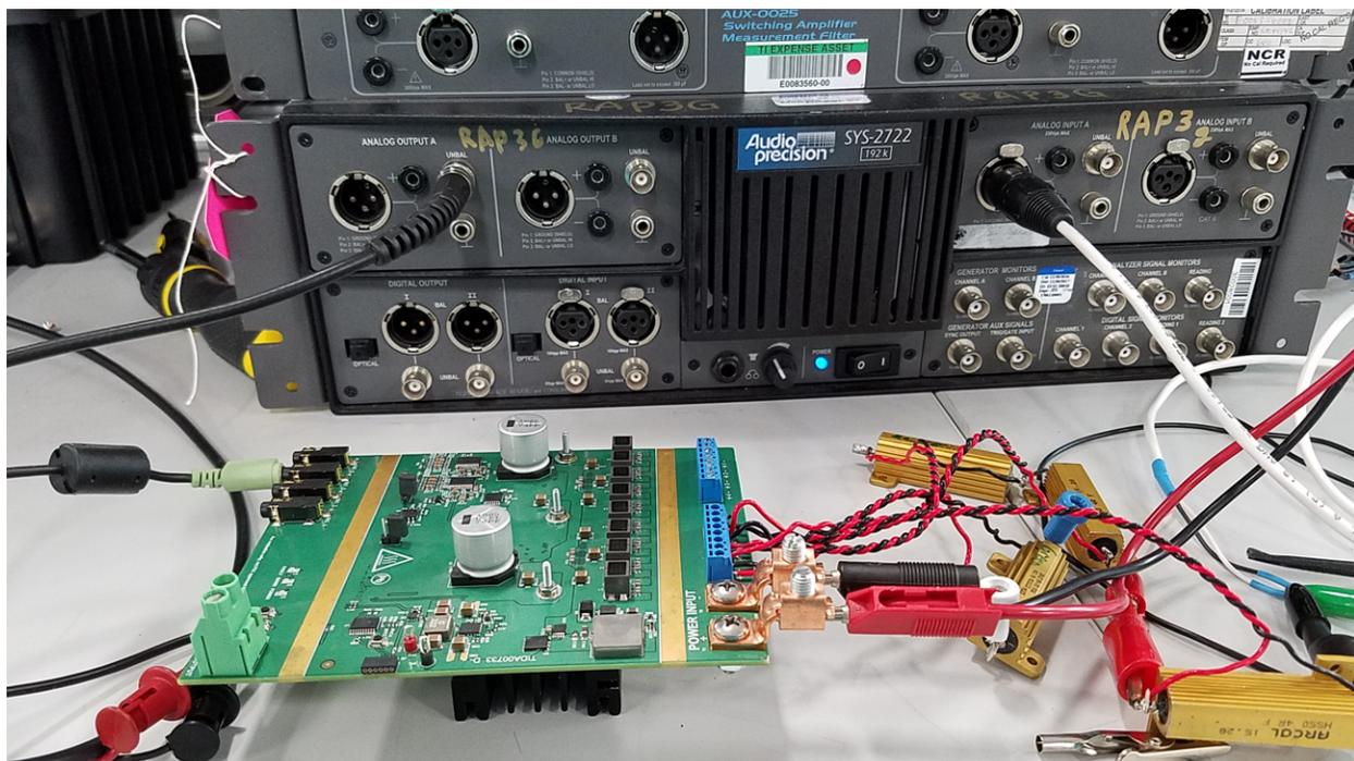
図 26. Test Setup for Power Output and Total Harmonic Distortion and Noise Tests
