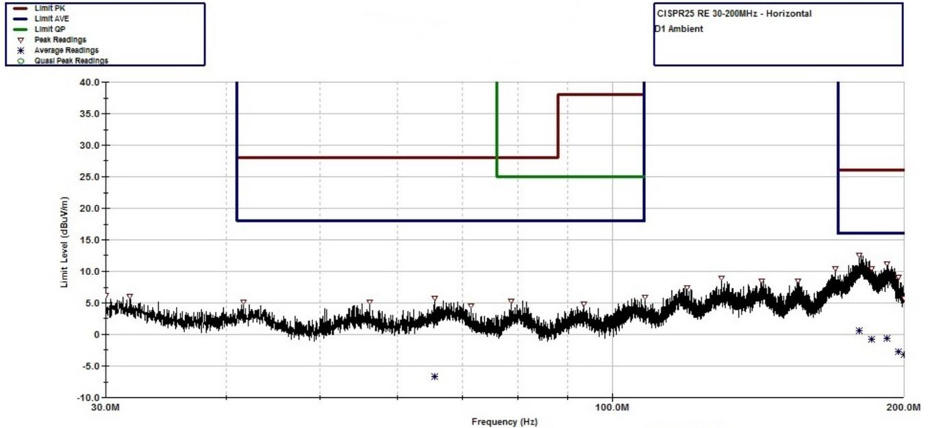
**Fig 34. CISPR 25 Radiated Emissions: 30 MHz to 200 MHz, Horizontal Antenna Orientation, Ambient Scan**
