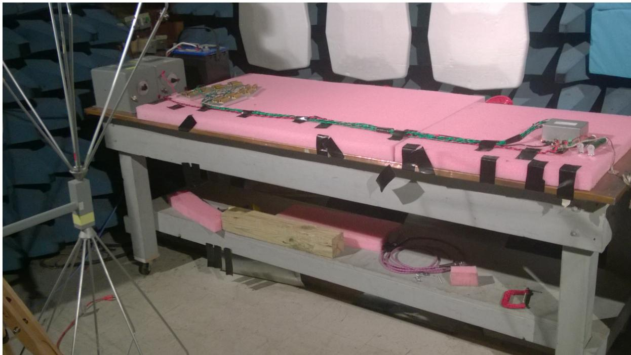
**図 29. Radiated Emissions Test Setup**
