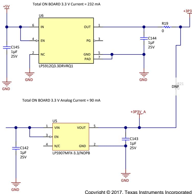
Figure 15. LP5912-Q1 and LP5907-Q1 Circuits
