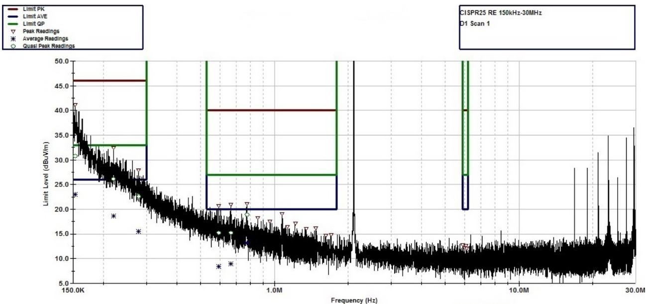
Figure 33. CISPR 25 Radiated Emissions: 150 kHz to 30 MHz
