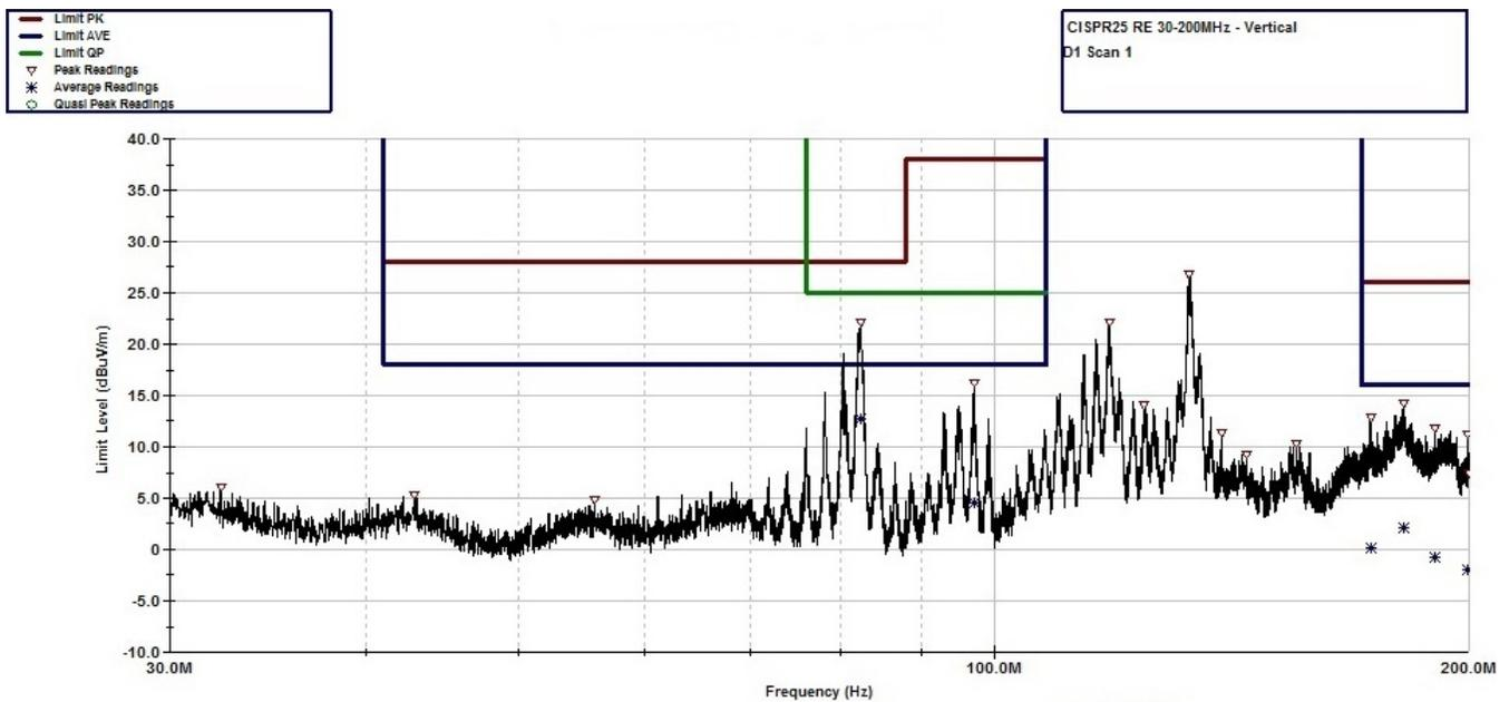
図 37. CISPR 25 Radiated Emissions: 30 MHz to 200 MHz, Vertical Antenna Orientation
