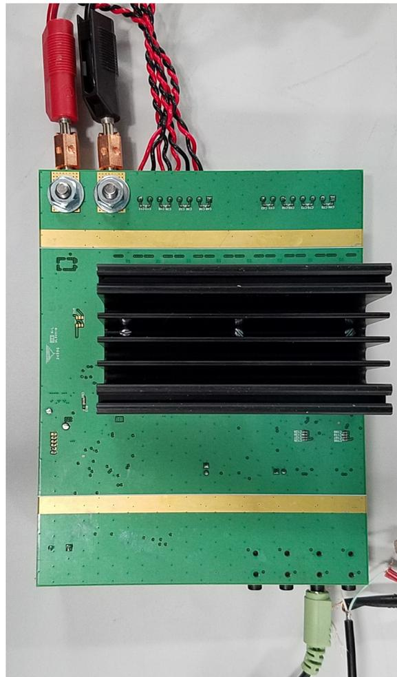
図 23. TIDA-00733 Board With Heat Sink
