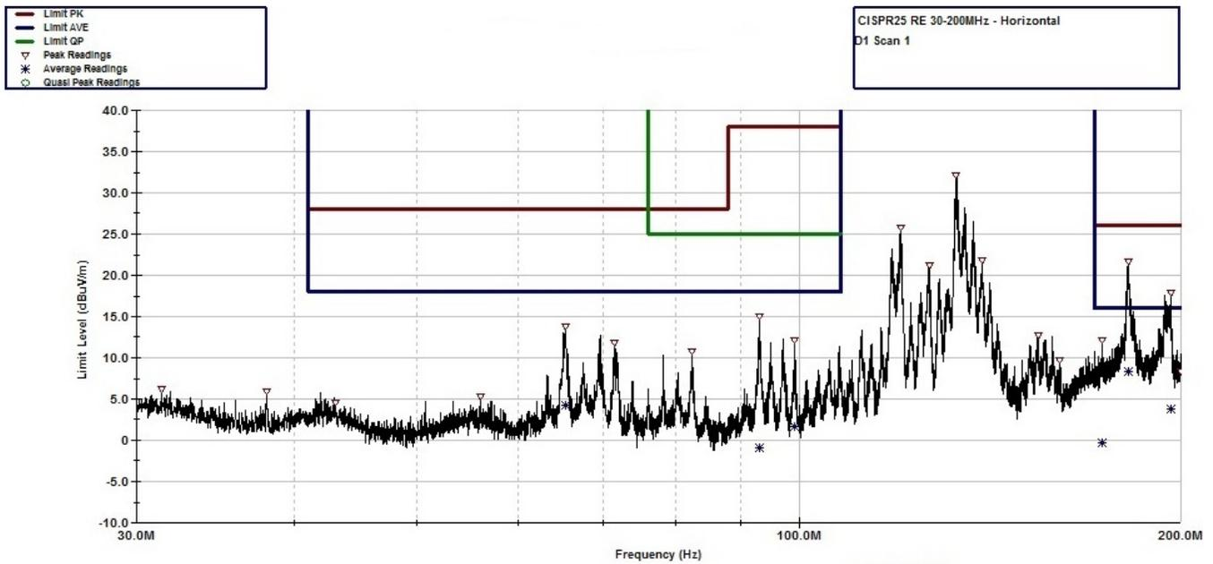
図 36. CISPR 25 Radiated Emissions: 30 MHz to 200 MHz, Horizontal Antenna Orientation
