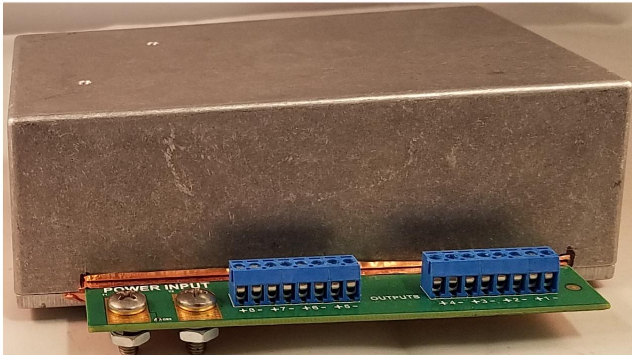
**Figure 27. TIDA-00733 in Metal Box for EMI Tests**
