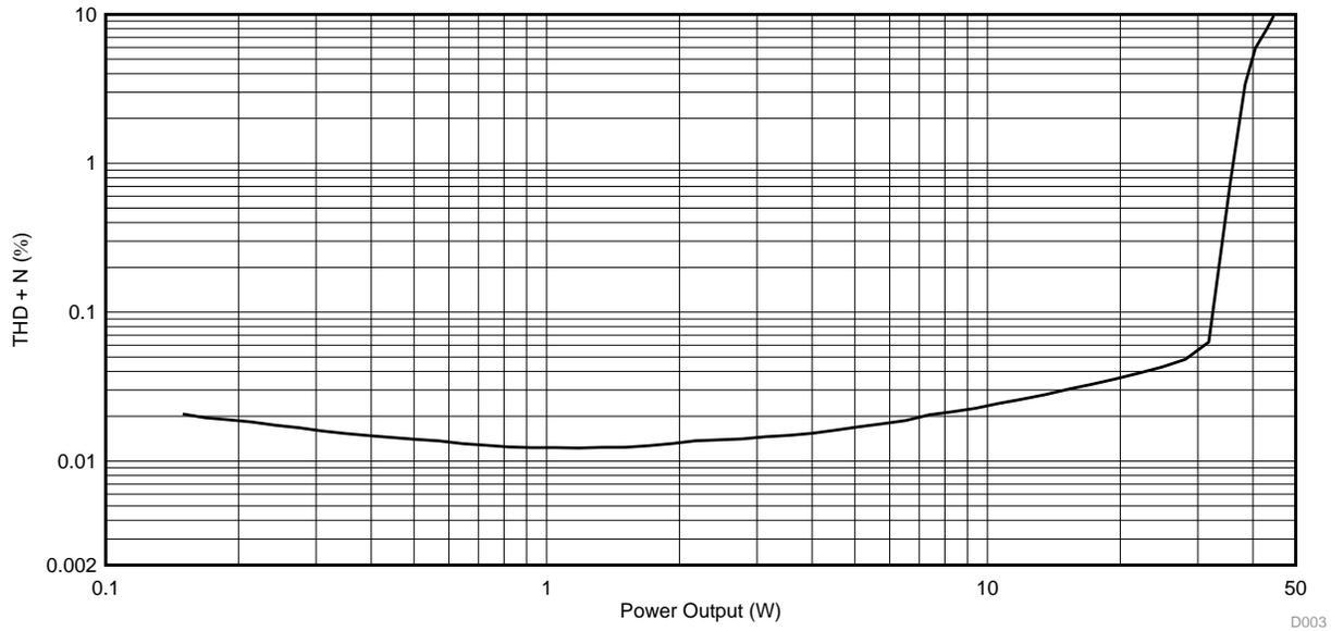
30. Power Output (W) vs THD + Noise (%) into 2 Ω
