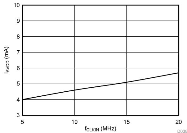
図 11. AMC1304 High-Side Current Consumption versus Clock Frequency
