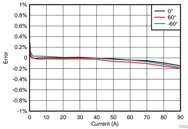
**図 42. Cumulative Active Energy % Error Versus Current, 220- $\mu\Omega$  Shunts**
