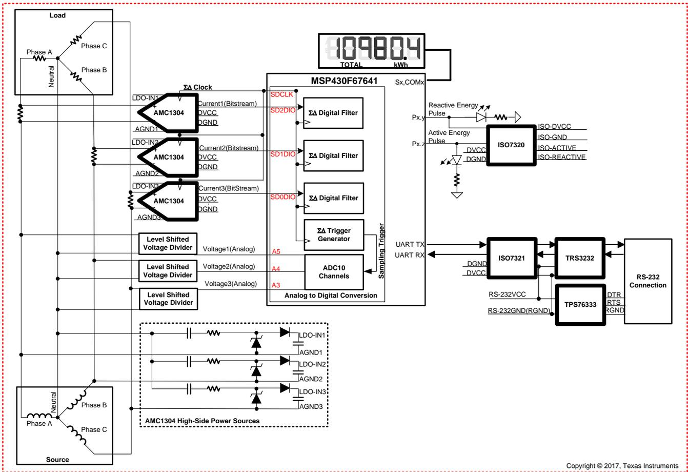
図 5. System Block Diagram for AMC1304 Configuration
