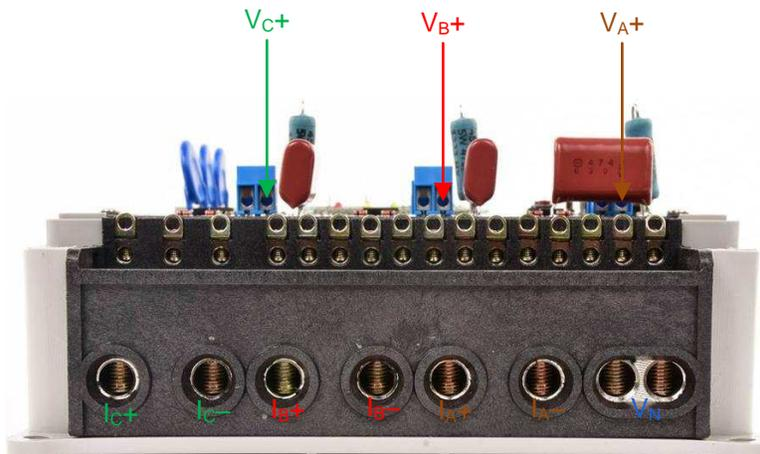
**図 24. Front View of EVM With Test Setup Connections With Current and Voltage Disconnected**
