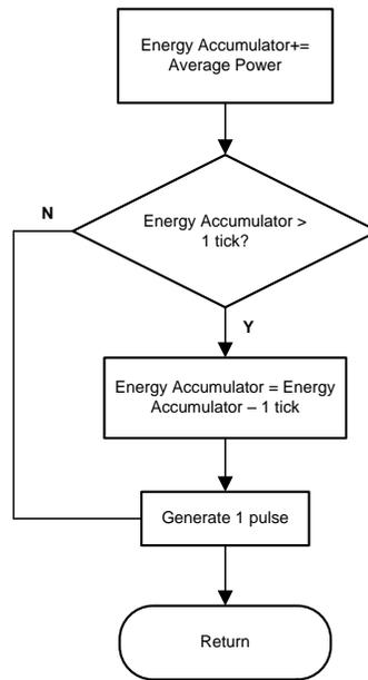
図 17. Pulse Generation for Energy Indication
