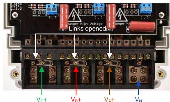
☒ 22. Top View of EVM With Test Setup Connections With Current and Voltage Disconnected
