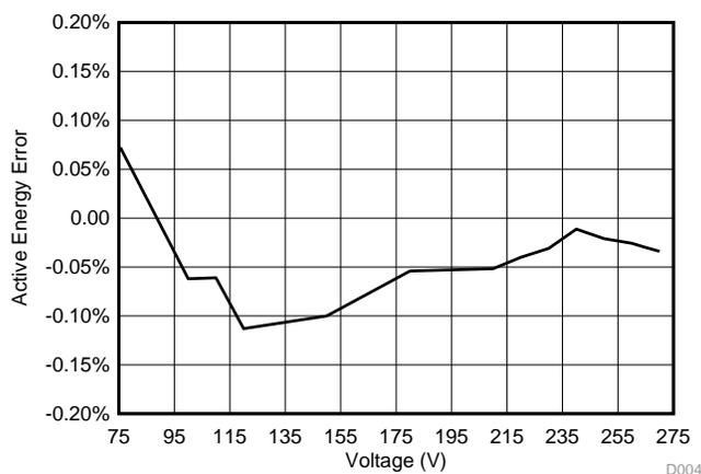
**図 44. Cumulative Active Energy Measurement Error Versus Voltage, 57.5 to 270 V**
