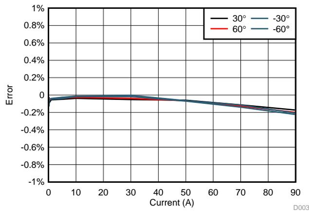
**図 43. Cumulative Reactive Energy % Error Versus Current**
