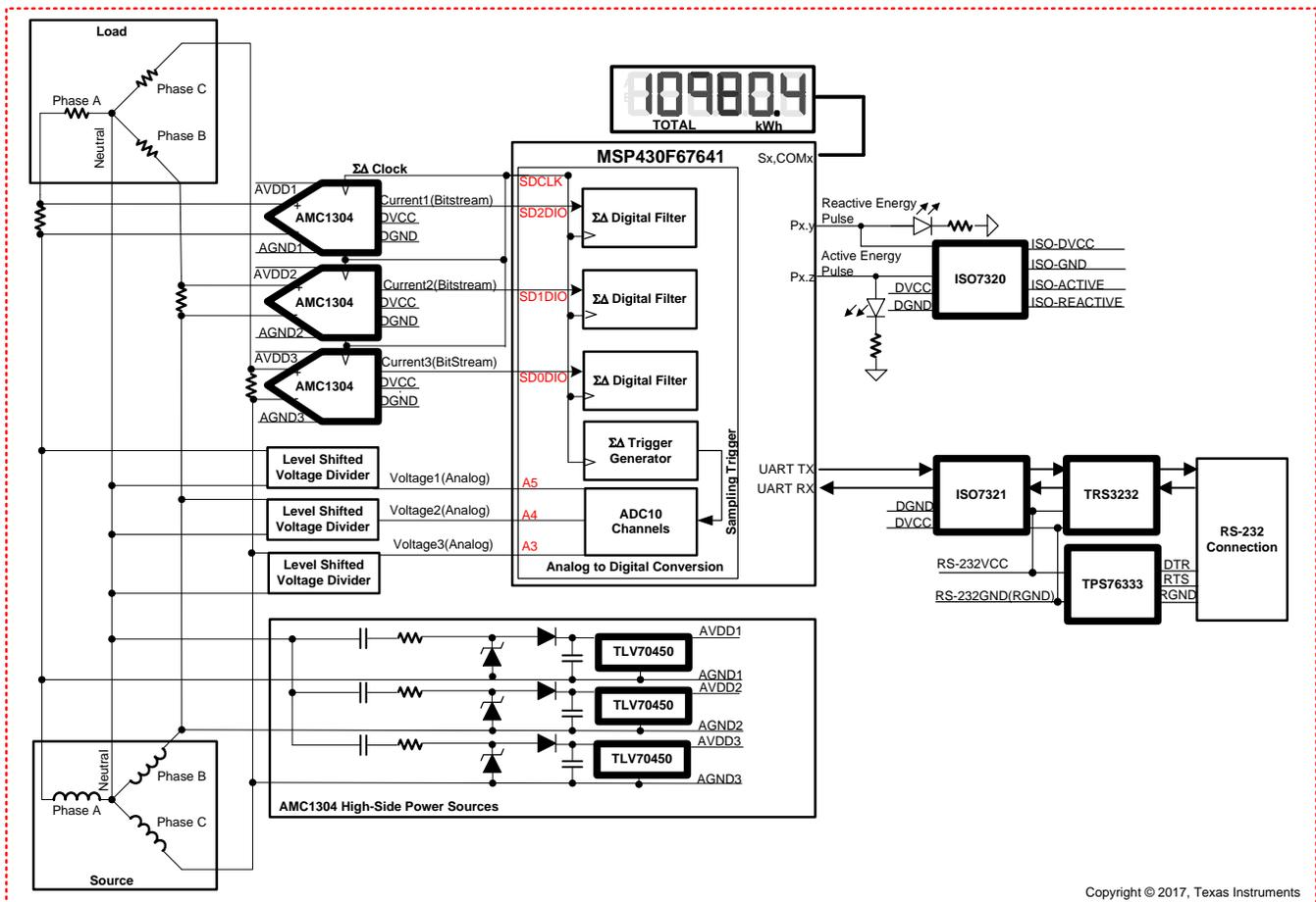
図 6. System Block Diagram for AMC1305 Configuration
