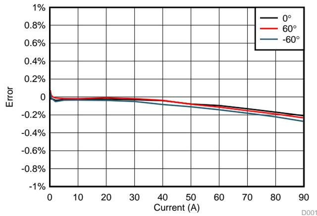
**図 41. Cumulative Active Energy % Error Versus Current, 400- $\mu\Omega$  Shunts**
