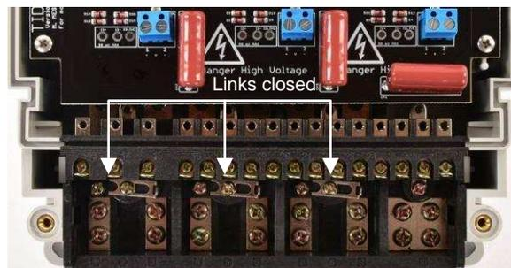
☒ 21. Top View of EVM With Test Setup Connections With Current and Voltage Connected
