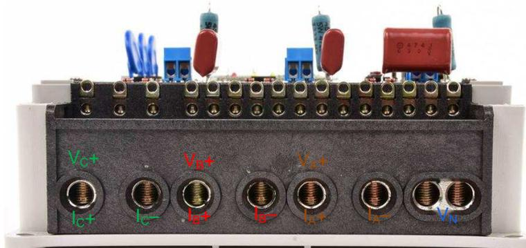
**図 23. Front View of EVM With Test Setup Connections With Current and Voltage Connected**
