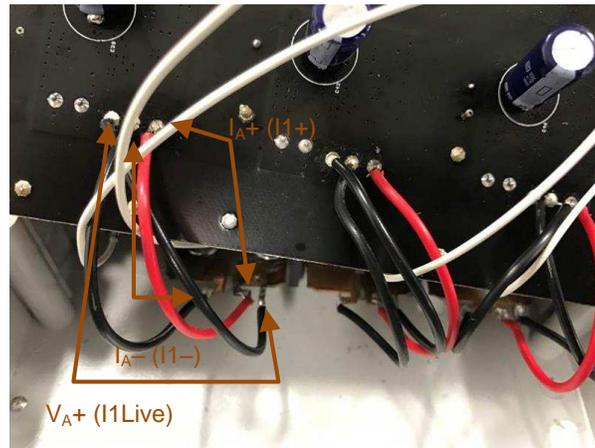
☒ 20. Mapping Between Shunt Terminals and Ix Current Pads
