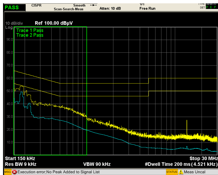
図 2-15. HS LISN — UCC33420 5V/5V Pout = 1.5W
