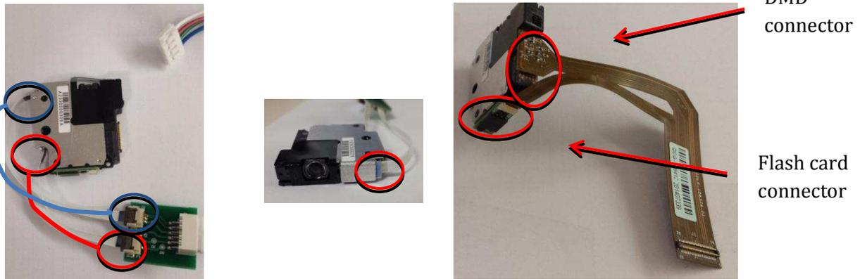
**Figure 7. LED Connection and Flex Cable Connection**
