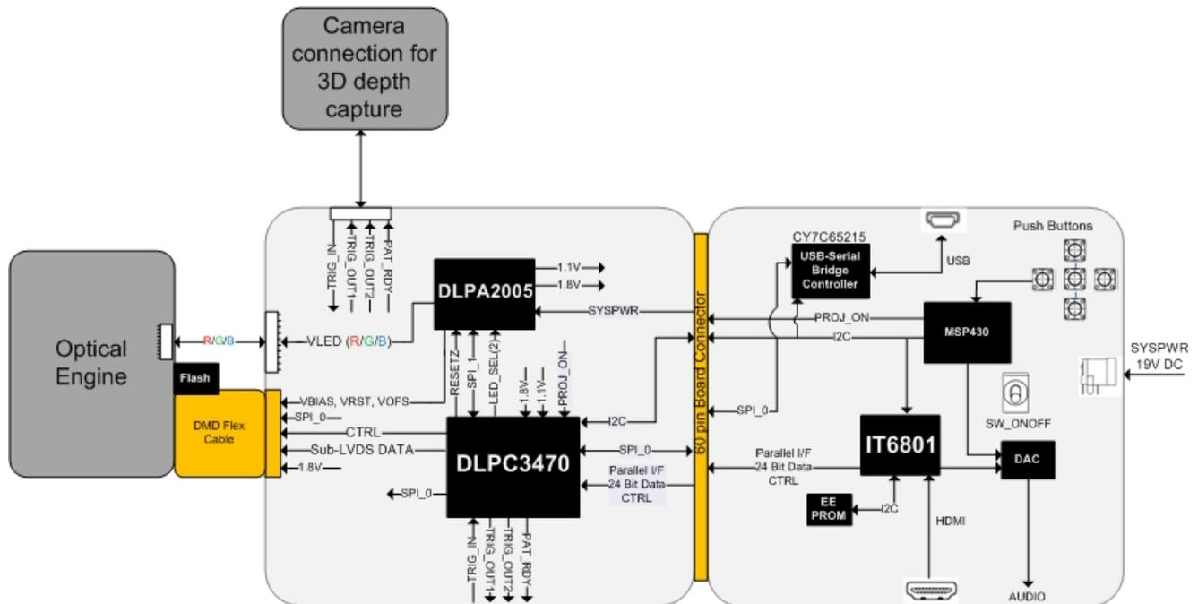
Figure 2. DLP2010 Light Control EVM Block Diagram
