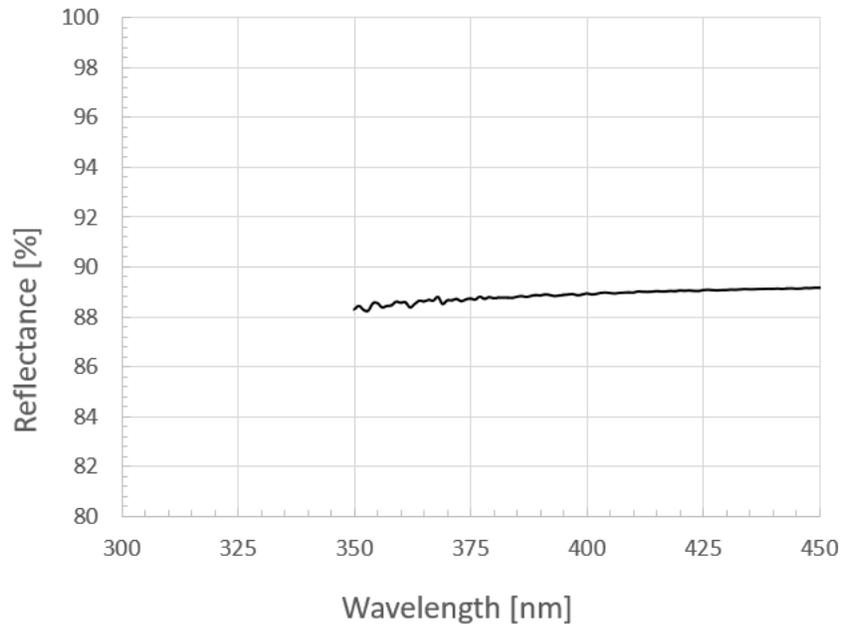
**Figure 2-1. Mirror Reflectivity versus Wavelength (UV)**
