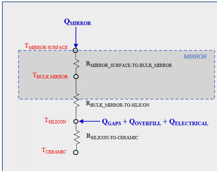
**Figure 1-1. Simplified DMD Thermal Resistor Network**
