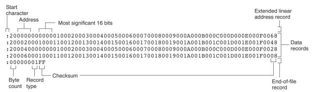
Figure 12-9. Intel Hexadecimal Object Format
