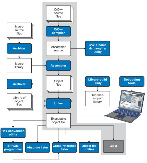
Figure 1-1. ARM Device Software Development Flow
