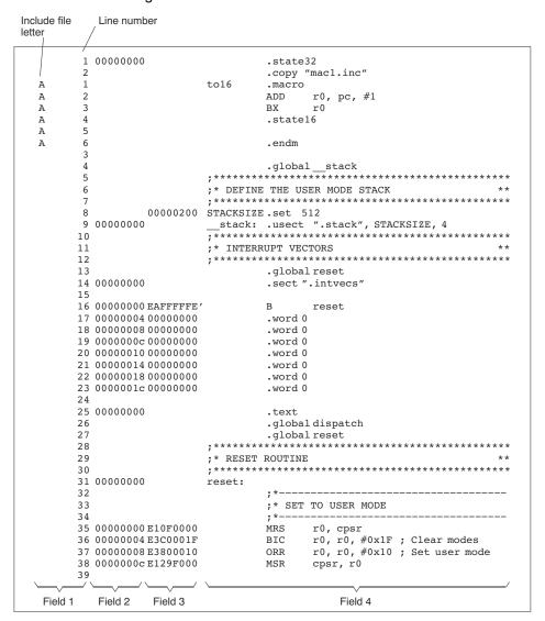
Figure 4-2. Example Assembler Listing
