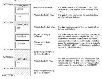
Figure 8-2. Section Placement Defined by the SECTIONS Directive Example
