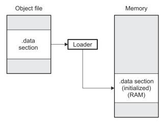
Figure 3-4. Initialization at Load Time
