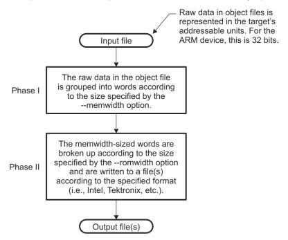
Figure 12-2. Hex Conversion Utility Process Flow
