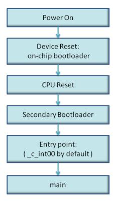
Figure 3-2. Bootloading Sequence with Secondary Bootloader
