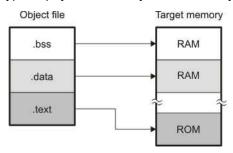
Figure 2-1. Partitioning Memory Into Logical Blocks
