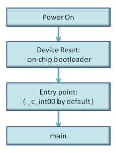
Figure 3-1. Bootloading Sequence (Simplified)
