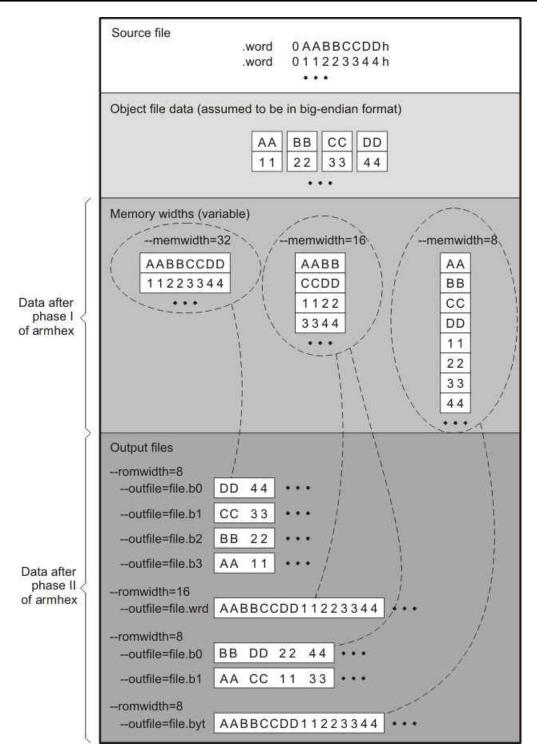
Figure 12-4. Data, Memory, and ROM Widths
