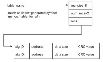
Figure 8-7. CRC\_TABLE Conceptual Model
