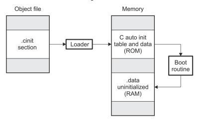
Figure 3-3. Autoinitialization at Run Time
