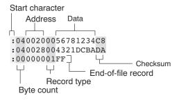
Figure C-6. Contents of Hex Output File lower16.bit
