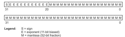
Figure 5-5. Double-Precision Floating-Point Format
