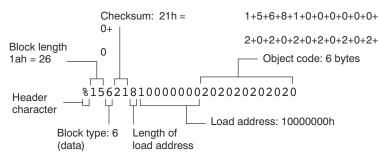
Figure 12-11. Extended Tektronix Object Format
