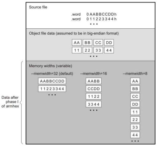
Figure 12-3. Object File Data and Memory Widths
