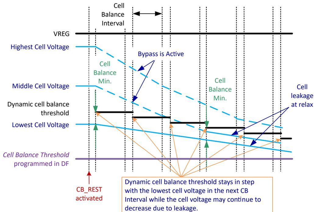
**Figure 3-1. Cell Balancing at Rest Operation**
