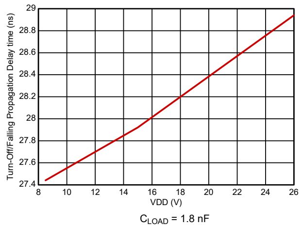
Figure 5-20. Input to Output Falling (Turnoff) Propagation Delay
