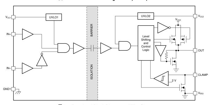
図 8-4. Functional Block Diagram — Miller Clamp
