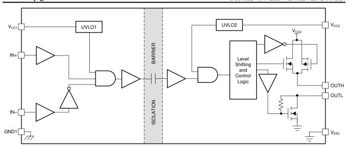
図 8-3. Functional Block Diagram — Split Output
