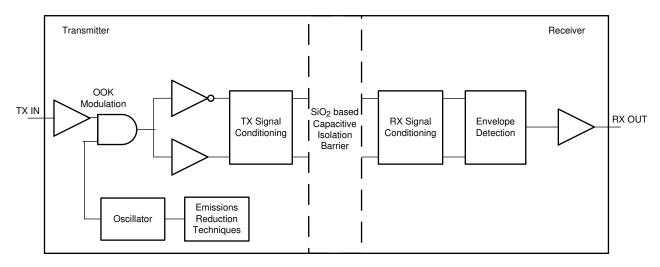
図 8-1. Conceptual Block Diagram of a Capacitive Data Channel
