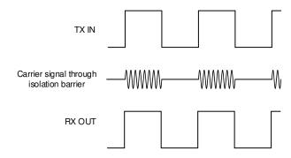
図 8-2. On-Off Keying (OOK) Based Modulation Scheme
