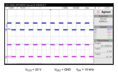
図 9-5. PWM Input and Gate Voltage Waveform
