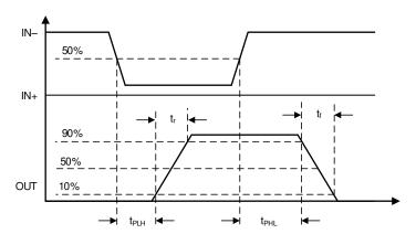
図 7-2. Propagation Delay, Inverting Configuration
