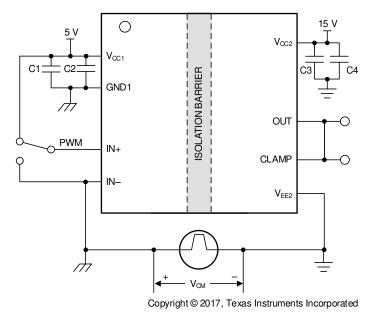
図 7-4. CMTI Test Circuit for Miller Clamp (UCC5350MC)
