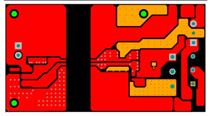
図 11-2. Top-Layer Traces and Copper
