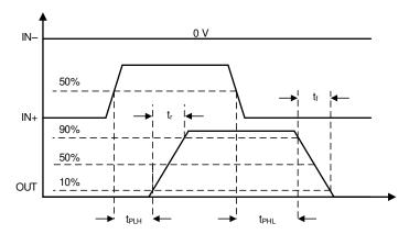
図 7-1. Propagation Delay, Noninverting Configuration
