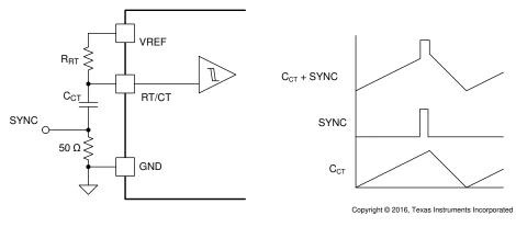
図 8-5. Oscillator Synchronization Circuit
