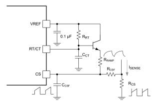
**図** 8-8. Slope Compensation Circuit
