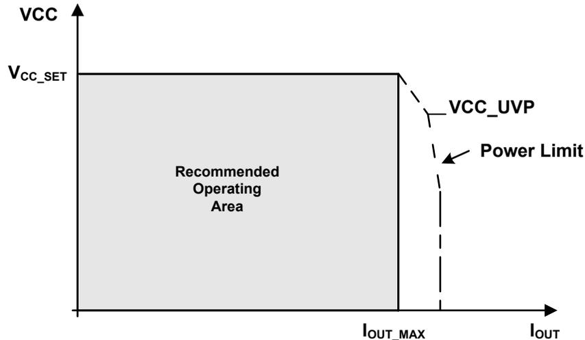
Figure 7-7. VCC Load Recommended Operating Area Description
