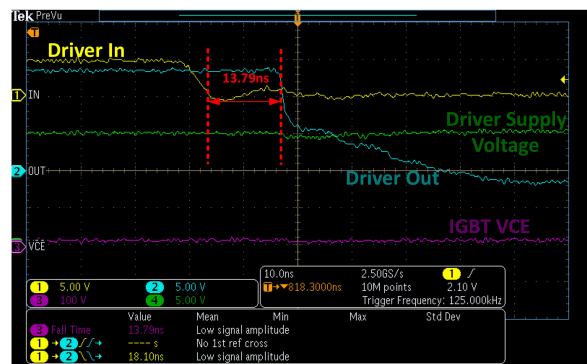
図 7-3. UCC27624-Q1 Used to Drive IGBT in the Boost Converter
