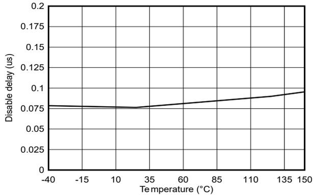
$V_{DD} = V_{HB} = 12V$
