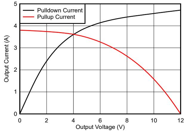
$V_{DD} = V_{HB} = 12V$
