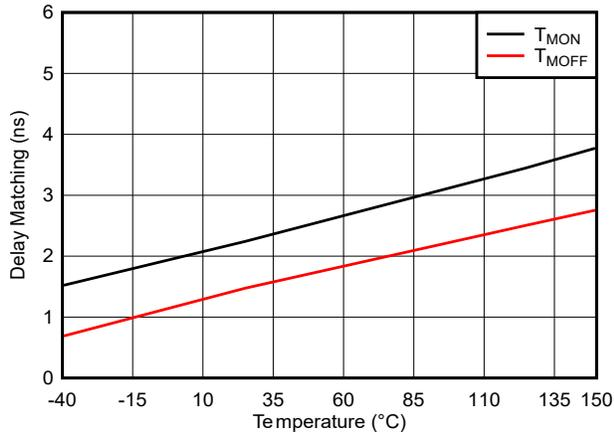
$V_{DD} = V_{HB} = 12V$
