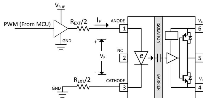
$$R_{EXT} = \frac{V_{SUP} - V_F}{I_F} - R_{OH\_buf}$$
