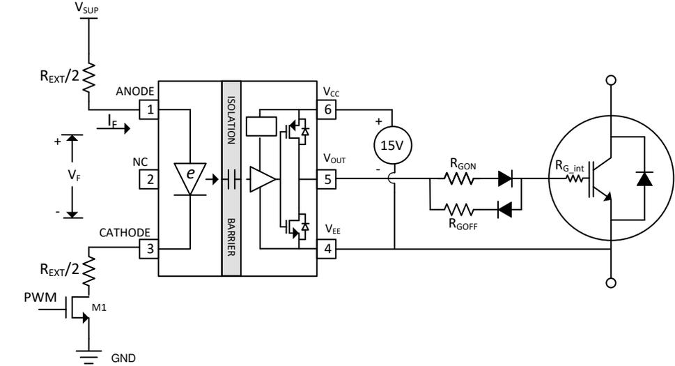
, shows a typical application for driving IGBTs.
