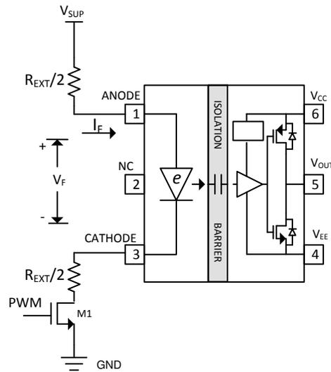
$$R_{EXT} = \frac{V_{SUP} - V_F}{I_F} - R_{M1}$$
