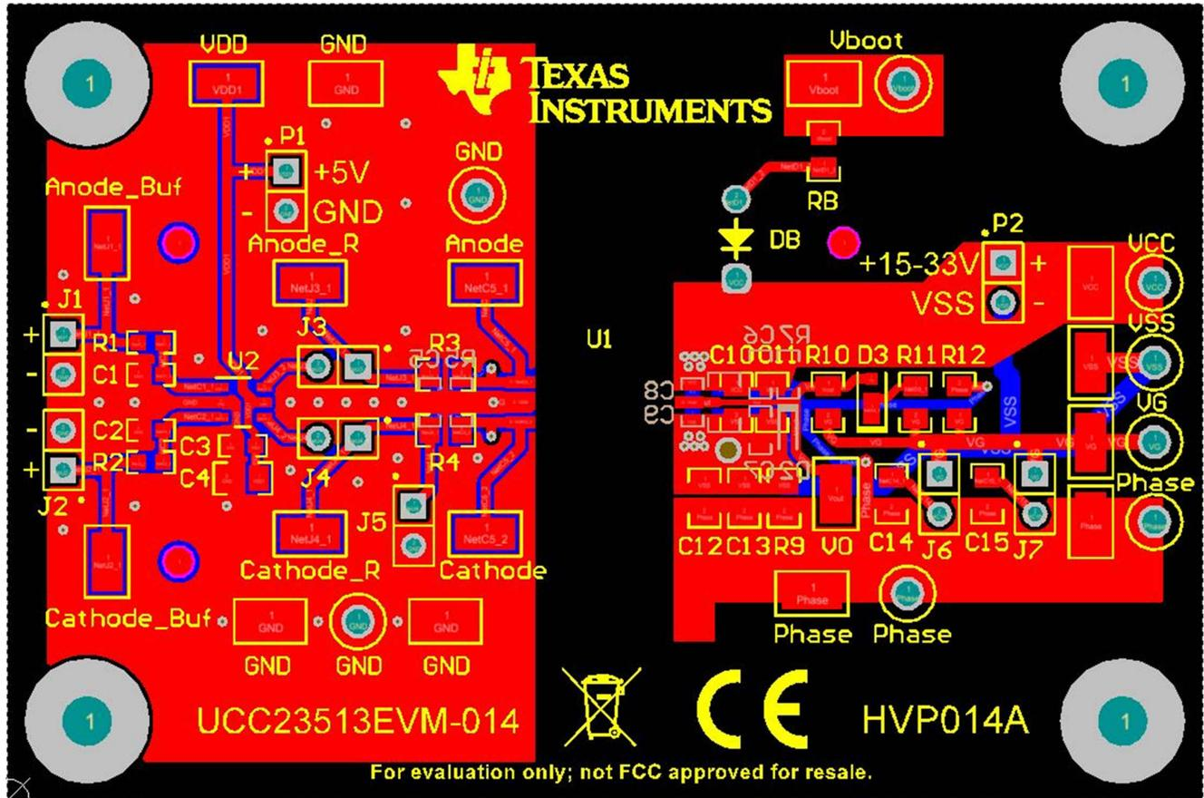
A. No PCB traces or copper are located between the primary and secondary side, which ensures isolation performance.
