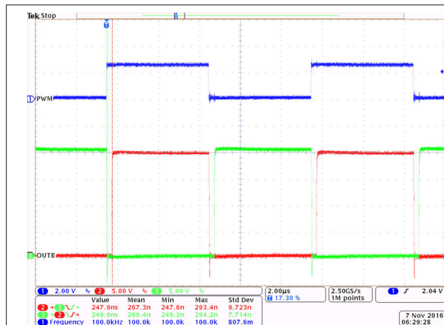
Figure 9-5. Bench Test Waveform for PWM and OUTA/B
