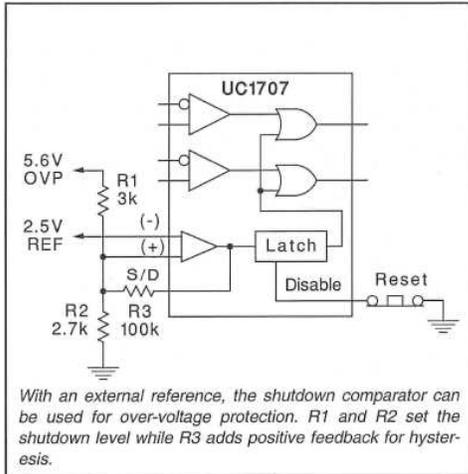
Figure 7. Over-Voltage Protection
