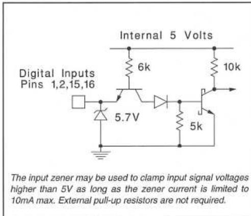
Figure 2. Typical Digital Input Gate
