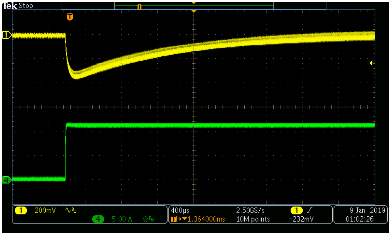
Figure 14. Load Step Up With 40 V IN
