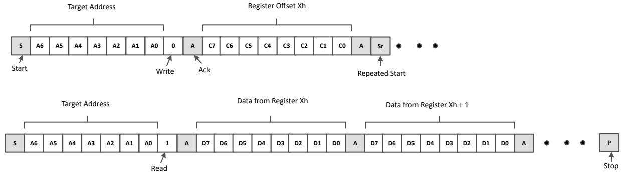
図 7-4. I2C Read with Repeated Start
