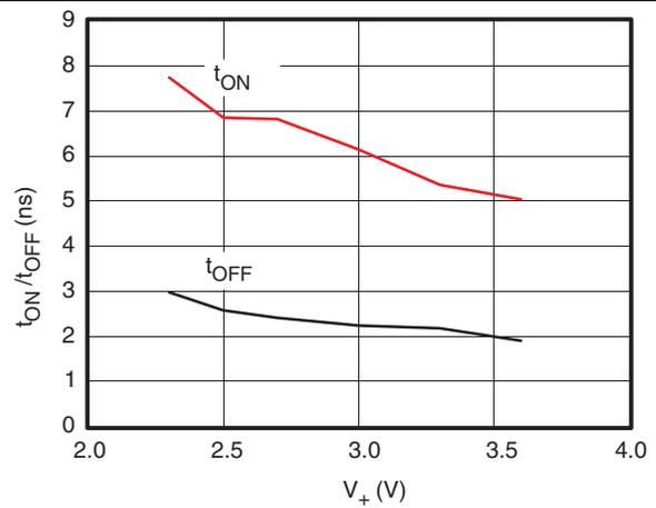
图 6.  $t_{ON}$  and  $t_{OFF}$  vs Supply Voltage
