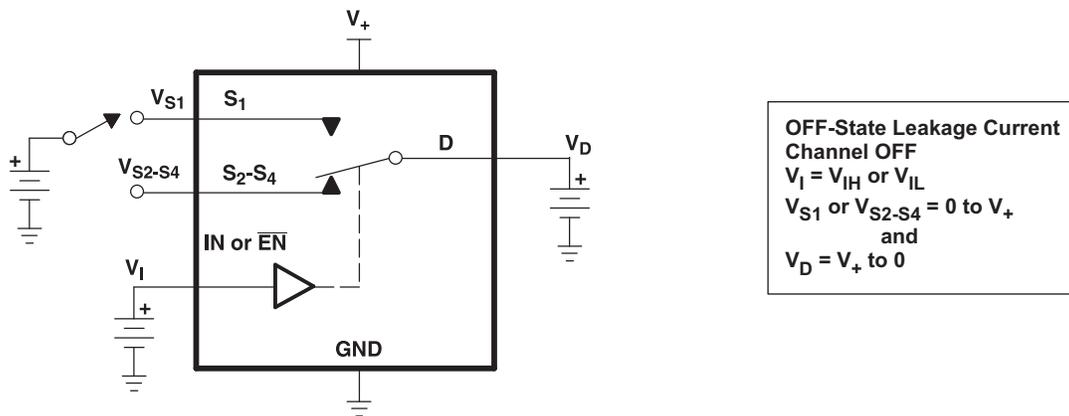
图 13. OFF-State Leakage Current ( $I_{D(OFF)}$ ,  $I_{S(OFF)}$ )
