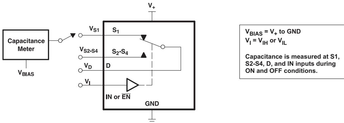
⊠ 15. Capacitance ( $C_I$ ,  $C_{D(OFF)}$ ,  $C_{D(ON)}$ ,  $C_{S(OFF)}$ ,  $C_{S(ON)}$ )
