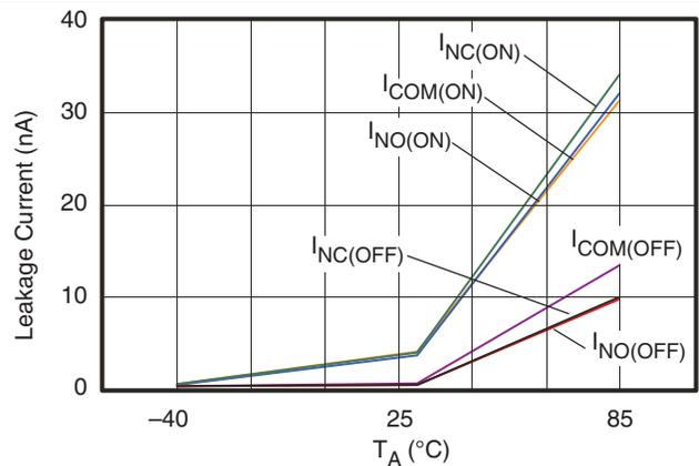
图 4. Leakage Current vs Temperature ( $V_+ = 3.6$  V)
