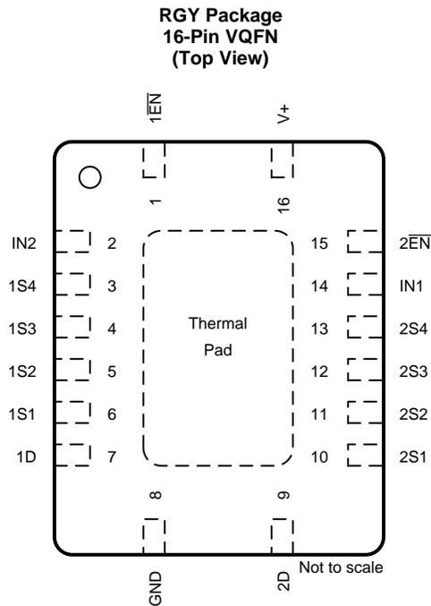
If exposed thermal pad is used, it must be connected as a secondary ground or left electrically open.
