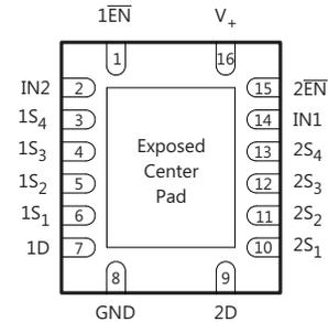
If exposed center pad is used, it must be connected as a secondary ground or left electrically open.
