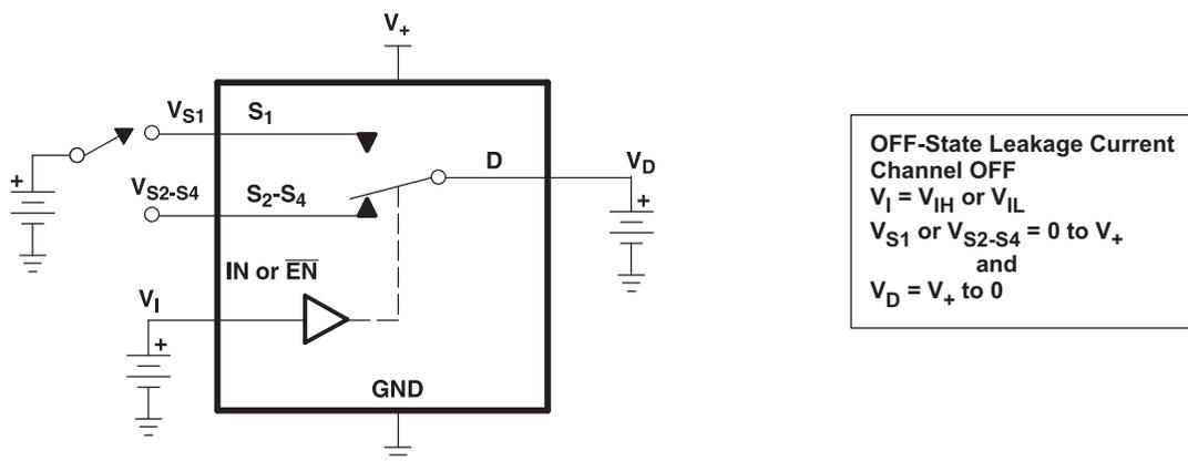
Figure 13. OFF-State Leakage Current ( $I_{D(OFF)}$ ,  $I_{S(OFF)}$ )
