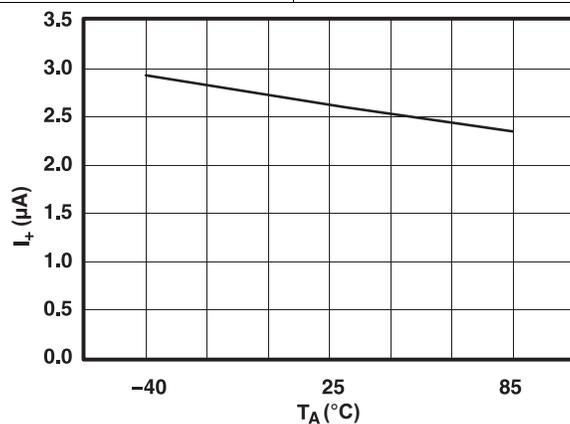
Figure 11. Power-Supply Current vs Temperature (V<sub>+</sub> = 3.6 V)
