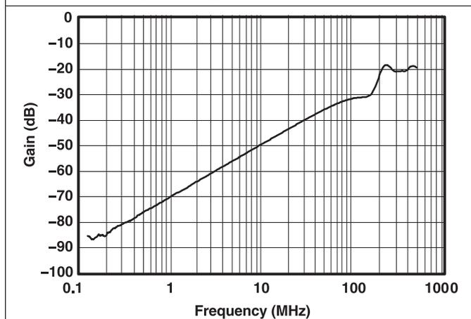
Figure 9. OFF Isolation and Crosstalk vs Frequency (V<sub>+</sub> = 3.3 V)
