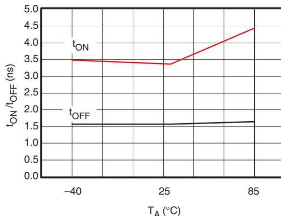
Figure 25. t<sub>ON</sub> and t<sub>OFF</sub> vs Temperature (V<sub>+</sub> = 3.3 V)
