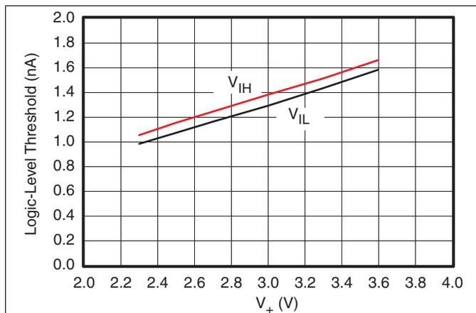
Figure 7. Logic-Level Threshold vs V<sub>+</sub>
