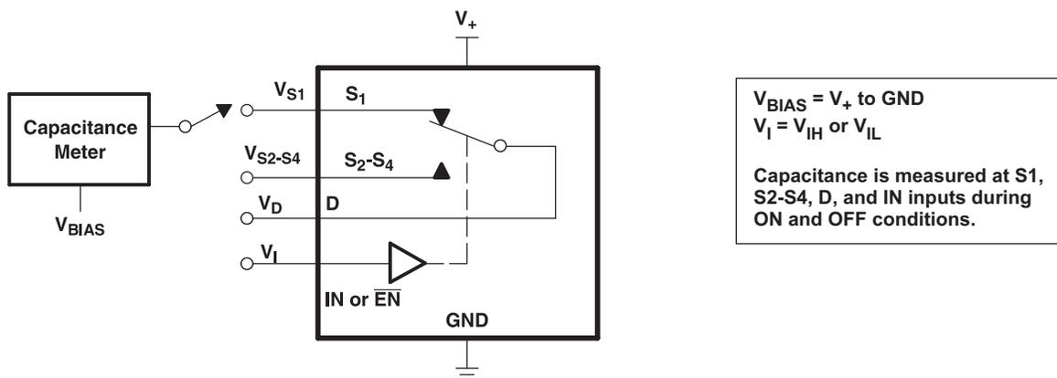
Figure 15. Capacitance ( $C_I$ ,  $C_{D(OFF)}$ ,  $C_{D(ON)}$ ,  $C_{S(OFF)}$ ,  $C_{S(ON)}$ )
