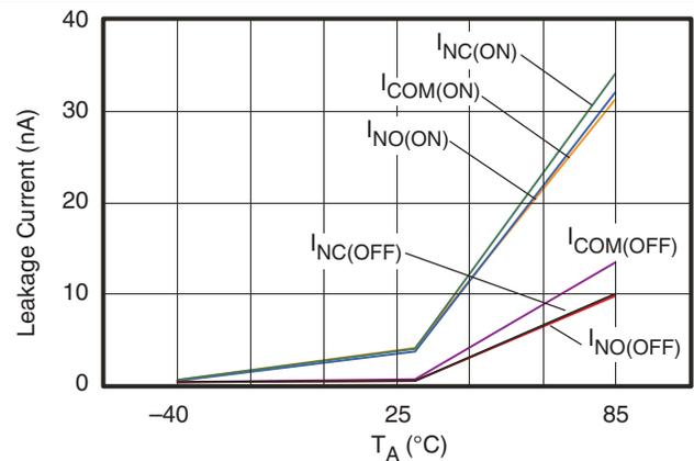
Figure 4. Leakage Current vs Temperature ( $V_+ = 3.6$  V)
