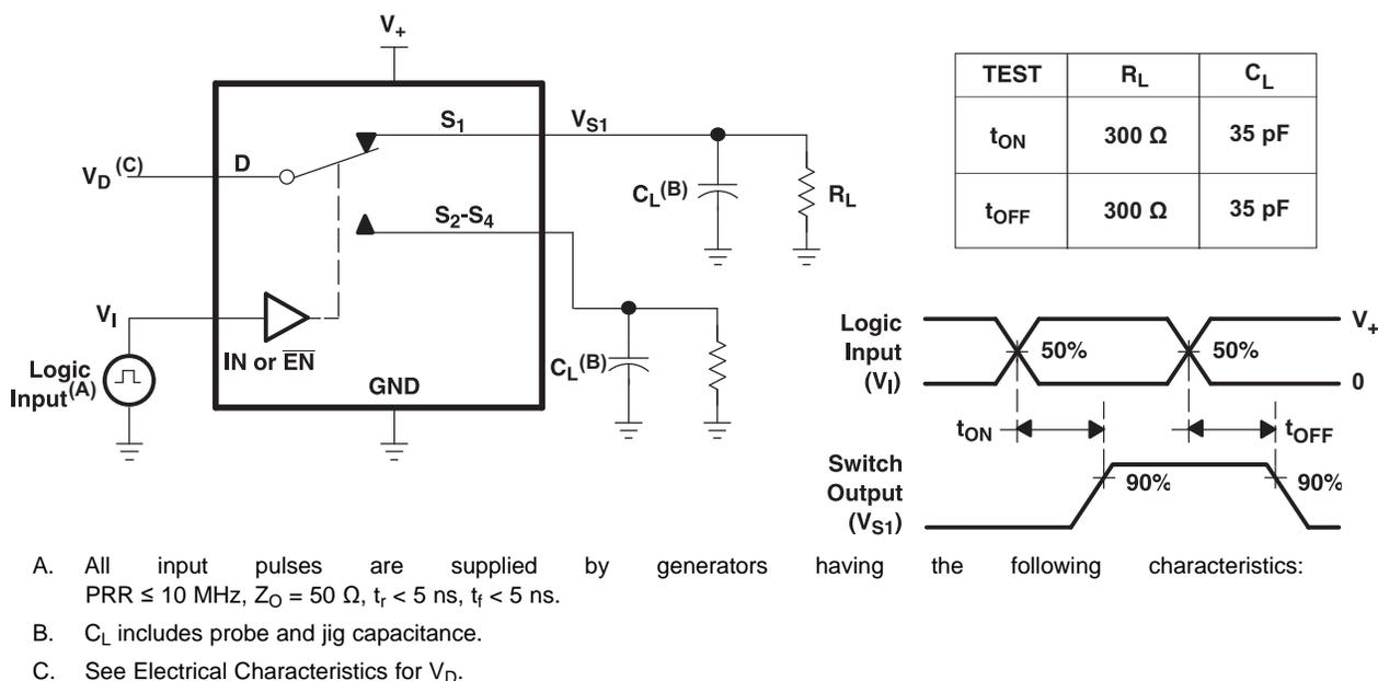
Figure 16. Turnon ( $t_{ON}$ ) and Turnoff Time ( $t_{OFF}$ )
