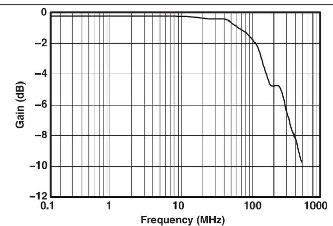
Figure 8. Bandwidth (Gain vs Frequency) (V<sub>+</sub> = 3.3 V)
