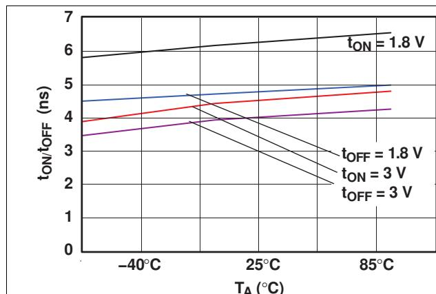
**Figure 12.**  $t_{ON}$  and  $t_{OFF}$  vs Temperature
