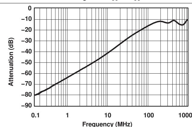
**Figure 15.** OFF Isolation vs Frequency
