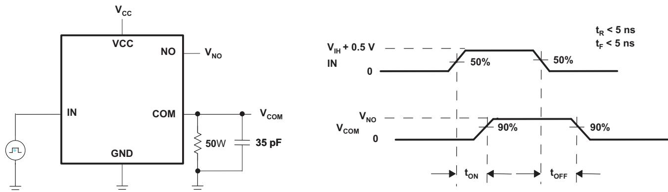
Figure 1. Switching Times
