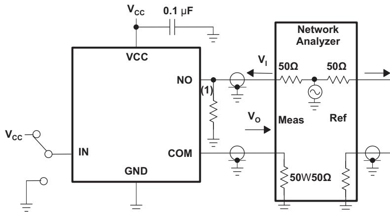
Measurements are standardized against short at socket terminals. OFF isolation is measured between COM and OFF terminals on each switch. Bandwidth is measured between COM and ON terminals on each switch. Signal direction through switch is reversed; worst values are recorded.
