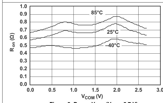
Figure 8.  $R_{on}$  vs  $V_{COM}$  ( $V_{CC} = 2.7\text{ V}$ )
