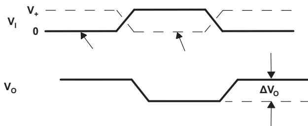
**Figure 5. Charge Injection ( $Q_C$ )**
