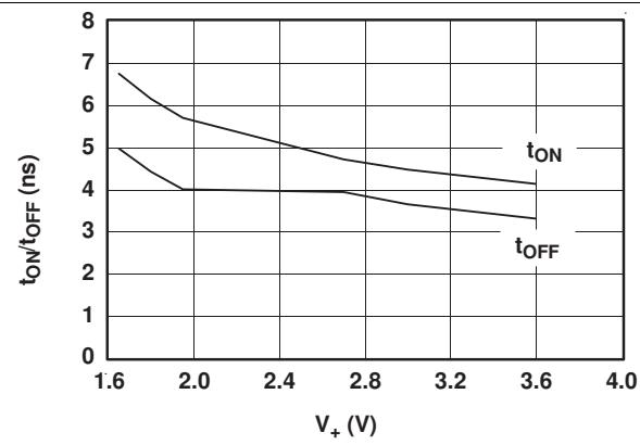
Figure 11.  $t_{ON}$  and  $t_{OFF}$  vs Supply Voltage
