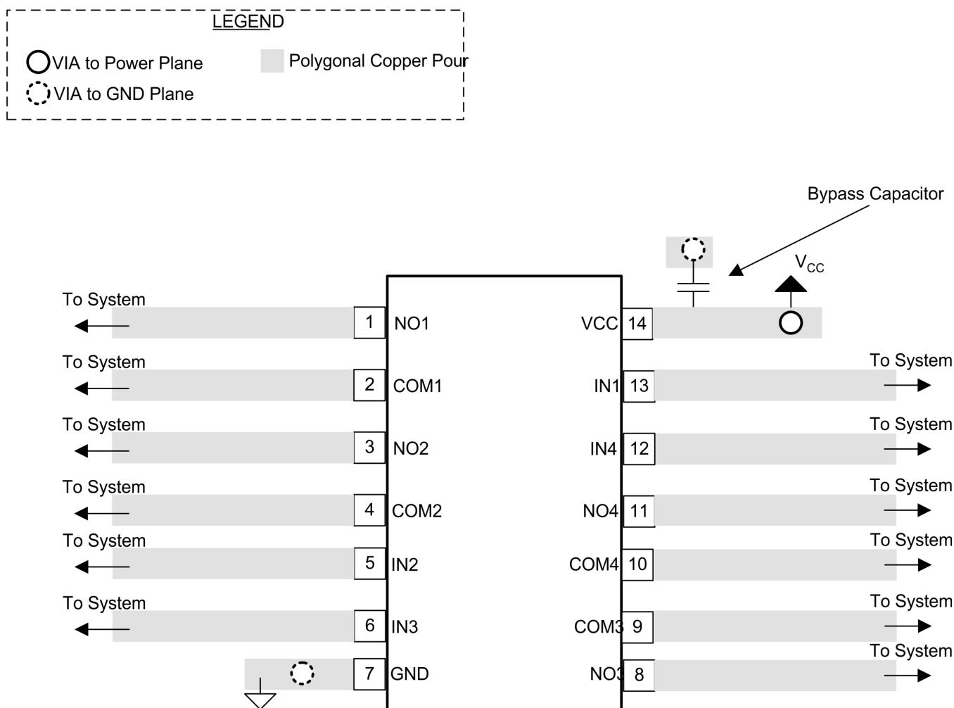
**Figure 21. Layout Schematic**
