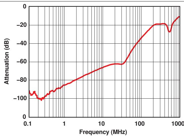
Figure 18. Crosstalk vs Frequency ( $V_{CC} = 3$  V)
