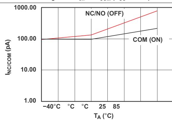
Figure 9.  $I_{ON}$  and  $I_{OFF}$  vs Temperature
