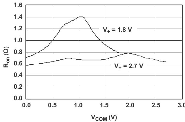
**Figure 20.**  $R_{on}$  vs  $V_{COM}$
