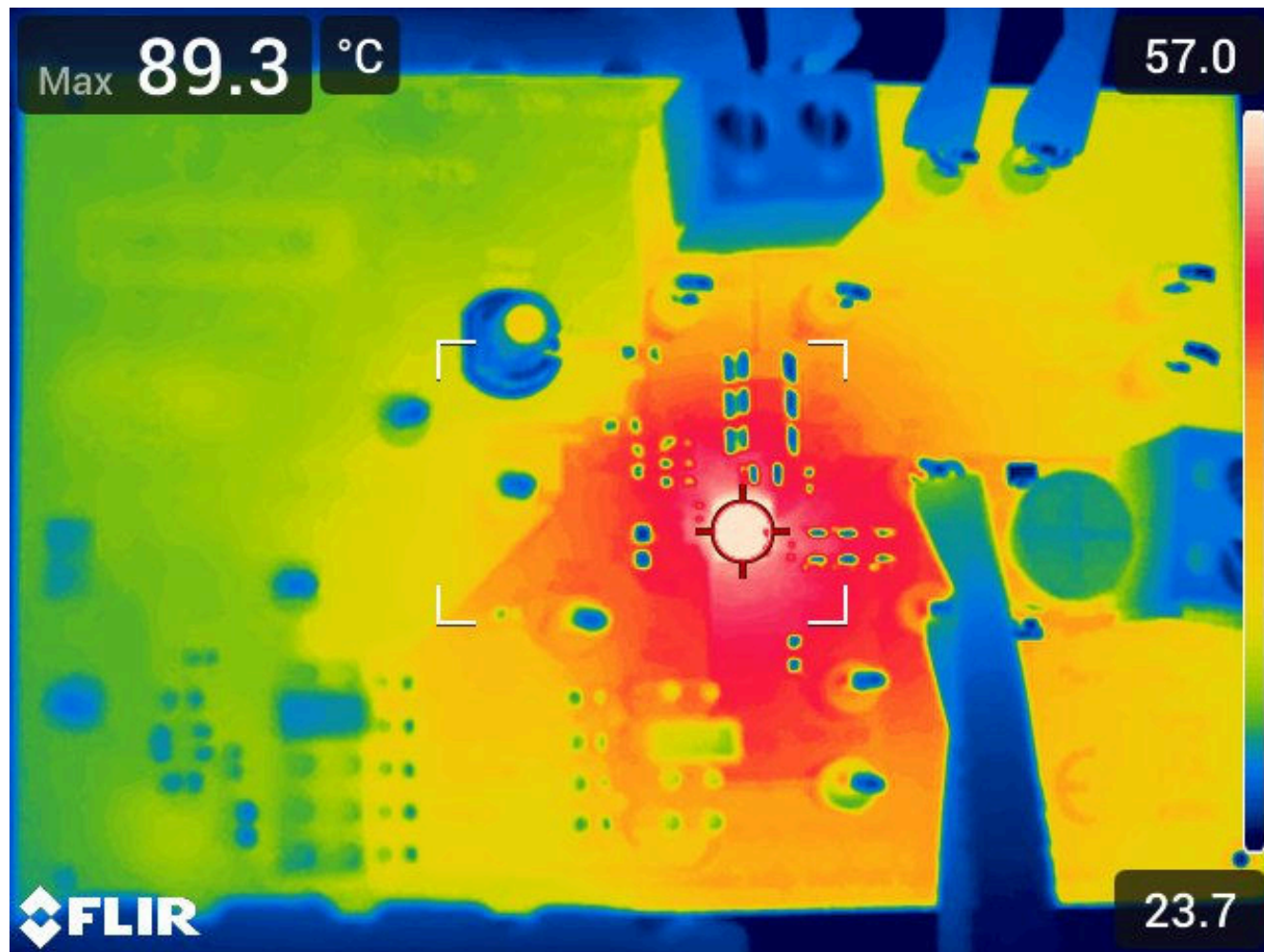
図 7-20. Thermal Image at 25^{\circ}\text{C} Ambient
