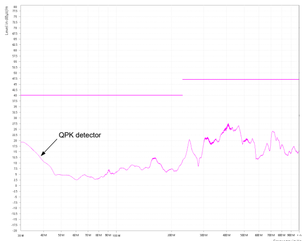
Figure 9-11. CISPR 32 Class B Radiated Emissions: Vertical Polarization
