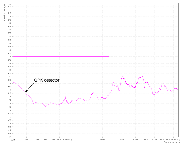
Figure 9-10. CISPR 32 Class B Radiated Emissions: Horizontal Polarization
