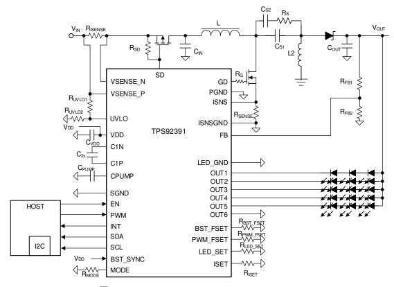
図 8-7. SEPIC Mode with Three LEDs in Series
