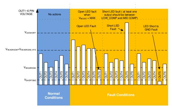
図 7-18. LED Open and Short Detection Logic
