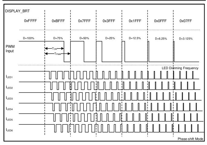
図 7-10. Phase-shift Dimming Diagram
