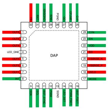
図 5-1. RHB Package 32-PIN QFN Top View
