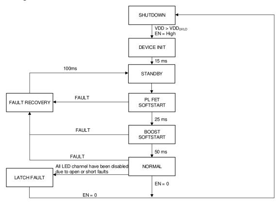
図 7-19. State Machine Diagram
