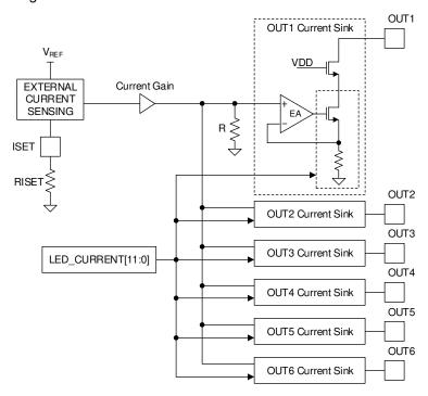
図 7-8. LED Driver Current Setting Circuit
