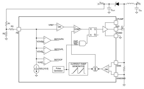
図 7-6. Three-Resistor FB Divider Circuit
