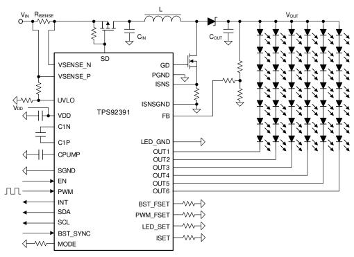
図 8-1. Full Feature Application for Display Backlight
