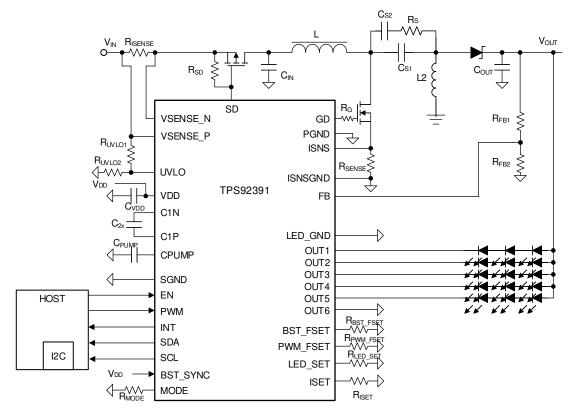
図 8-6. SEPIC Mode with Three LEDs in Series
