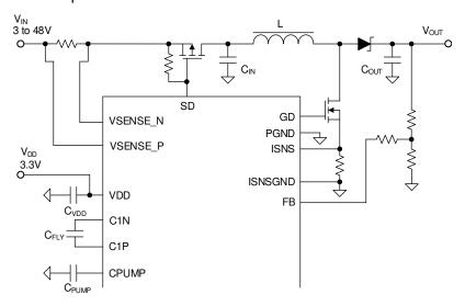
図 7-1. Charge Pump Enabled Circuit
