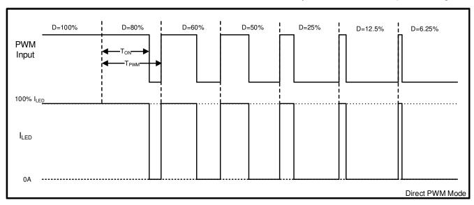
図 7-12. Direct PWM Dimming Diagram
