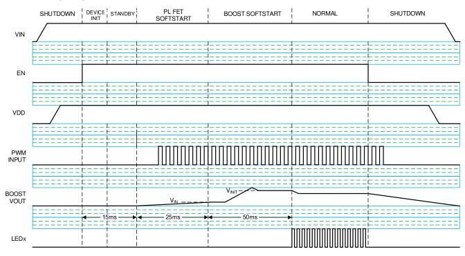
図 7-20. Start-Up Sequence Diagram
