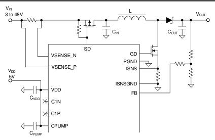
図 7-2. Charge Pump Disabled Circuit
