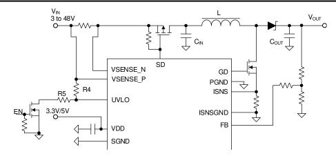
図 7-17. VIN UVLO Setting Circuit Without Current Leakage Path
