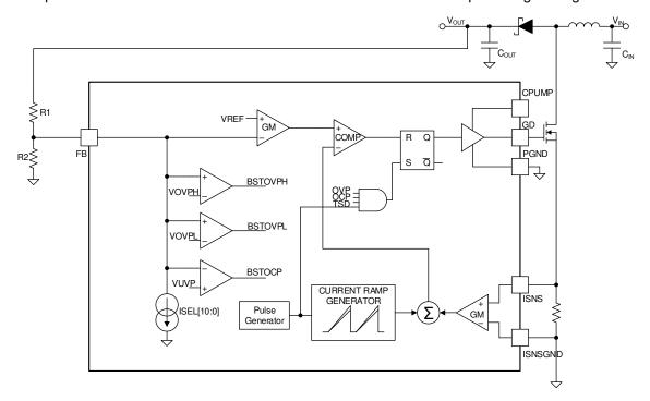
図 7-5. Two-Resistor FB Divider Circuit
