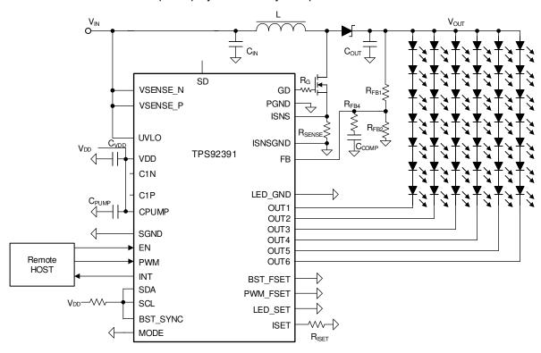
図 8-5. Minimal Solution/Minimum Components Application
