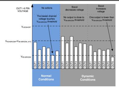
図 7-4. Adaptive Boost Voltage Control Loop Function
