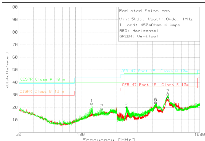
Figure 36. Radiated Emissions 5-V Input, 1.8-V Output, 4-A Load (EN55022 Class B)
