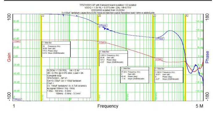
図 8-7. Bode Plot for a Typical DDR3 Configuration
