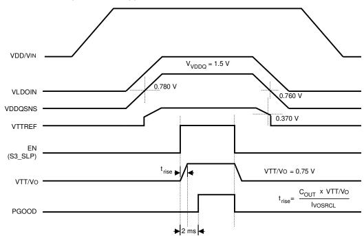
図 8-3. Typical Timing Diagram for S3 and Pseudo-S5 Support
