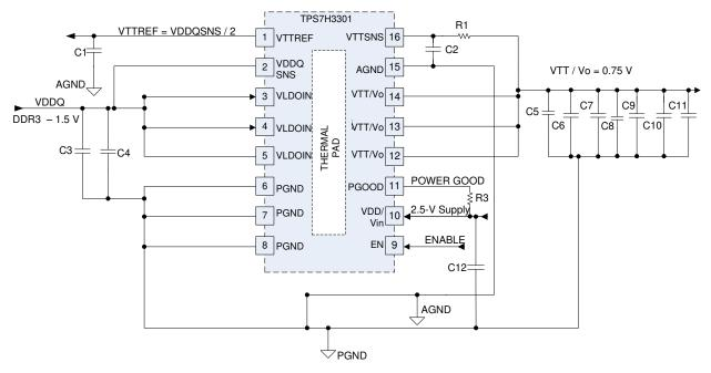
図 8-1. Typical Application Circuit
