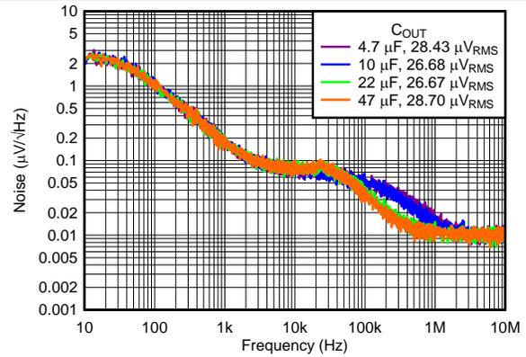
$V_{OUTN} = -5\text{ V}$ ,  $I_{OUTN} = -150\text{ mA}$ ,  $V_{INP} = V_{EN} = 6\text{ V}$ ,  $V_{OUTN} = -5\text{ V}$ ,  $I_{OUTP} = 0\text{ mA}$ ,  $C_{NR/SS} = C_{FFX} = 10\text{ nF}$
