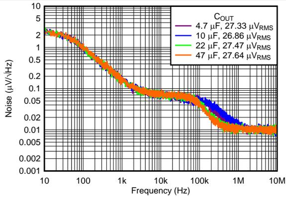
$V_{OUTP} = 5\text{ V}$ ,  $I_{OUTP} = 150\text{ mA}$ ,  $V_{INP} = V_{EN} = 6\text{ V}$ ,  $V_{OUTN} = -5\text{ V}$ ,  $I_{OUTN} = 0\text{ mA}$ ,  $C_{NR/SS} = C_{FFX} = 10\text{ nF}$
