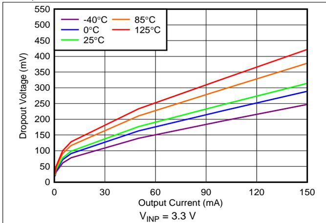
图 50. Positive Regulator Dropout Voltage vs Output Current
