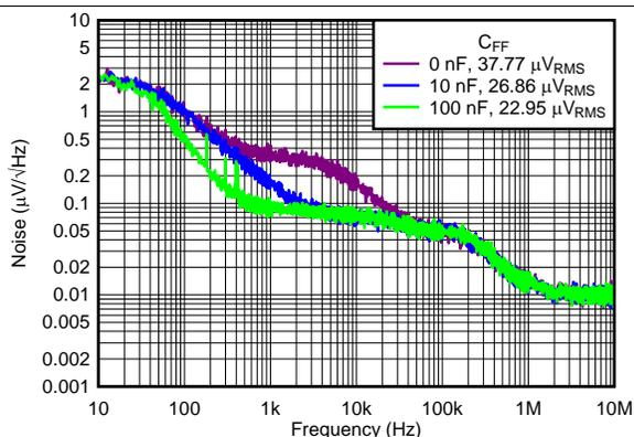
$V_{OUTP} = 5\text{ V}$ ,  $I_{OUTP} = 150\text{ mA}$ ,  $V_{INP} = V_{EN} = 6\text{ V}$ ,  $V_{OUTN} = -5\text{ V}$ ,  $I_{OUTN} = 0\text{ mA}$ ,  $C_{NR/SS} = 10\text{ nF}$
