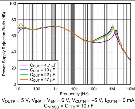
Figure 6. Positive PSRR vs Frequency and  $C_{OUTP}$
