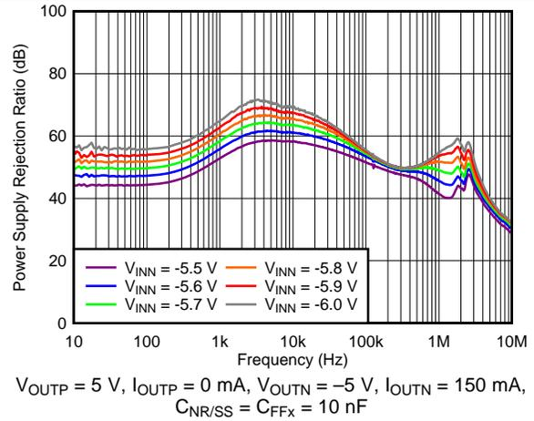
Figure 3. Negative PSRR vs Frequency and  $V_{INN}$
