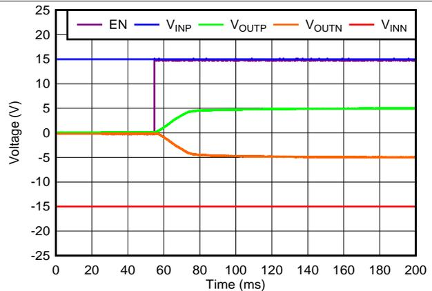
$V_{OUTP} = -V_{OUTN} = 5\text{ V}$ ,  $V_{INP} = -V_{INN} = 15\text{ V}$
