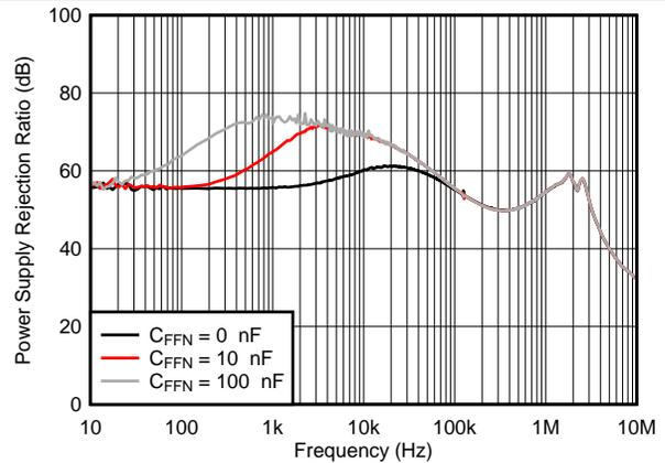
$V_{OUTP} = 5\text{ V}$ ,  $I_{OUTP} = 0\text{ mA}$ ,  $V_{INN} = -6\text{ V}$ ,  $V_{OUTN} = -5\text{ V}$ ,  $C_{NR/SS} = C_{FFN} = 10\text{ nF}$
