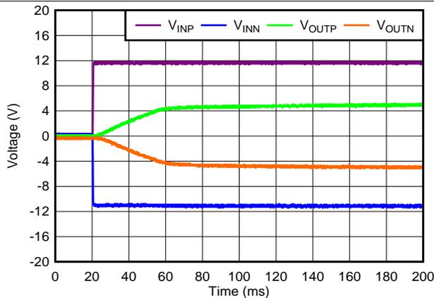
$V_{OUTP} = -V_{OUTN} = 5\text{ V}$ ,  $V_{INP} = -V_{INN} = 12\text{ V}$
