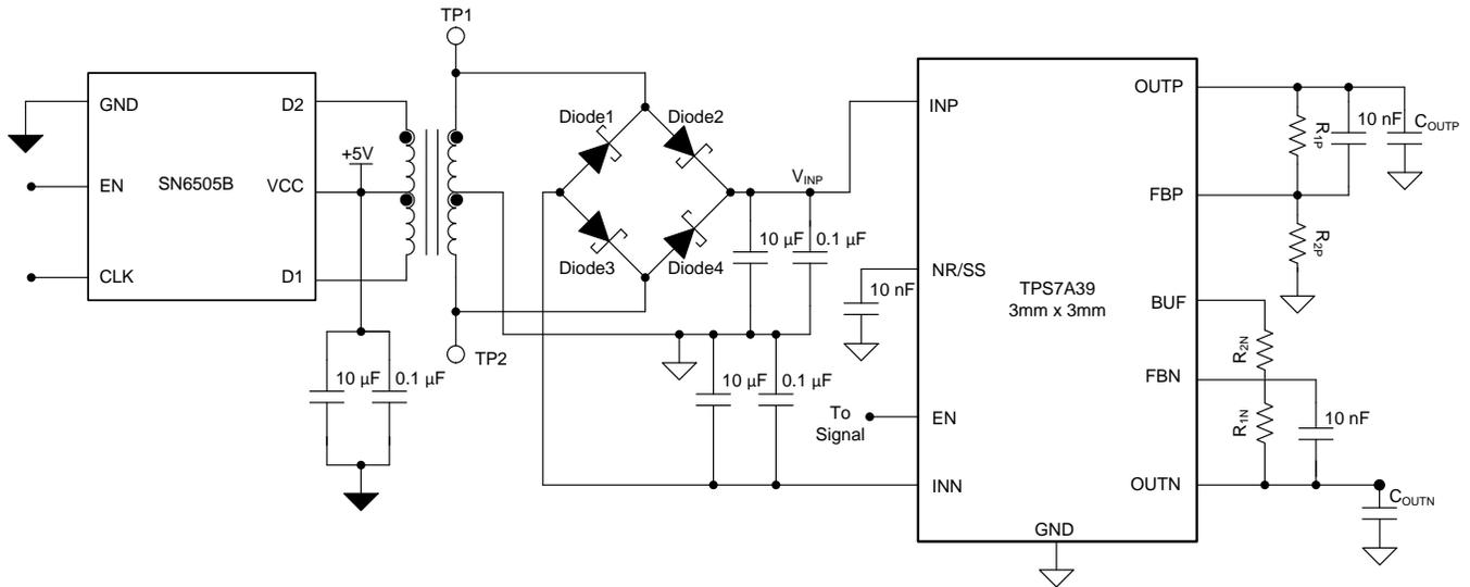
图 71. Single-Ended to Differential Isolated Supply Schematic
