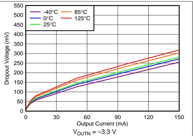
图 51. Negative Regulator Dropout Voltage vs Output Current
