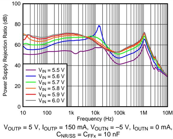
Figure 2. Positive PSRR vs Frequency and  $V_{INP}$
