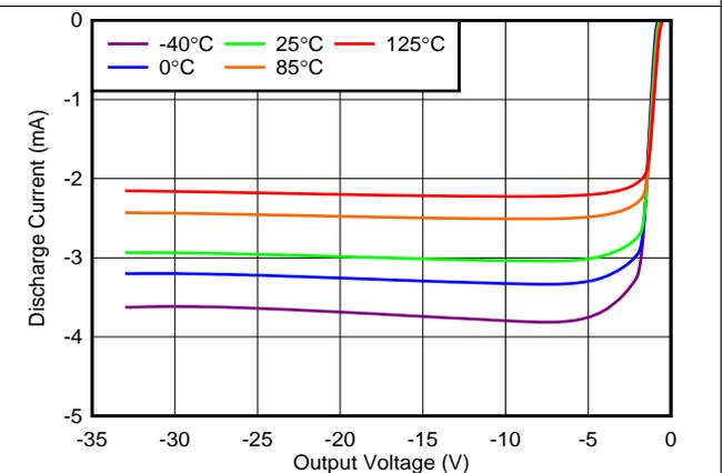
图 55. Negative Output Discharge Current vs Output Voltage
