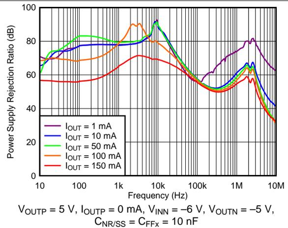
Figure 5. Negative PSRR vs Frequency and  $I_{OUTN}$
