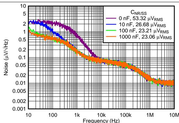
$V_{OUTN} = -5\text{ V}$ ,  $I_{OUTN} = -150\text{ mA}$ ,  $V_{INP} = V_{EN} = 6\text{ V}$ ,  $V_{OUTN} = -5\text{ V}$ ,  $I_{OUTP} = 0\text{ mA}$ ,  $C_{FFX} = 10\text{ nF}$
