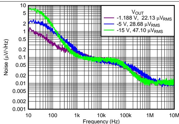
$I_{OUTN} = -150\text{ mA}$ ,  $V_{INP} = V_{EN}$ ,  $V_{OUTN} = -V_{OUTP}$ ,  $I_{OUTP} = 0\text{ mA}$ ,  $C_{NR/SS} = C_{FFX} = 10\text{ nF}$
