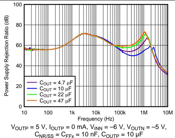
Figure 7. Negative PSRR vs Frequency and  $C_{OUTN}$
