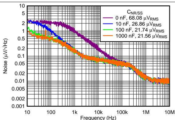
$V_{OUTP} = 5\text{ V}$ ,  $I_{OUTP} = 150\text{ mA}$ ,  $V_{INP} = V_{EN} = 6\text{ V}$ ,  $V_{OUTN} = -5\text{ V}$ ,  $I_{OUTN} = 0\text{ mA}$ ,  $C_{FFX} = 10\text{ nF}$
