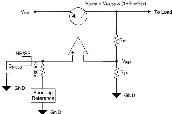
, and in normal regulation  $V_{FBP} = V_{NR/SS}$ . Sharing a single reference ensures that both channels track each other during start-up.
