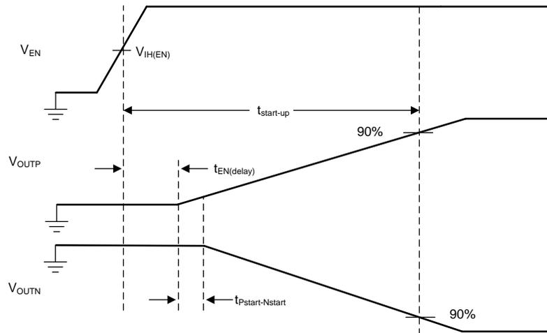
NOTE: Slow ramps ( $t_{rise(V_{INx})} > 10$  ms typically) on  $V_{INx}$  with EN tied to  $V_{INP}$  does not meet the tracking specification. Use a resistor divider from  $V_{INP}$  to EN for these applications.
