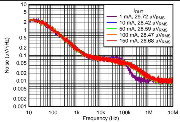
$V_{OUTN} = -5\text{ V}$ ,  $V_{INP} = V_{EN} = 6\text{ V}$ ,  $V_{OUTN} = -5\text{ V}$ ,  $I_{OUTP} = 0\text{ mA}$ ,  $C_{NR/SS} = C_{FFX} = 10\text{ nF}$
