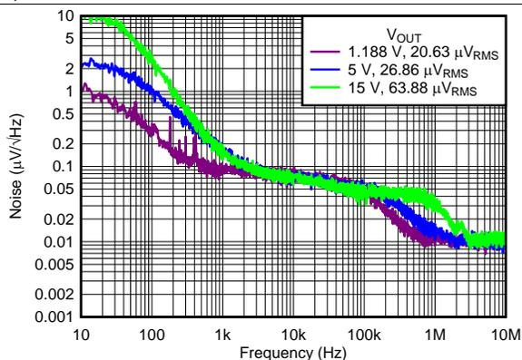
$I_{OUTP} = 150\text{ mA}$ ,  $V_{INP} = V_{EN}$ ,  $V_{OUTN} = -V_{OUTP}$ ,  $I_{OUTN} = 0\text{ mA}$ ,  $C_{NR/SS} = C_{FFX} = 10\text{ nF}$
