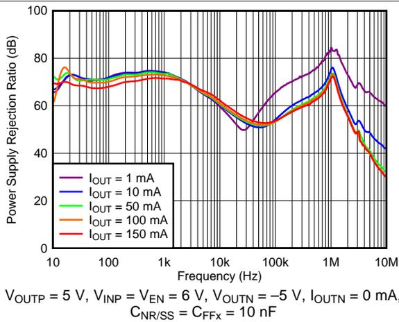
Figure 4. Positive PSRR vs Frequency and  $I_{OUTP}$
