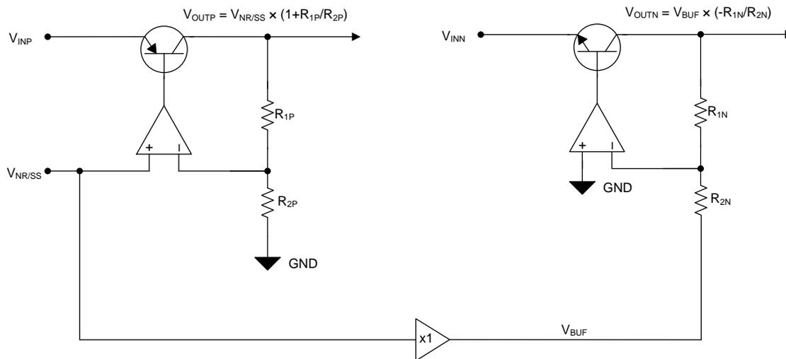
Figure 63. Simplified Regulation Circuit
