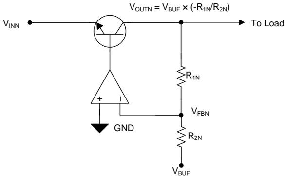
shows, the negative LDO on the device regulates with a  $V_{FBN} = 0\text{ V}$  and inverts the positive reference ( $V_{BUF}$ ). This topology allows the negative regulator to regulate down to 0 V.
