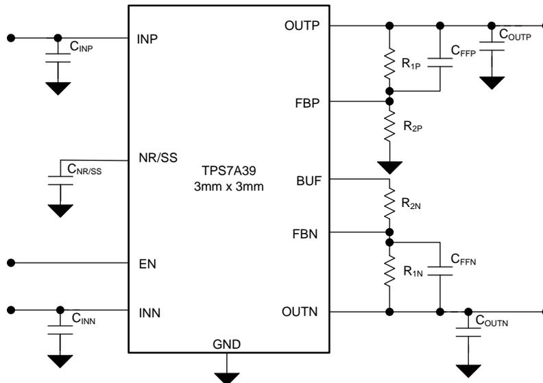
Figure 65. Adjustable Operation
