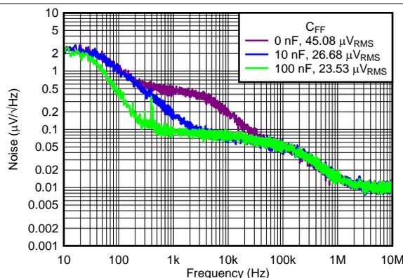
$V_{OUTN} = -5\text{ V}$ ,  $I_{OUTN} = -150\text{ mA}$ ,  $V_{INP} = V_{EN} = 6\text{ V}$ ,  $V_{OUTN} = -5\text{ V}$ ,  $I_{OUTP} = 0\text{ mA}$ ,  $C_{NR/SS} = 10\text{ nF}$
