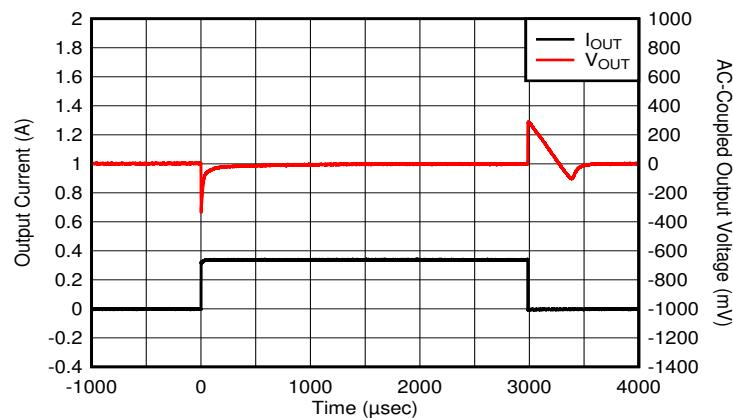
$I_{OUT} = 1 \text{ mA to } 0.33 \text{ A, slew rate} = 0.5 \text{ A}/\mu\text{s},$
