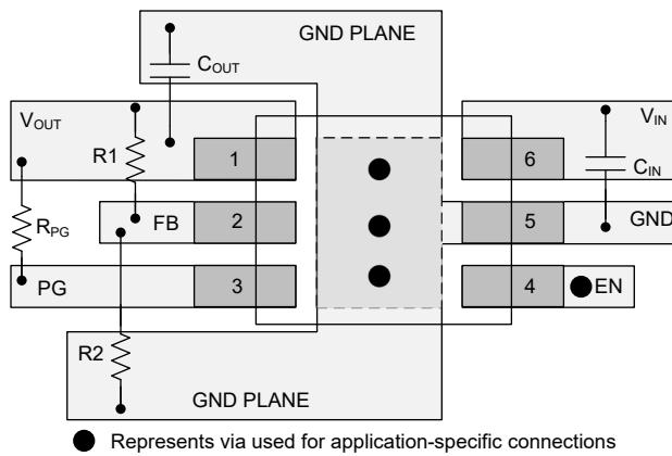
図 42. Adjustable Version Layout Example
