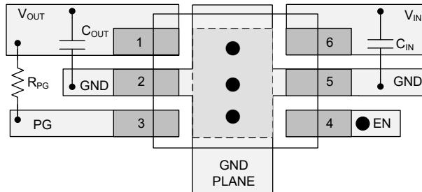
● Represents via used for application-specific connections
