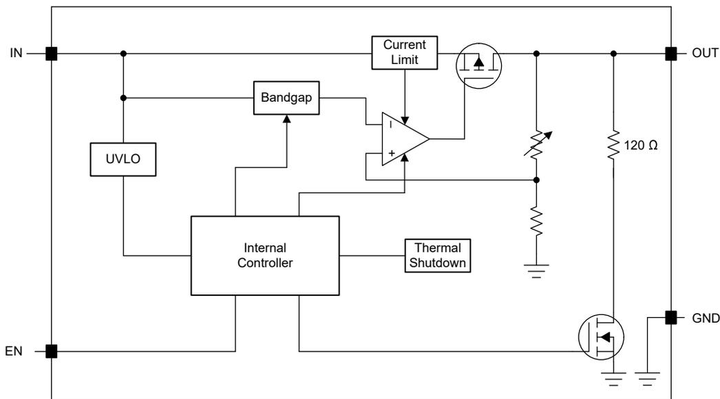
図 6-4. Functional Block Diagram – Fixed Version (New Chip)
