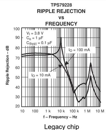
5-24. TPS792 Ripple Rejection vs Frequency
