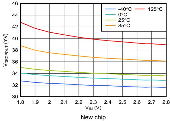
5-19. TPS792 Dropout Voltage vs Input Voltage
