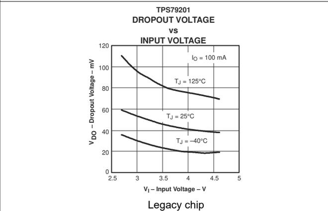
Figure 5-18. TPS792 Dropout Voltage vs Input Voltage
