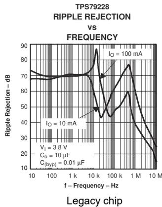
5-21. TPS792 Ripple Rejection vs Frequency
