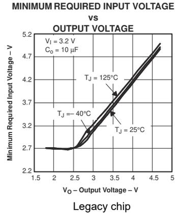
5-20. Minimum Required Input Voltage vs Output Voltage
