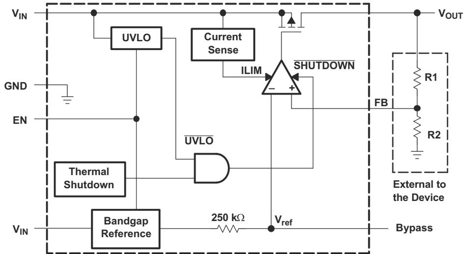
☒ 6-1. Functional Block Diagram – Adjustable Version (Legacy Chip)
