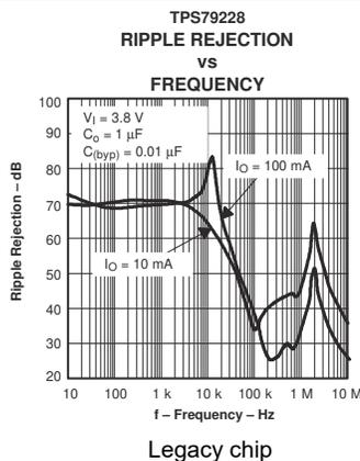
5-23. TPS792 Ripple Rejection vs Frequency
