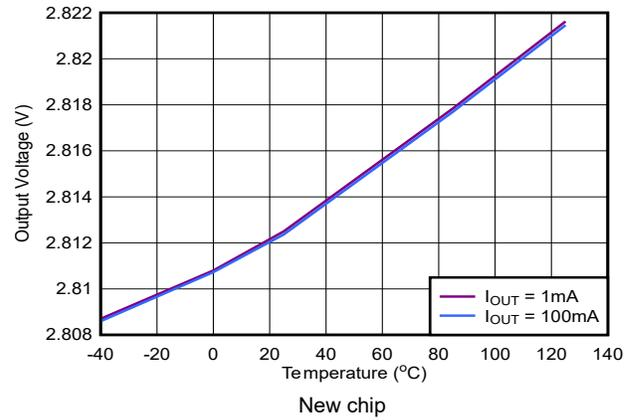
Figure 5-4. TPS792 Output Voltage vs Junction Temperature
