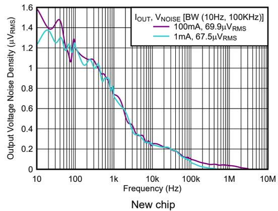
5-10. TPS792 Output Spectral Noise Density vs Frequency
