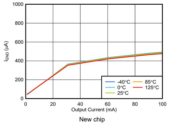
Figure 5-6. TPS792 Ground Current vs  $I_{OUT}$
