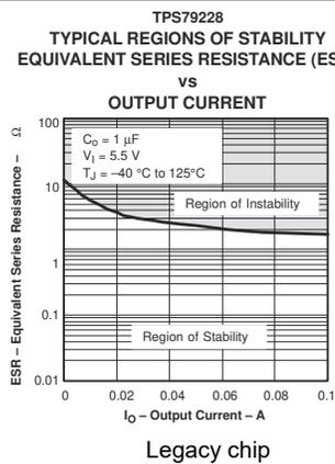
5-33. Typical Regions of Stability Equivalent Series Resistance (ESR) vs Output Current
