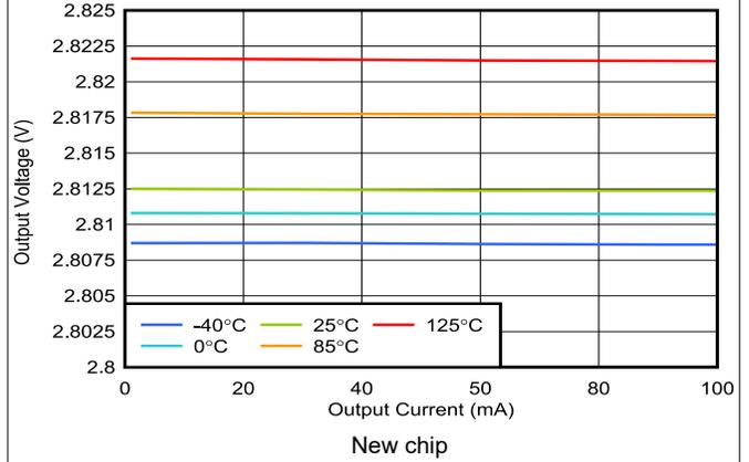
Figure 5-2. TPS792 Output Voltage vs Output Current
