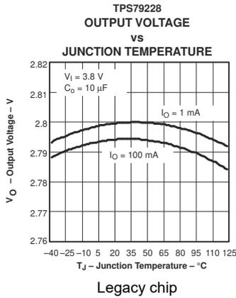
Figure 5-3. TPS792 Output Voltage vs Junction Temperature
