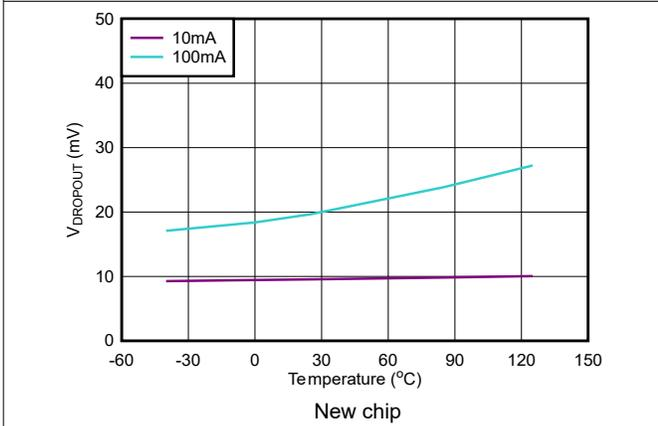
Figure 5-15. TPS792 Dropout Voltage vs Junction Temperature
