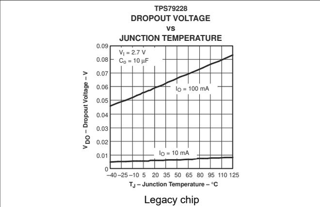
Figure 5-14. TPS792 Dropout Voltage vs Junction Temperature
