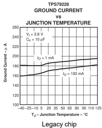
Figure 5-5. TPS792 Ground Current vs Junction Temperature
