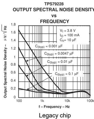
5-9. TPS792 Output Spectral Noise Density vs Frequency
