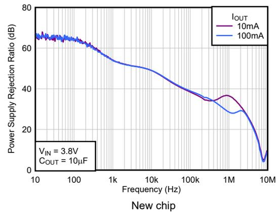
5-22. TPS792 Ripple Rejection vs Frequency
