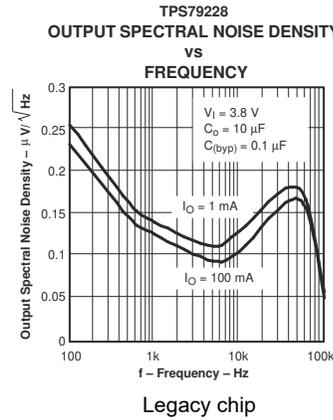
5-8. TPS792 Output Spectral Noise Density vs Frequency
