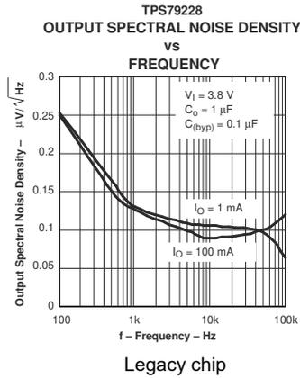
5-7. TPS792 Output Spectral Noise Density vs Frequency
