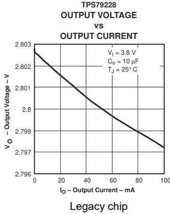
Figure 5-1. TPS792 Output Voltage vs Output Current
