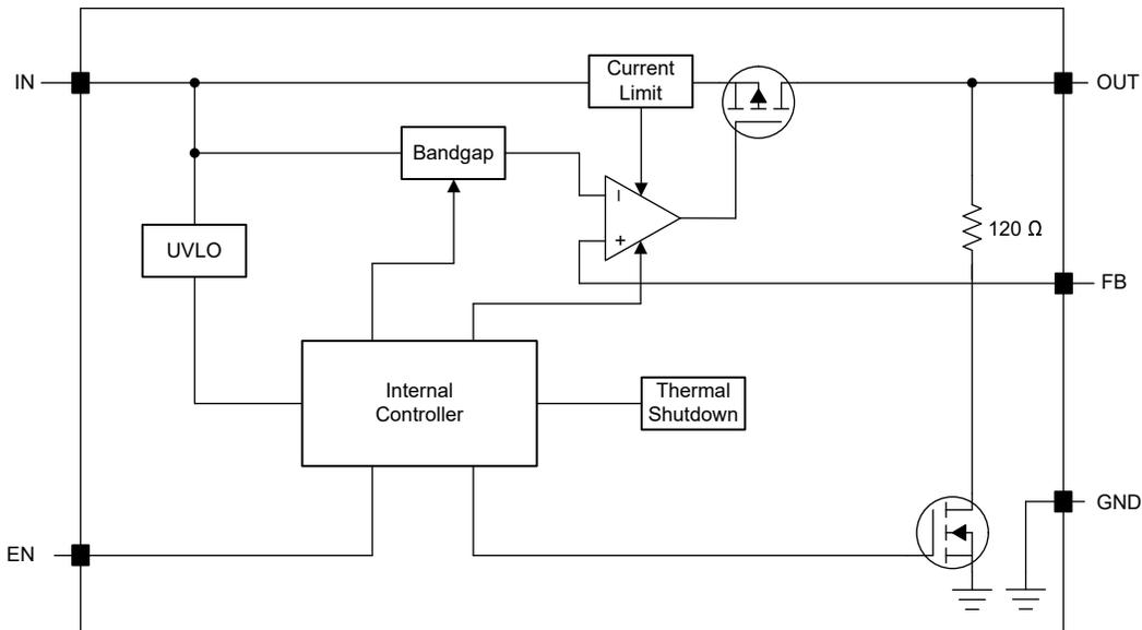
☒ 6-2. Functional Block Diagram – Adjustable Version (New Chip)
