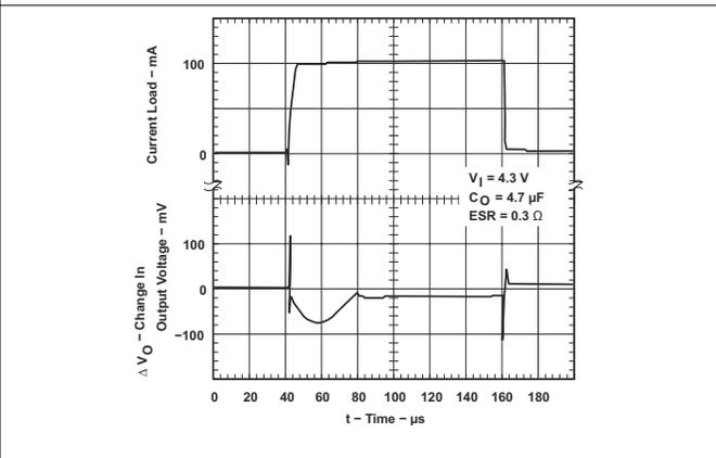
Figure 5-42. TPS76933-Q1 Load Transient Response (Legacy Chip)
