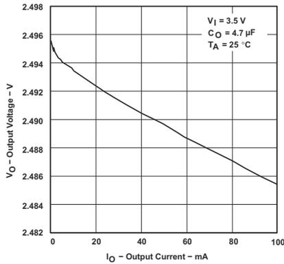
☒ 5-1. TPS76925-Q1 Output Voltage vs Output Current (Legacy Chip)
