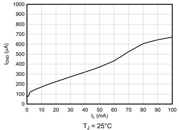
图 5-14. TPS76933-Q1 Ground Current vs Output Current (New Chip)
