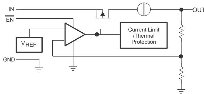
图 6-2. TPS769-Q1 Functional Block Diagram (Legacy Chip)
