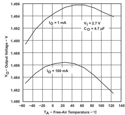
☒ 5-6. TPS76915-Q1 Output Voltage vs Free-Air Temperature (Legacy Chip)
