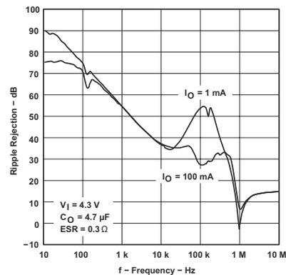
Figure 5-30. TPS76933-Q1 Ripple Rejection vs Frequency (Legacy Chip)
