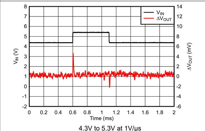
Figure 5-40. TPS76933-Q1 Line Transient Response (New Chip)
