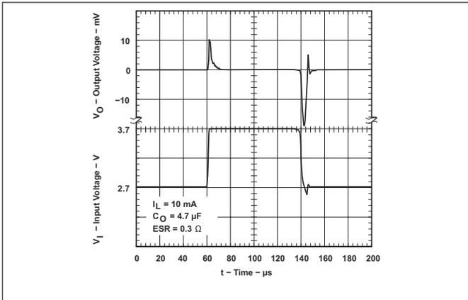
Figure 5-37. TPS76915-Q1 Line Transient Response (Legacy Chip)
