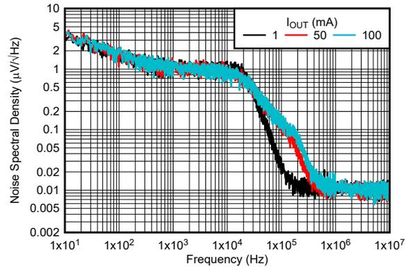
5-22. TPS76933-Q1 Output Spectral Noise Density vs Output Current (New Chip)
