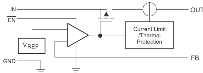
图 6-1. TPS76901-Q1 Functional Block Diagram (Legacy Chip)
