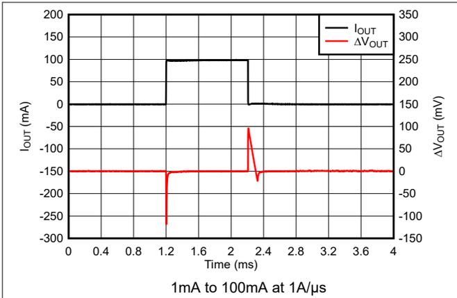
图 5-43. TPS76933-Q1 Load Transient Response (New Chip)
