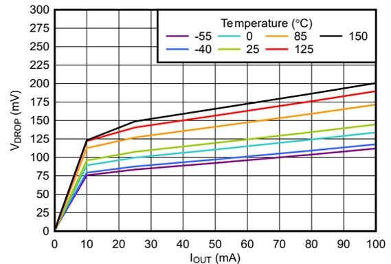
Figure 5-28. TPS76933-Q1 Dropout Voltage vs Output Current (New Chip)
