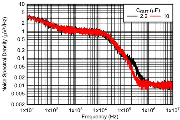
5-23. TPS76933-Q1 Output Spectral Noise Density vs Output Capacitor (New Chip)
