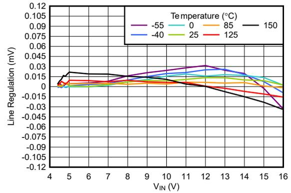
5-10. TPS76933-Q1 Line Regulation vs Free-Air Temperature (New Chip)
