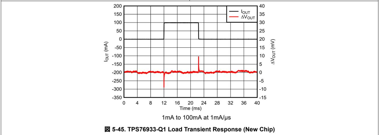
图 5-45. TPS76933-Q1 Load Transient Response (New Chip)
