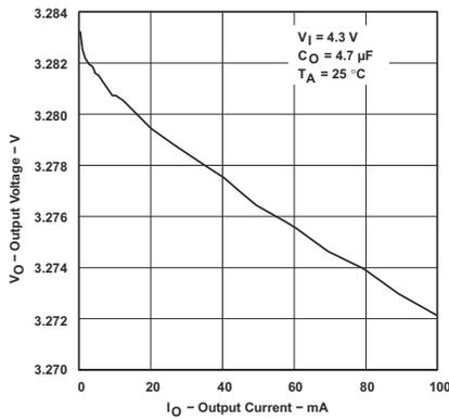
☒ 5-3. TPS76933-Q1 Output Voltage vs Output Current (Legacy Chip)
