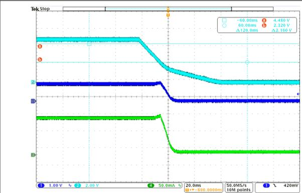
Channel 1 =  $V_{OUT}$ , channel 2 =  $V_{IN}$ , channel 4 =  $I_{OUT}$
