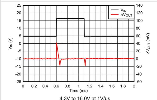
Figure 5-41. TPS76933-Q1 Line Transient Response (New Chip)
