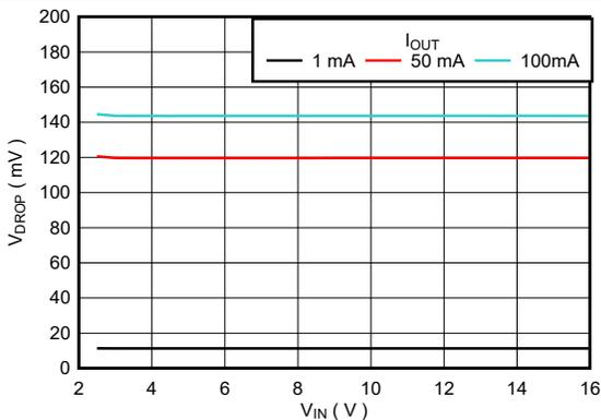
Figure 5-29. TPS76901-Q1 Dropout Voltage vs Input Supply (New Chip)
