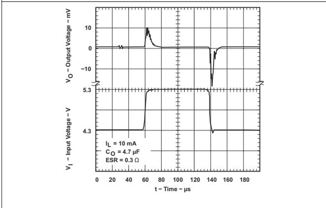
Figure 5-39. TPS76933-Q1 Line Transient Response (Legacy Chip)
