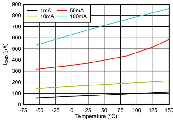
图 5-13. TPS76933-Q1 Ground Current vs Free-Air Temperature (New Chip)
