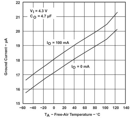
5-12. TPS76933-Q1 Ground Current vs Free-Air Temperature (Legacy Chip)
