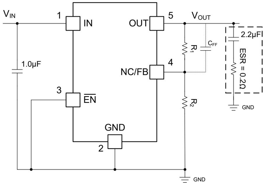
For adjustable output voltage options only. Dotted lines indicate an optional  $C_{FF}$  capacitor (new chip). See the [Feed-Forward Capacitor \( \$C\_{FF}\$ \)](#) section.
