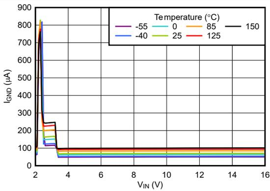
图 5-17. TPS76933-Q1 Ground Current vs Input Supply (New Chip)
