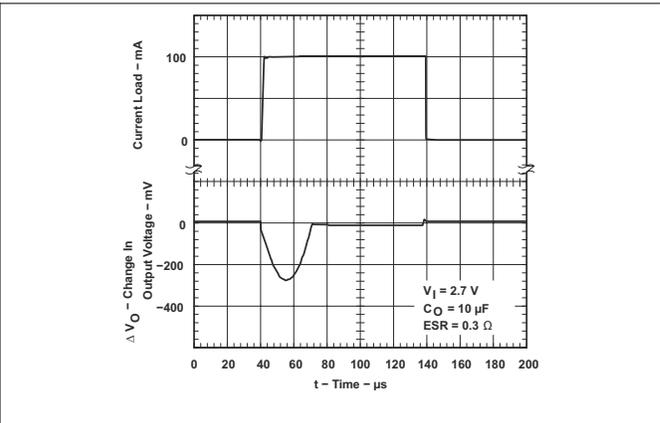
Figure 5-38. TPS76915-Q1 Load Transient Response (Legacy Chip)
