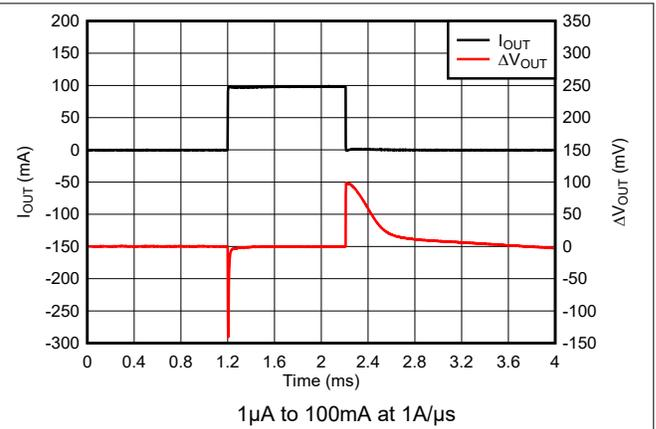
图 5-44. TPS76933 Load Transient Response (New Chip)
