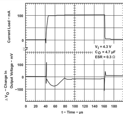
Figure 5-42. TPS76933 Load Transient Response (Legacy Chip)
