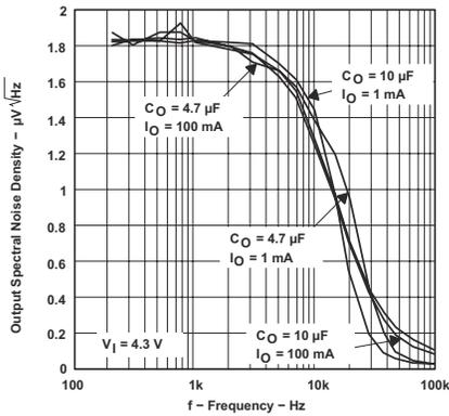
5-21. TPS76933 Output Spectral Noise Density vs Frequency (Legacy Chip)
