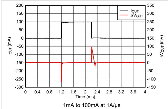
图 5-43. TPS76933 Load Transient Response (New Chip)
