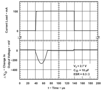
Figure 5-38. TPS76915 Load Transient Response (Legacy Chip)
