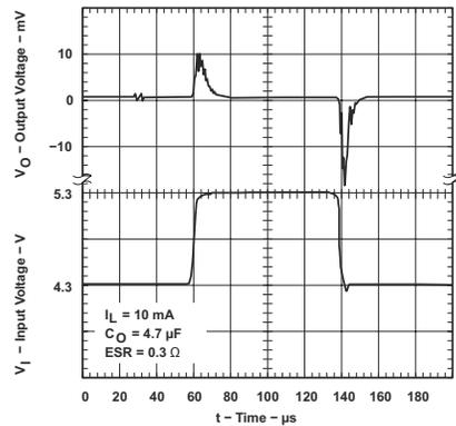
Figure 5-39. TPS76933 Line Transient Response (Legacy Chip)
