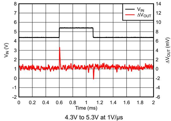
Figure 5-40. TPS76933 Line Transient Response (New Chip)
