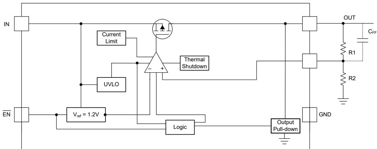
图 6-3. TPS76901 Adjustable Functional Block Diagram (New Chip)
