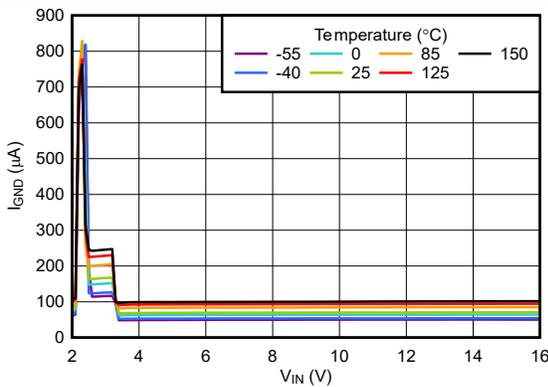
5-17. TPS76933 Ground Current vs Input Supply (New Chip)
