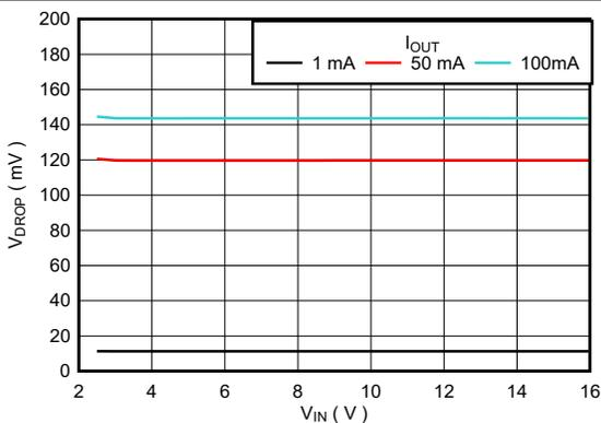
図 5-29. TPS76901 Dropout Voltage vs Input Supply (New Chip)
