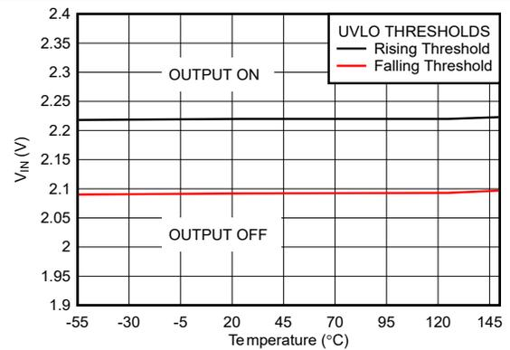
5-18. TPS76933 UVLO Threshold vs Free-Air Temperature (New Chip)
