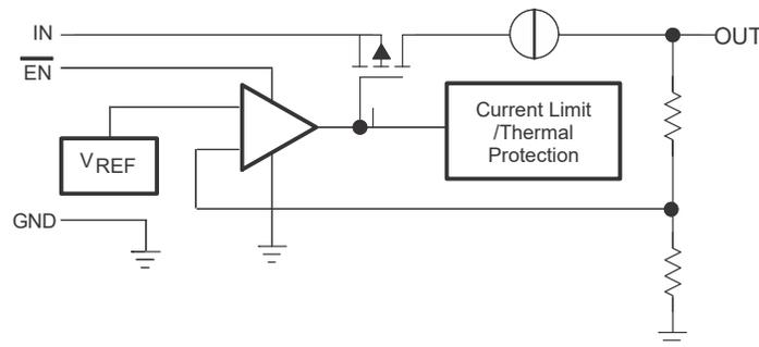
图 6-2. TPS769 Functional Block Diagram (Legacy Chip)
