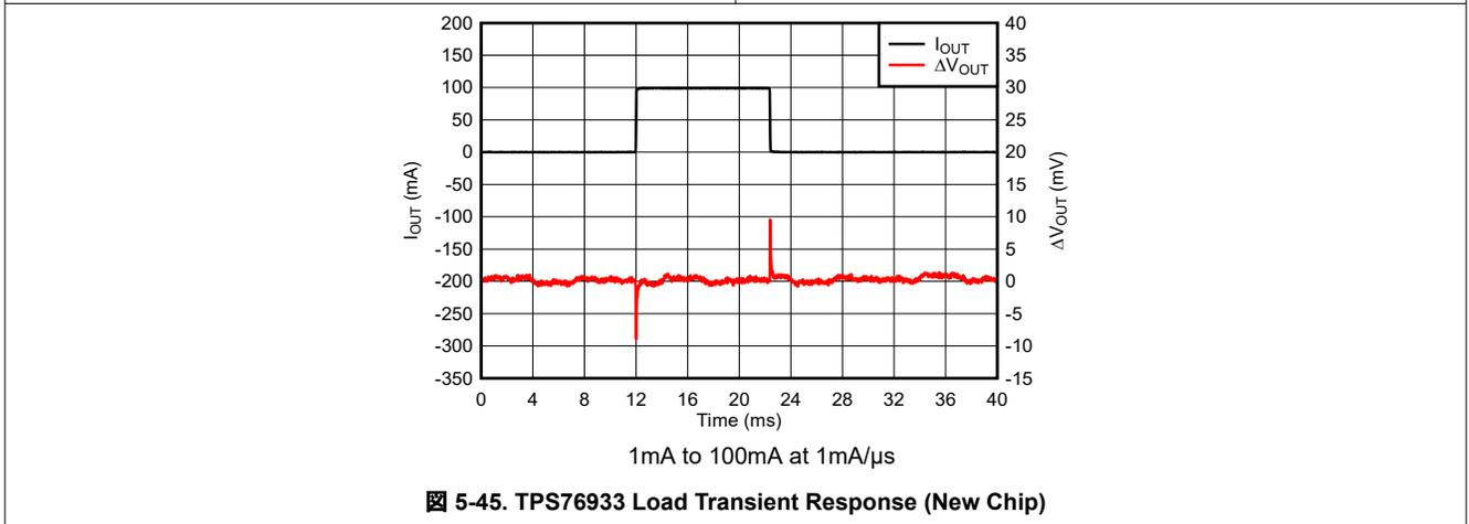
图 5-45. TPS76933 Load Transient Response (New Chip)
