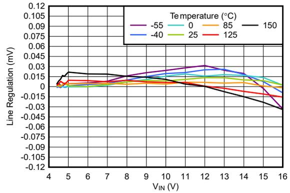
5-10. TPS76933 Line Regulation vs Free-Air Temperature (New Chip)
