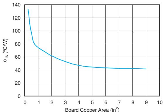
$R_{\theta JA}$  value at board size of 9  $\text{in}^2$  (that is, 3-in  $\times$  3-in) is a JEDEC standard.
