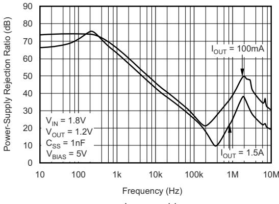
FIG 5-16.  $V_{IN}$  PSRR vs Frequency
