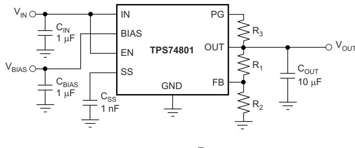
$$V_{\text{OUT}} = 0.8 \times \left( 1 + \frac{R_1}{R_2} \right)$$
