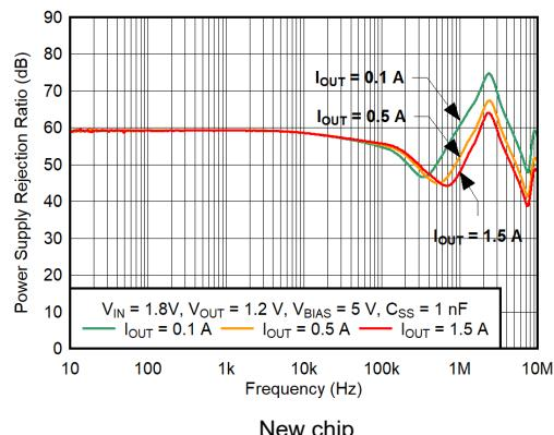
FIG 5-15.  $V_{BIAS}$  PSRR vs Frequency
