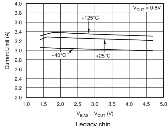
图 5-30. Current Limit vs  $(V_{BIAS} - V_{OUT})$
