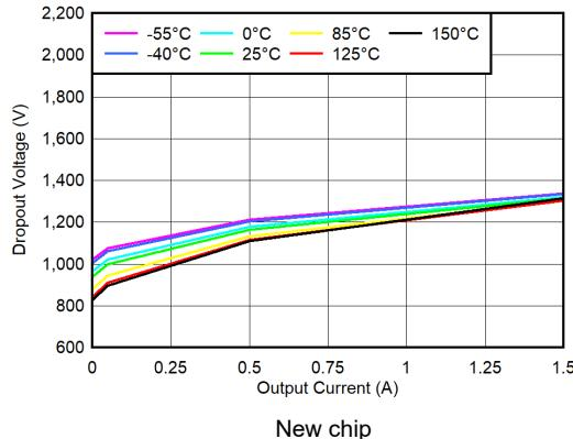
FIG 5-13.  $V_{BIAS}$  Dropout Voltage vs  $I_{OUT}$  and Temperature ( $T_J$ )
