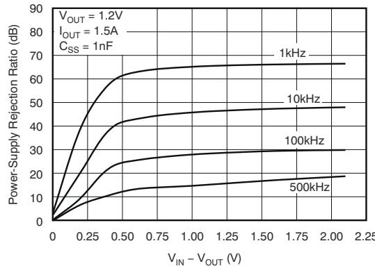
FIG 5-18.  $V_{IN}$  PSRR vs  $(V_{IN} - V_{OUT})$
