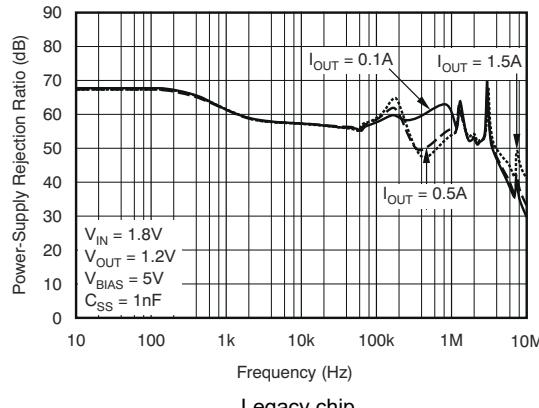
FIG 5-14.  $V_{BIAS}$  PSRR vs Frequency
