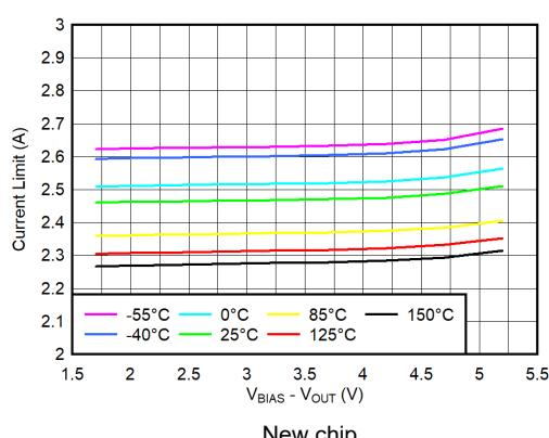
图 5-31. Current Limit vs  $(V_{BIAS} - V_{OUT})$
