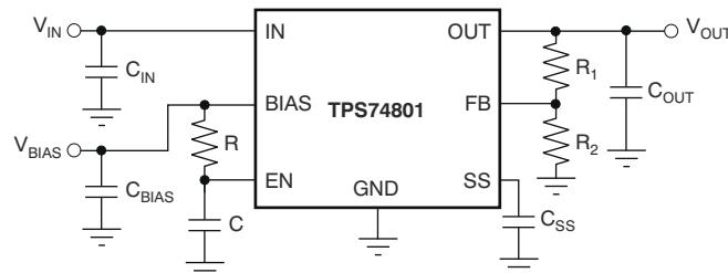
図 6-3. Soft-Start Delay Using an RC Circuit to Enable the Device
