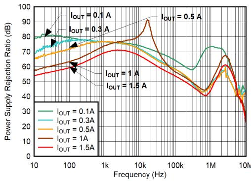
FIG 5-17.  $V_{IN}$  PSRR vs Frequency
