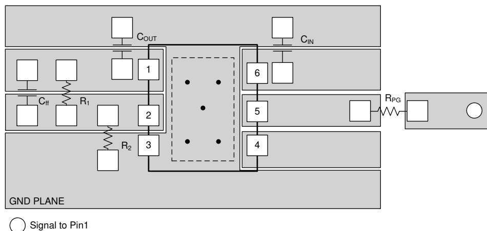
図 52. Layout Example for the DRV Package
