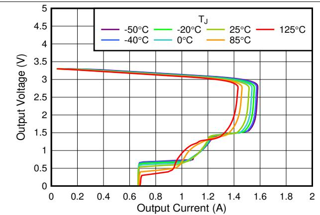
图 23. 3.3-V Foldback Current Limit vs I<sub>OUT</sub>
