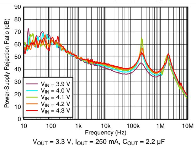
図 34. PSRR vs Frequency and  $V_{\text{IN}}$
