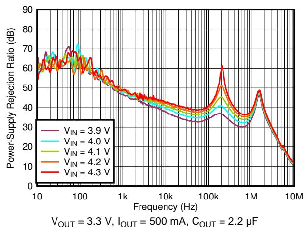
図 32. PSRR vs Frequency and  $V_{\text{IN}}$
