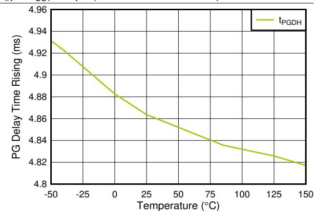
图 19. t<sub>PGDH</sub> vs Temperature (For TPS746B Only)
